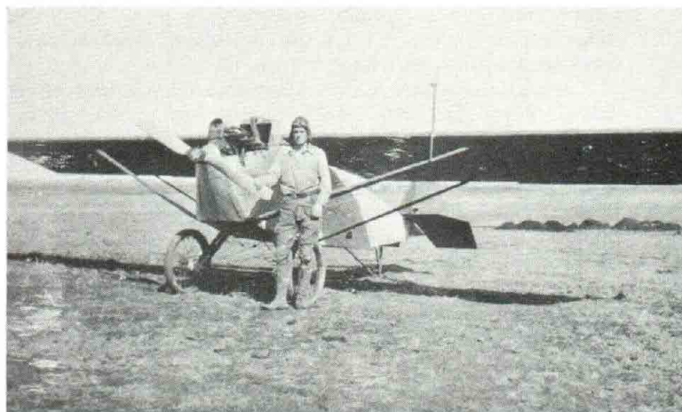
The second Ford A powered homebuilt appears to be an improved version of the earlier one, with the landing gear changed to a more conventional form.
