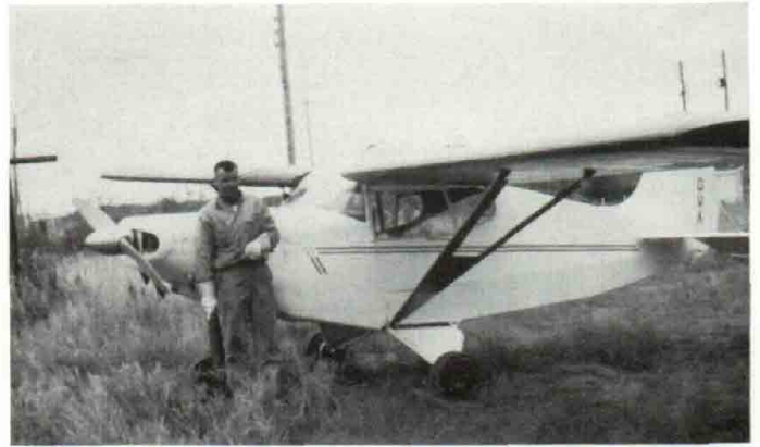
Cecil Goddard poses with his Stits "Skycoupe", CF-OWA, powered with a 125 hp Lycoming ground power unit. It is the latest in the long line of homebuilt aircraft which he has built.
