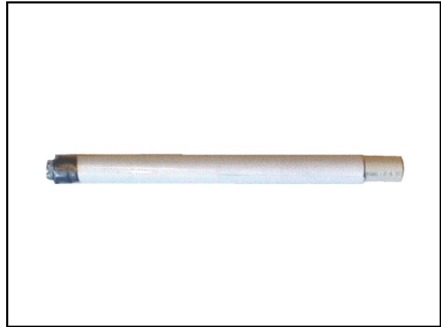
Figure 3: Cardstock Wrapped Around the Mold (½" PVC Pipe). In this Illustration, the Left End has been Crimped and Sealed and Ballast has been added. Note a Portion of the PVC Pipe Protruding from the Right End of the Rocket Tube.
