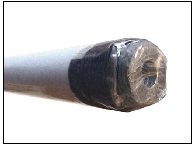
Figure 4: Ballast Secured to the Sealed End of the Rocket Tube
