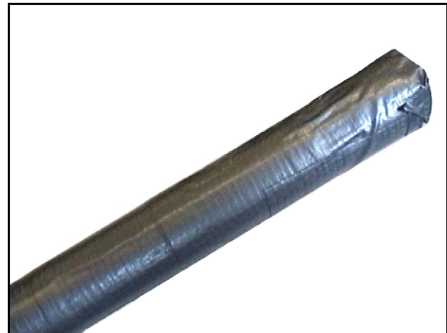
Figure 6: Duct Tape Applied to Exterior of Rocket Tube. This Measure is Only Needed for Medium- and High-Pressure Rockets.
