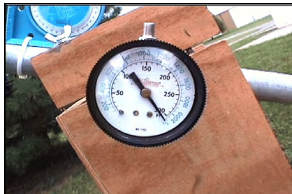
Figure 9: Launcher Pressurized to 300 PSI
