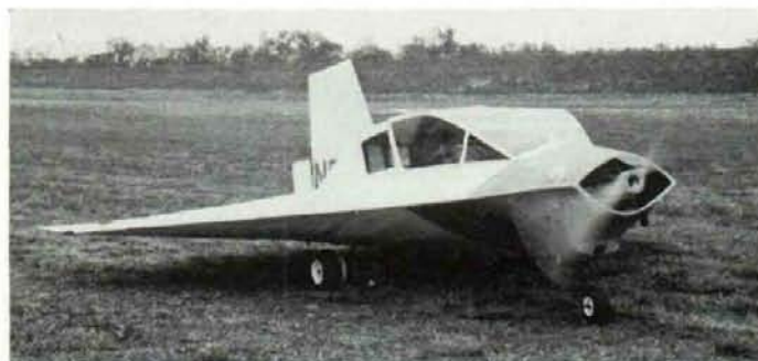
The cockpit canopy of the Dyke "Delta" forms an airfoil section matching the wing section. Certain areas of the plane, such as the engine cowling, were not painted at the time this photograph was taken.
