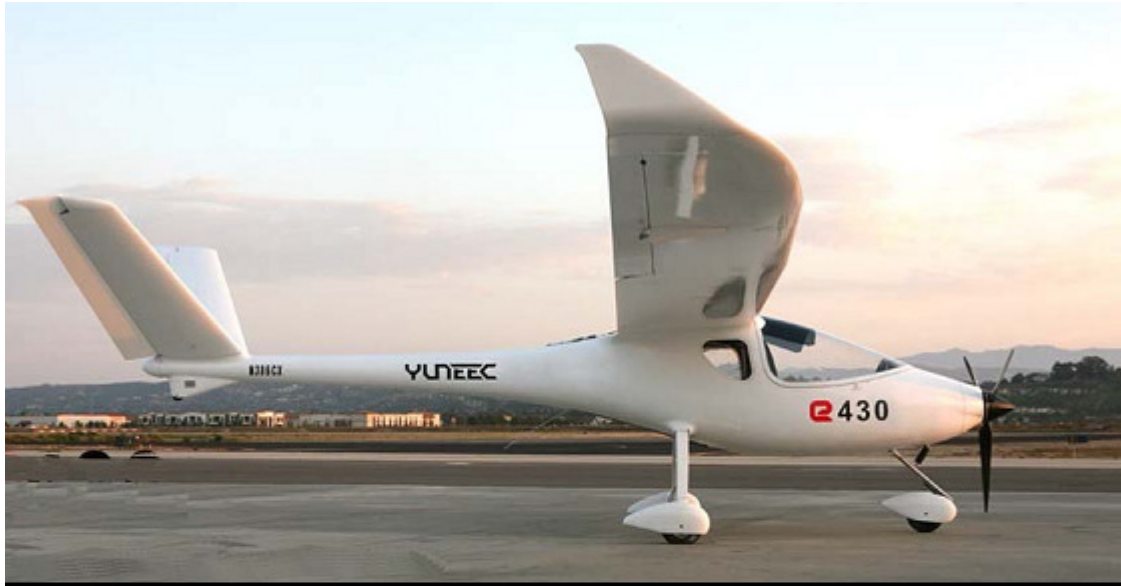
Variations on the theme. Both the Chinese Yuneec, above, and, Randall Fischman's Electraflyer 2, below, are basically motorgliders — currently the most appropriate use of electric power.
