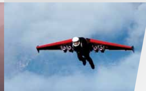
Yves' first four-engine wing had a rigid, carbon structure and folding wingtips. The four engines provided enough thrust for Yves to climb.
