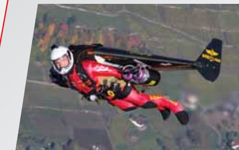
Reducing the size of the wing to 6 feet eliminated the need to fold the wings, saving 15 pounds. With the lighter, more agile wing, Yves performed his first aerobatics—two loops.
