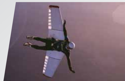
Using an inflatable wing, Yves improved his lift-to-drag ratio to 4-to-1. With this wing he glided the 12 kilometers across Lake Geneva.
