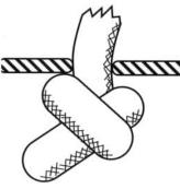
THIS IS A MODIFICATION OF JOE'S ORIGINAL DESIGN BY BION MCPEAK - ELIMINATE THE "U" BOLT, AND ON A NEW SET OF BASE PLATES, CAREFULLY RADIUS THE NEW HOLE FOR THE ROPE TO PREVENT CHAFING. THE HOLE SHOULD BE A TIGHT FIT FOR THE ROPE. KNOT THE ROPE AS SHOWN ON THE BACKSIDE OF THE BASEPLATE. MELT OR GLUE THE KNOT TO BE SURE IT WILL NOT COME UNDONE. THIS BASEPLATE IS NOT RECOMMENDED FOR USE WITH POLYETHYLENE ROPE.
