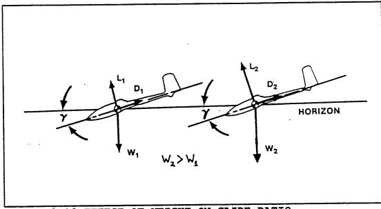
FIGURE 9.12 EFFECT OF WEIGHT ON GLIDE RATIO
