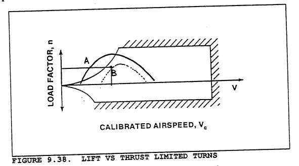
when it reached the stall. In other words, the thrust limits our sustained turn capability in situation B, and lift limits out sustained turn capability in case A. To determine the limiting factor of the aircraft, you must examine which parameter, at a given airspeed, is reached first (stall or  $P_a = 0$ ) at a set load factor. If, at 300 KIAS and 10,000 feet pressure altitude, you attempt to make a stabilized airspeed military power level turn and at 3 g you find you are
