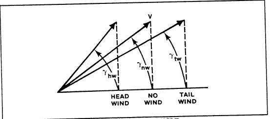
FIGURE 9.3 WIND EFFECT ON CLIMB ANGLE
