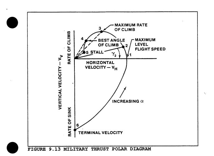
This plot represent all the combinations of vertical and horizontal velocities that the airplane can attain in unaccelerated flight at a given altitude, throttle setting, and weight.
