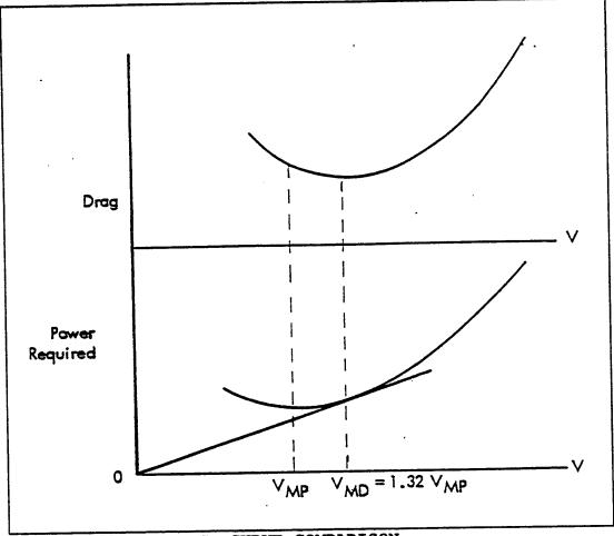
FIGURE 9.15 D AND P, CURVE COMPARISON
