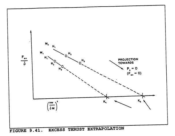
Lines of constant Mach should appear in Figure 9.41 as straight lines and can be extrapolated to zero thrust. The point at which zero excess thrust is reached is the point of maximum sustained load factor in a turn ( $P_s = 0$ ). Load factor can be calculated once the value of K is known.
