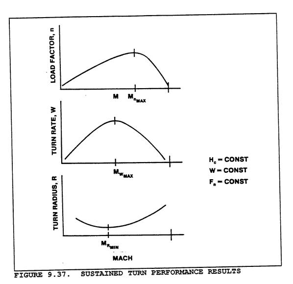
Thus, turn rate, turn radius, and radial acceleration are very important parameters, along with P<sub>s</sub>, in comparing relative performance of maneuvering aircraft. Such comparison, derived from the energy approximation, are of extreme interest to designers, operators, and test personnel.
