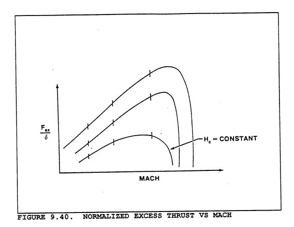
From figure 9.40 and Equation 9.30,  $F_{ex}/\delta$  can be plotted as a function of  $(nW/\delta M)^2$  at a given Mach and at n = 1 as shown in Figure 9.41.
