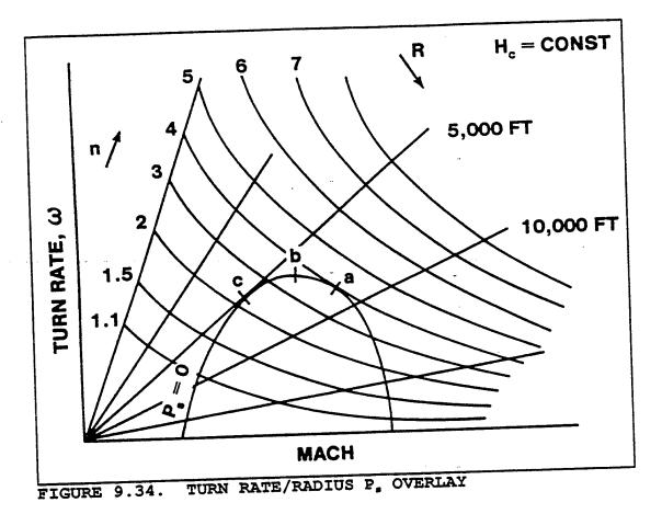
The point where the  $P_s = 0$  curve is tangent to a constant load factor line (Point a in Figure 9.34) yields the Mach for maximum sustained g for that configuration. The peak of the  $P_s = 0$  curve (Point b in Figure 9.34) yields the Mach for maximum turn rate, and the point where the  $P_s = 0$  curve is tangent to a value of constant turn radius (Point c in Figure 9.34)
