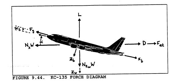
Summing forces perpendicular to the fight path  $(x_{w}$ -wind axis):
