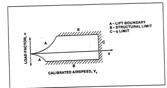
FIGURE 9.29 V-n DIAGRAM
