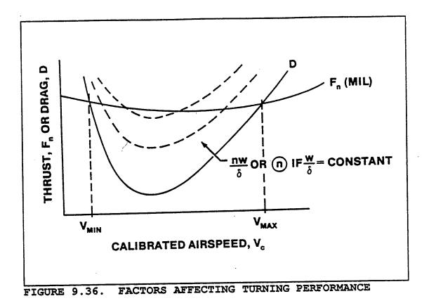
Figure 9.36 implies that a graph of load factor as a function of Mach for a sustained turn,  $P_n = 0$  ( $F_n = D$ ), would look like the upper plot of Figure 9.37. Once load factor is known,  $\omega$  and R can be calculated. Typical results are also presented at Figure 9.37.
