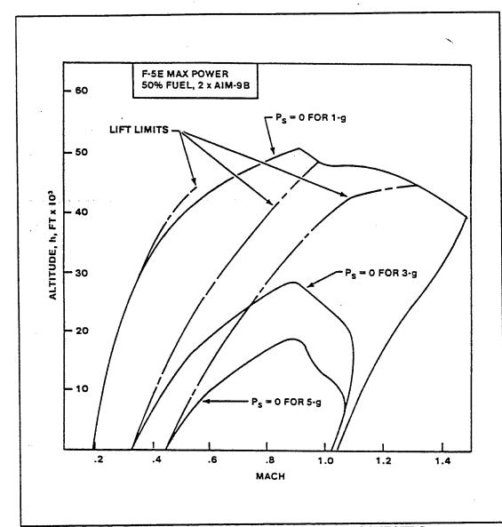
FIGURE 9.22 EFFECT OF LOAD FACTOR ON P. CONTOURS
