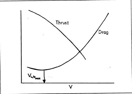
FIGURE 9.6 PISTON AIRCRAFT THRUST/DRAG CURVES
