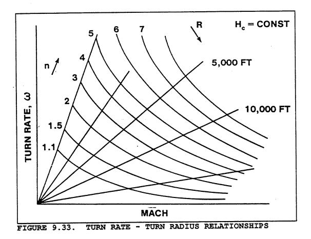
Overlaying a  $P_a = 0$  curve for a particular aircraft onto Figure 9.33 makes the chart aircraft specific and will yield three Mach numbers of interest as illustrated in Figure 9.34.
