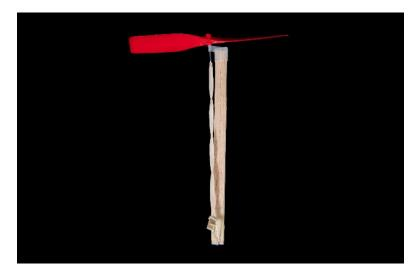
In a helicopter, the tail rotor would be used to counteract torque. Because the helicopter you are building is so light, you will be using air resistance to counteract the effects of torque. If the force of torque is left unbalanced, the rotor and the craft stick will both turn, in opposite directions (Newton's third law), and use up much of its energy. If we can counteract the torque effect, your helicopter will fly much higher!
