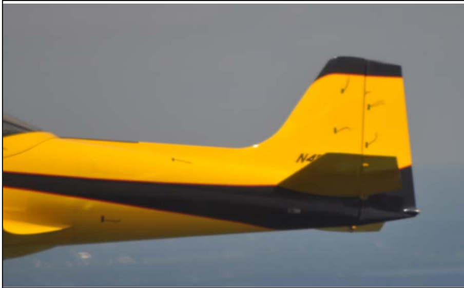
Figure13. Separation on concave Side of Vertical Tail
