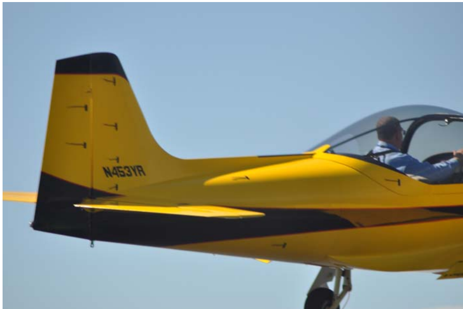
Figure 12. No tendency for separation on the convex side of the vertical tail
