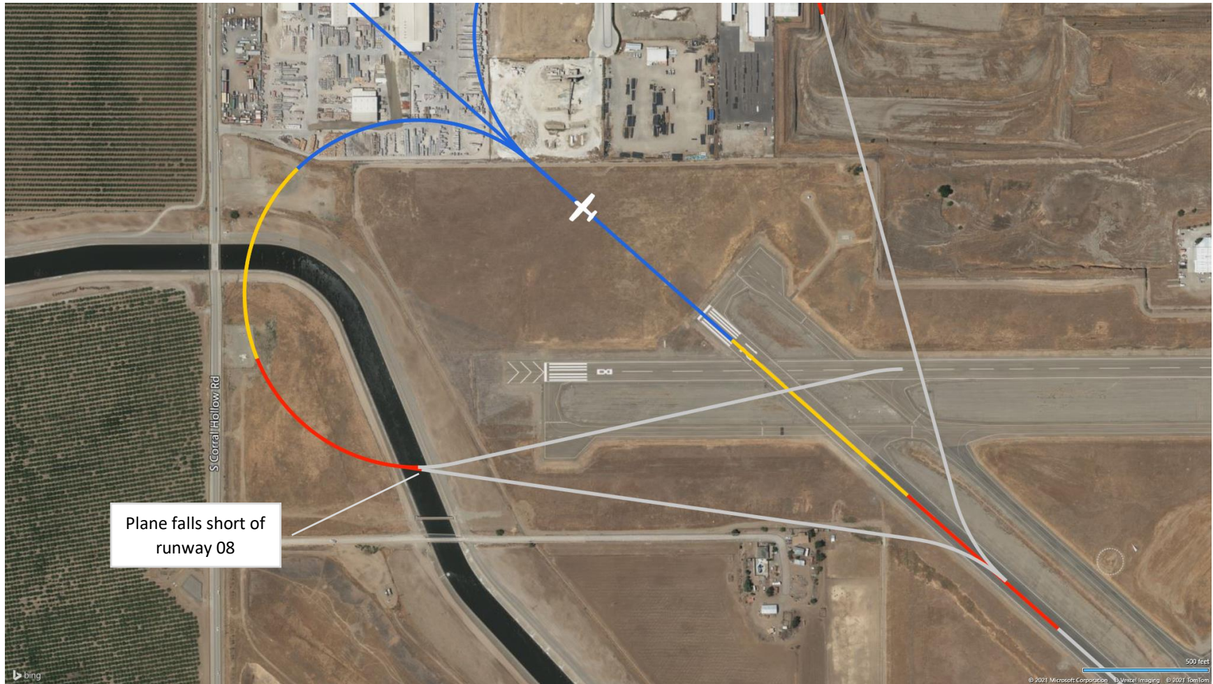
Figure 8. Loss of power occurs at 300 ft.
