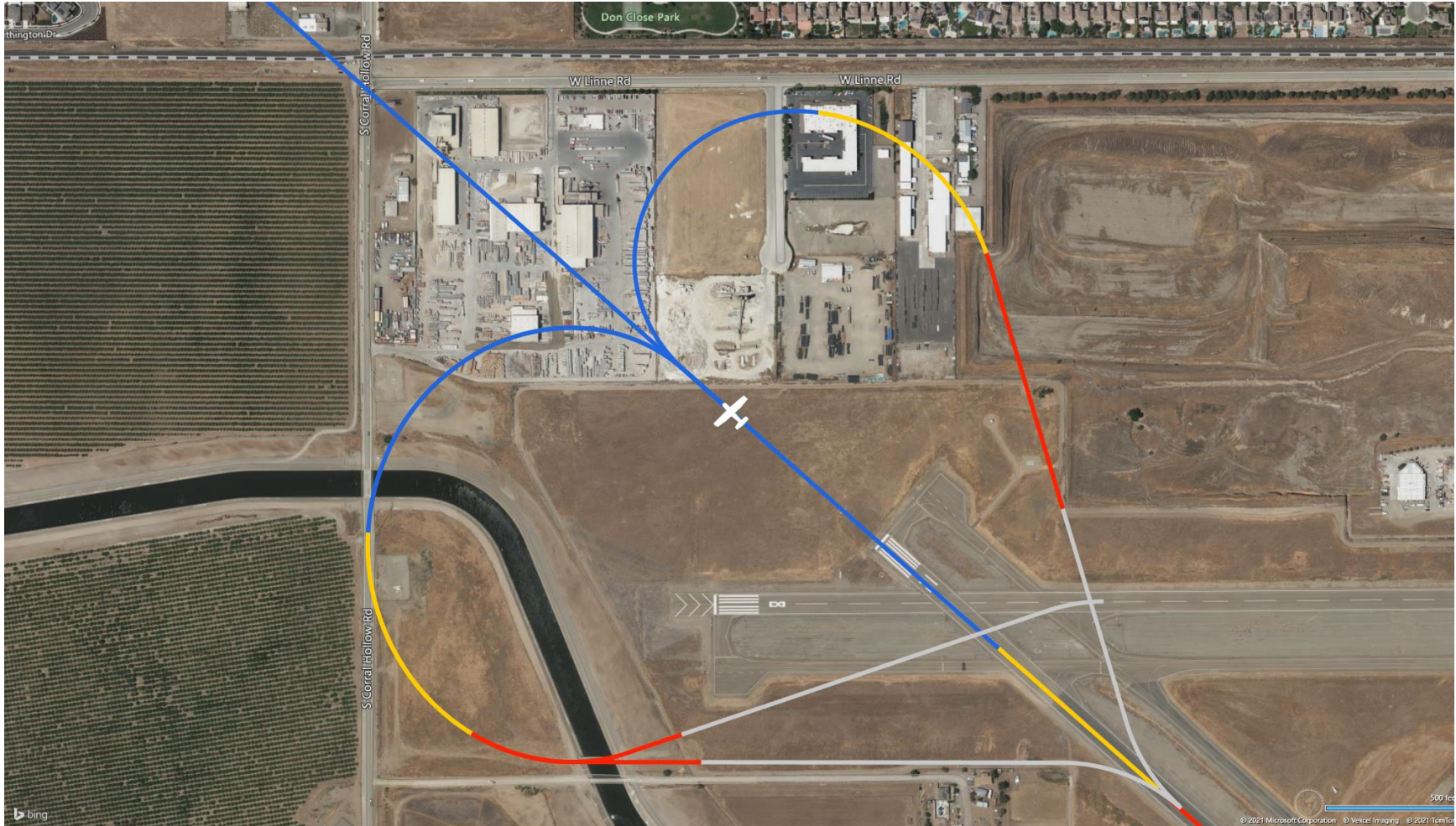
Figure 19. 10-knot wind from 0 degrees. Plane crabs into the wind to maintain track. Loss of power occurs at 371 feet AGL.
