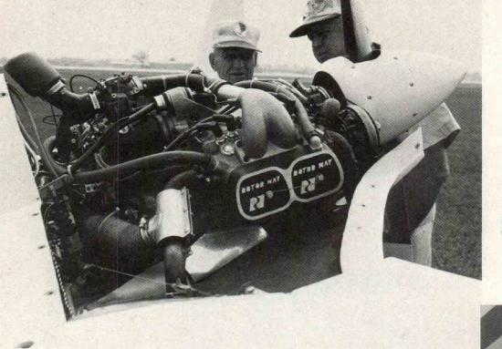
(Photo by Jack Cox) Latest version of RotorWay's water cooled flat four installed in a VariEze.
