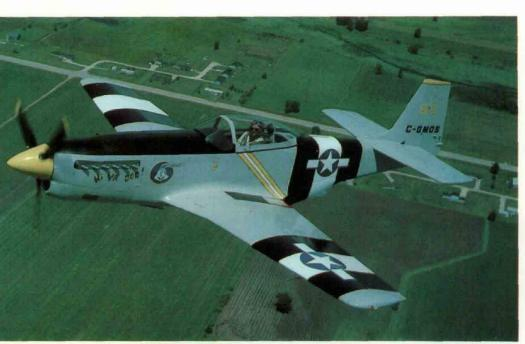
(Photo by Ted Koston) Ross Grady (EAA 124821), 9547 81st St., Edmonton, Alberta in his modified SAL 2/3 scale Mustang. Powered by a 200 hp Ranger. Quite realistic, eh.
