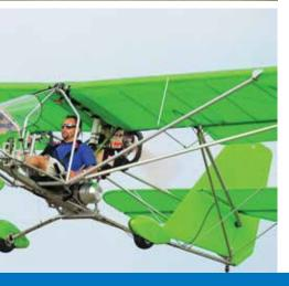
than 254 pounds, or has a stall speed that exceeds 24 knots or a top speed greater than 55 knots, then this plane cannot be operated under the ultralight Part 103 rules. If it is not N-numbered and airworthiness certificated, it is considered an illegal aircraft and you could be fined by the FAA for flying it.
