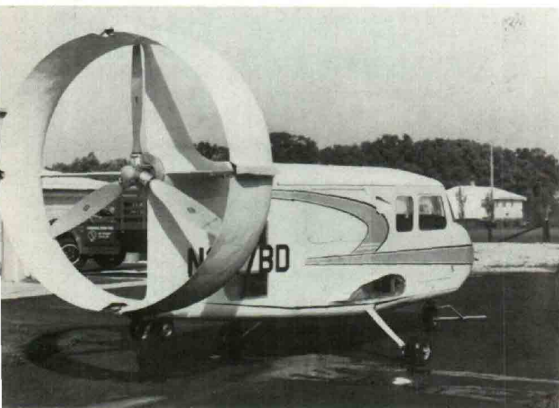
The Bede XB1D, a pusher boundary layer control aircraft, has been donated to the EAA Air Education Museum by Jim Bede of Cleveland, Ohio. This advanced design started in 1960 and was powered by two Franklin 165 hp engines mounted one above the other in the honeycomb sandwich constructed fuselage. The metal wings have thousands of tiny holes in their surface and many flights were conducted as a research aircraft. It was brought to the EAA Museum on a truck by EAA Director Val Brugger and EAA member Les Kellogg. It is now on display in the Air Museum.
