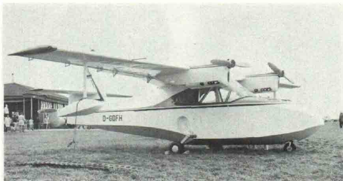
This handsome German-registered amphibian was built by Carl Johannsen of Denmark. Power is two 65 hp Walter "Mikron III" engines, the wing is full cantilever, and the airplane is generally quite clean. The main gear legs swing upward and slide inward for flush retraction. The builder poses with his amphibian which is much smaller than one would expect.
