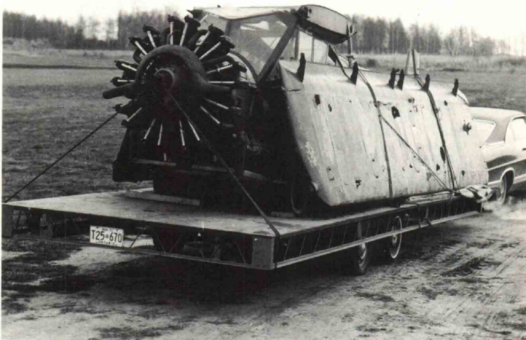
The Salmson with its front exhaust collector presents a formidable appearance. The windshield and cabin windows consist of flat panels, and there are few items on the entire airplane that would present any problems should refabrication be necessary.
