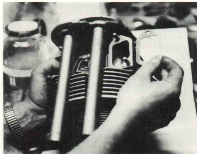
FIG. 3: The template is matched to the cylinder being used as the master.
