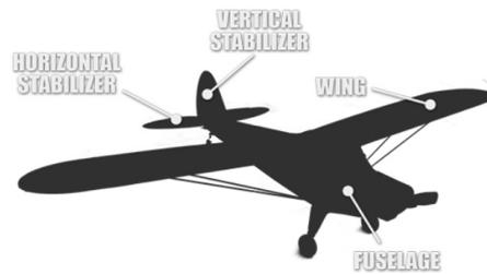
With the students helping identify the different components, now get into the forces that act on the aircraft during flight. See diagram below as a resource;
