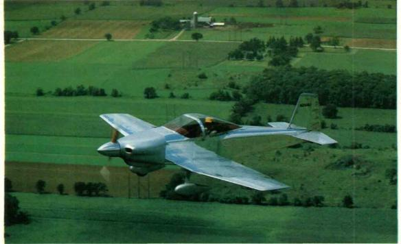
(Photo by Ted Koston) Mike Rudolph (EAA 121003) of Rt. 2, Box 48, Sand Springs, OK 74063 in his highly polished Mustang II. Powered by a Lycoming 0-320-B2B (160 hp). Empty weight is 924 pounds and gross is 1500. Cruise with a Pacesetter 200 prop is 185 mph.
