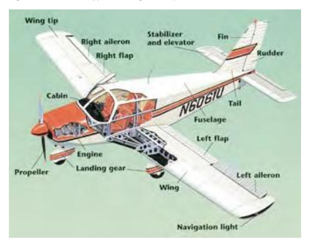
Image above: This drawing shows the parts of a light airplane called a Piper Cherokee.
