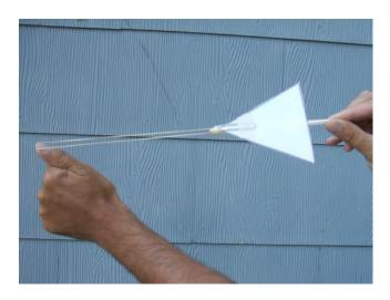
7. Students should vary the thrust of their planes by varying the initial stretch of the rubber bands. Using a ruler or meter stick would allow students to double the stretch and see how the distance of flight changes, all else constant
