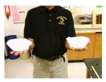
Simulating more weight, constant surface area 1 filter vs. 2 filters (nested) vs. 3 filters (nested) vs. 4 filters (nested)
