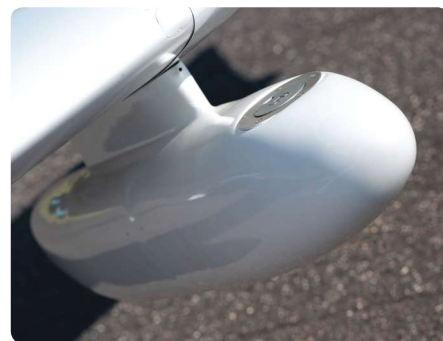
The tanks hold six gallons of fuel each and Lee says he only sees about a two to three mph loss in speed.
