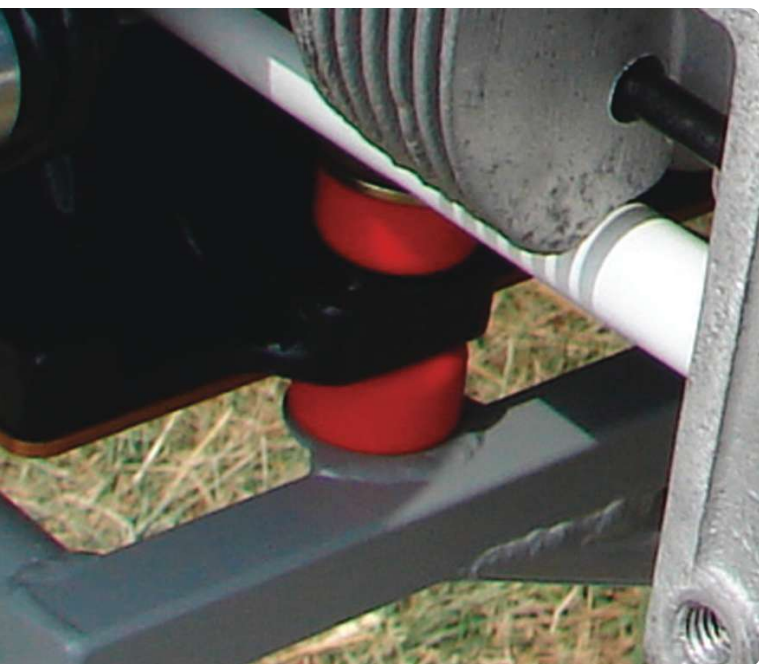
“Doughnuts” may also be used vertically in compression. This example is on the Corvair-powered Panther prototype on display at EAA AirVenture Oshkosh 2012.
