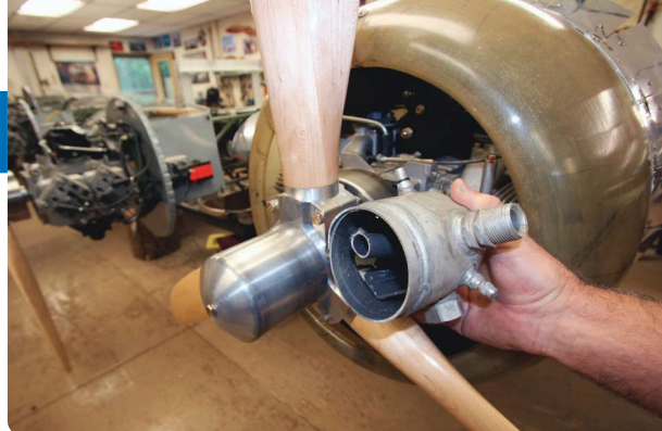
The spinner for the propellers is made from a home air conditioner part, sliced in half, and machined to fit and look to scale.
