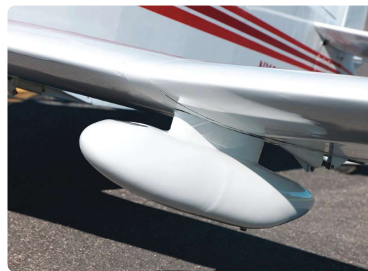
Lee added F-86-style drop tanks to increase the range of this aircraft.
