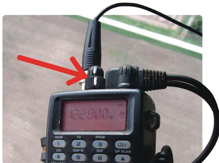
White index marks on radio controls let me confirm at a glance that my radio volume and squelch are set properly so I won't miss any radio calls.
