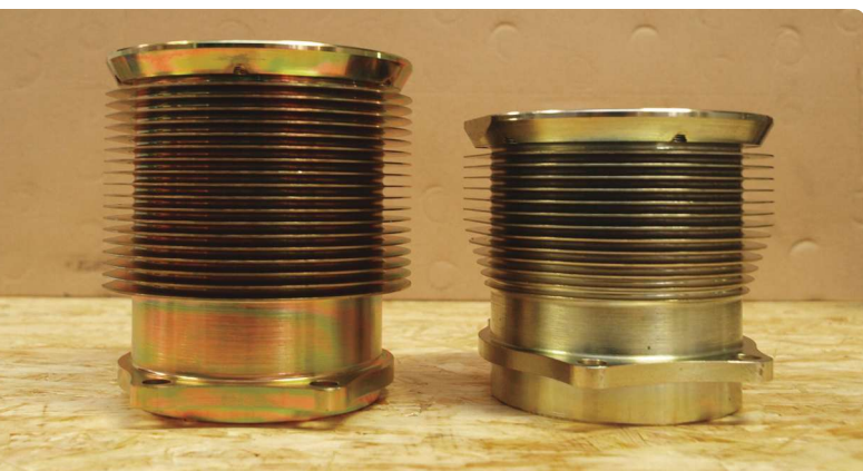
All ULPower engines exist in two different displacements and compression versions. The higher displacement versions use the taller cylinder (at left) while the lower displacement versions use the cylinder shown at right. All ULPower cylinders have a 105.6 mm cylinder bore; with two different crankshafts and shorter and longer cylinders, the stroke is 74 mm or 100 mm respectively, resulting in two different displacements. That is the difference between the ULPower 260 and 350 engines with 2.6 and 3.5 liter of volumetric displacement. But additionally on each engine with the same displacement, with two different cylinder heads and two different compression ratios you get two different power outputs. That's the ULPower equation for a wide power output choice.
