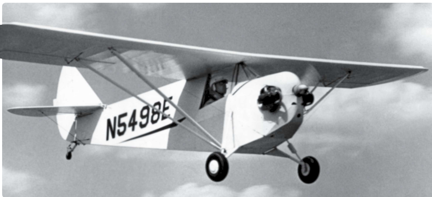
Dick Giede, a retired Cessna engineer from Wichita, built this to-the-plans Headwind in the early 1960s. Equipped with a direct-drive VW, at last report he had logged more than 1,000 hours on the airplane.
