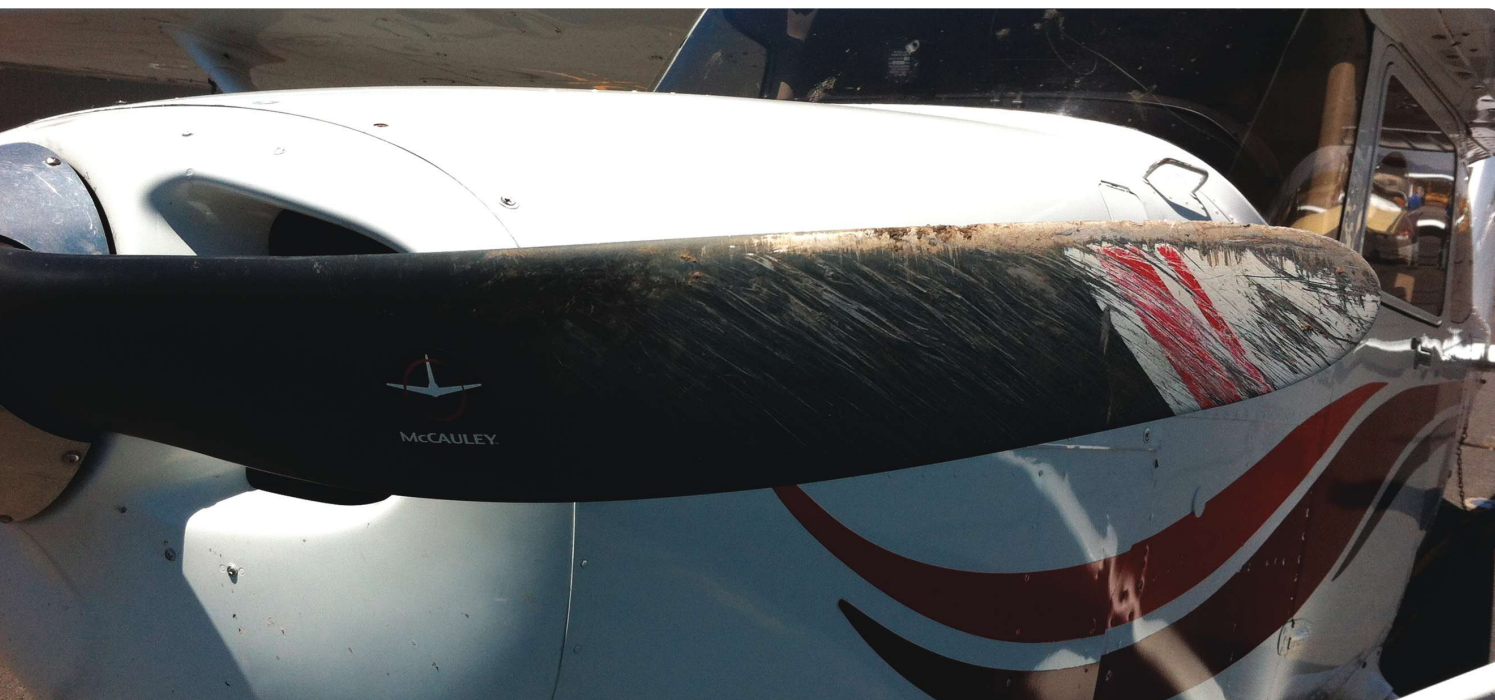
An off-ramp excursion, even into soft earth, will often lead to a written-off prop. This one might be salvageable, but only the manufacturer will be able to tell.
