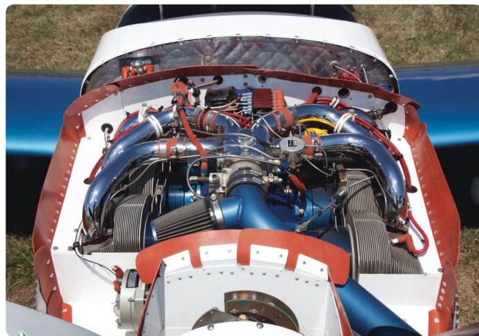
When Andy's 310-hp Continental IO-550N wasn't coming together quickly enough, Andy assisted the engine builder to finish the project.
