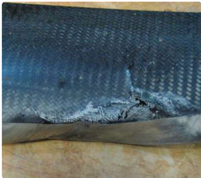
Even a tough all-composite prop will be ruined when it hits something solid.
