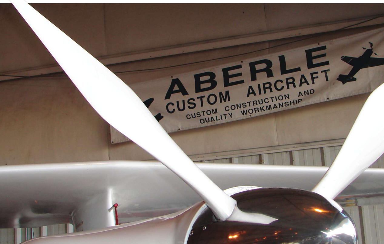
Tom Aberle's Phantom biplane runs this radical Paul Lipps-designed prop at Reno. Takeoff is long, but its top speed is dominant in the class.
