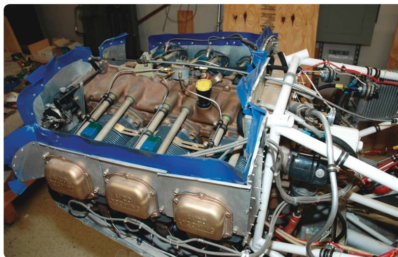
Jeff added fuel injection to the Lycoming 540 powering the Barracuda. It puts out 300 hp.
