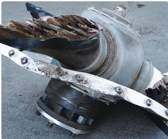
This wood-core composite prop failed when it was over-revved at more than 400 mph. No propeller would survive this.
