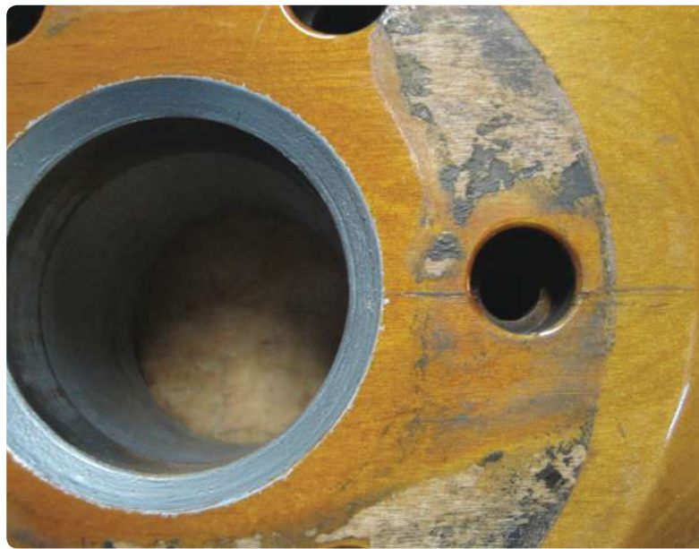
When a prop is even slightly loose, it can "burn" as it rubs against the hub causing the prop to become less efficient.
