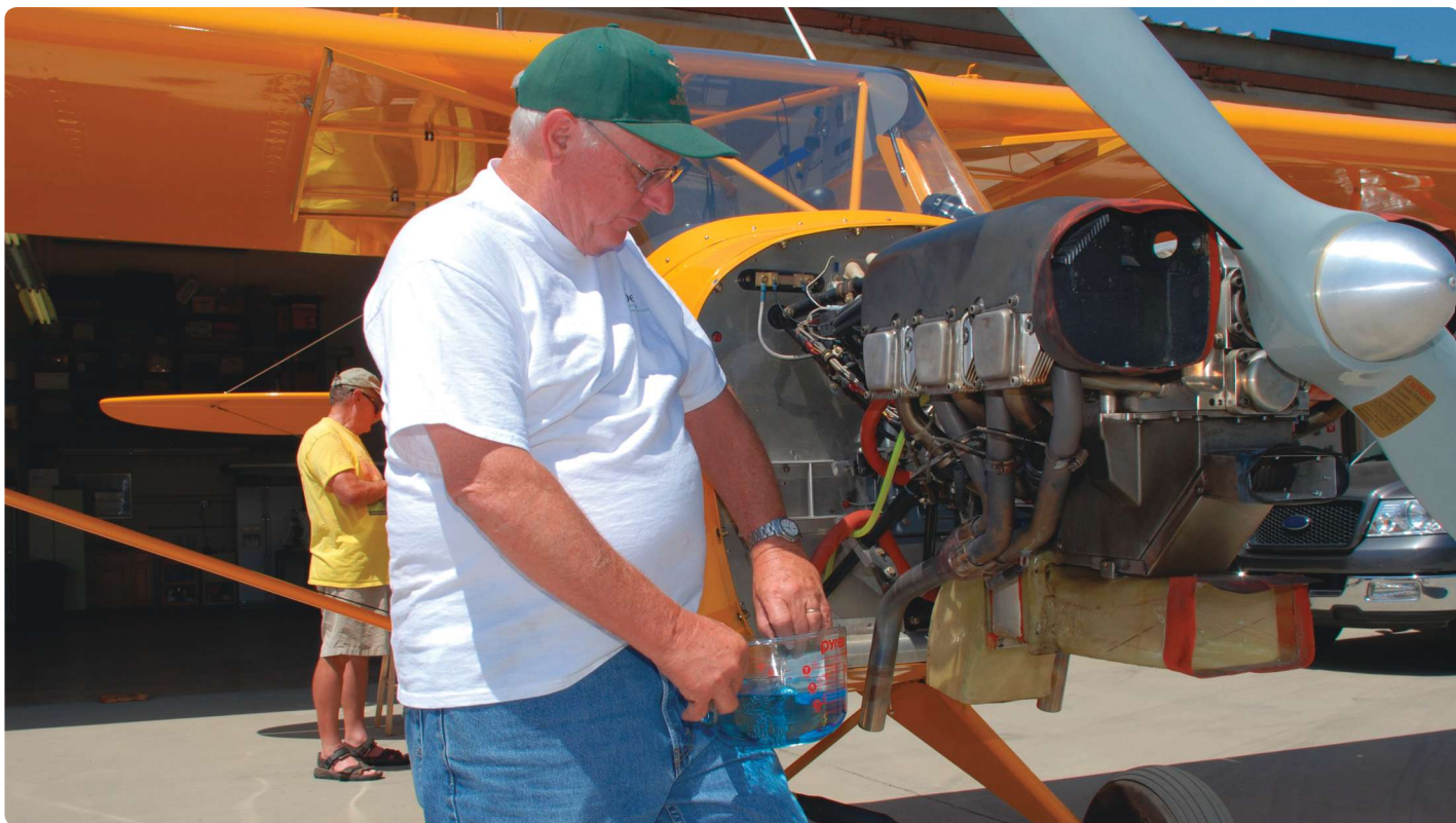
EAA member Ed Zaleski measures the fuel flow in the level-flight position of a Jabiru-powered Texas Sport Cub. A 2-quart measuring cup works well for this.
