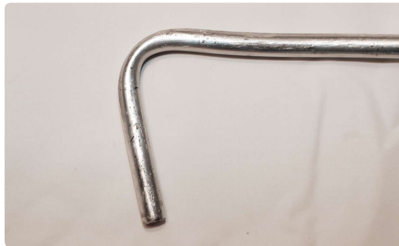
A kinked or partially collapsed fuel line, such as the one shown here, will drastically reduce fuel flow.
