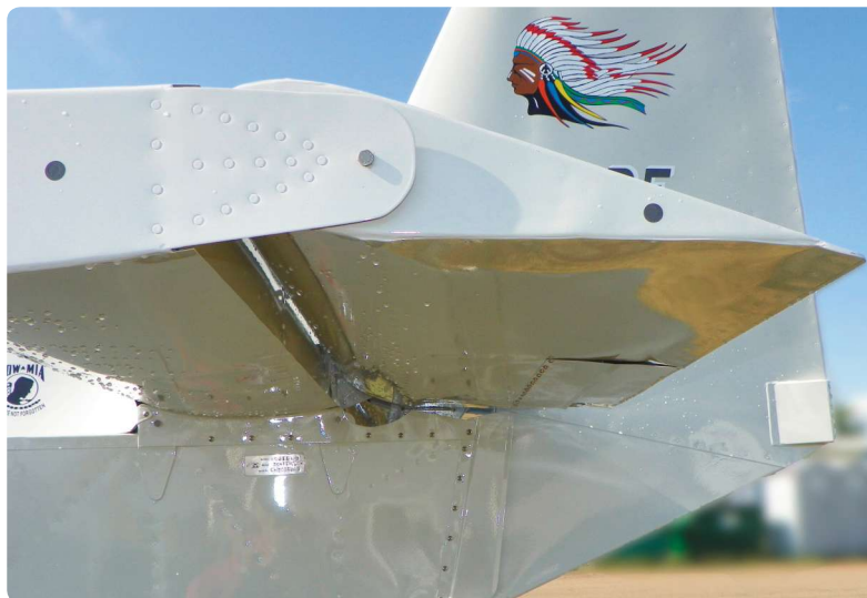
Details of the empennage, including gap seals and trim tab.
