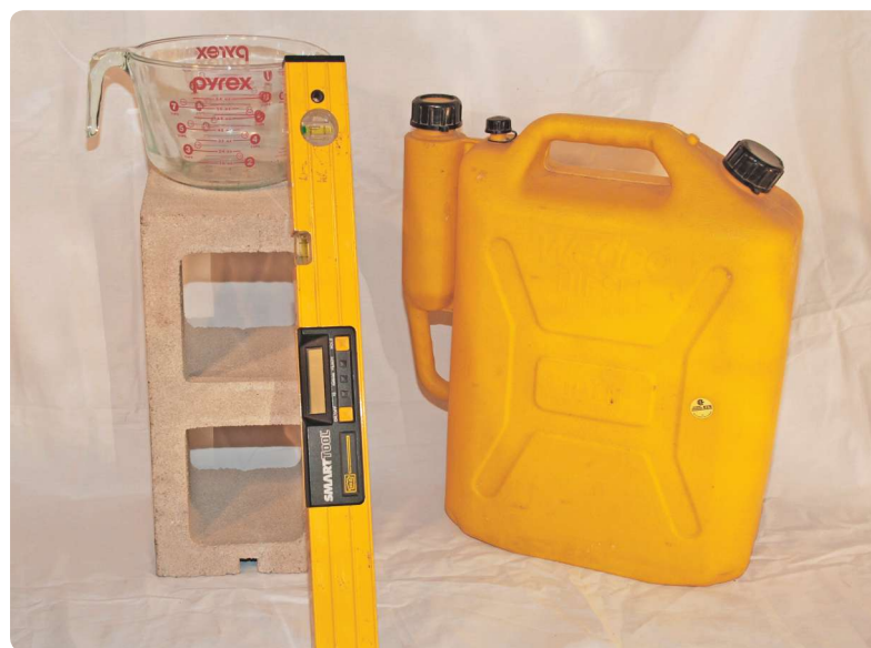
To do the fuel flow tests you will need a gas can, a 2-quart measuring cup, a Smart level, and some cinder blocks or other blocking material.
