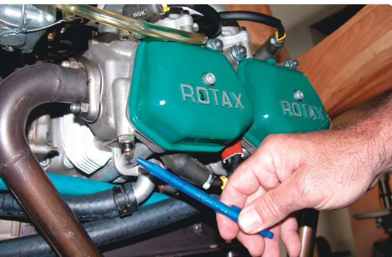
A common failure happens when this temperature sensor melts or gets crushed. It's easy to check.
