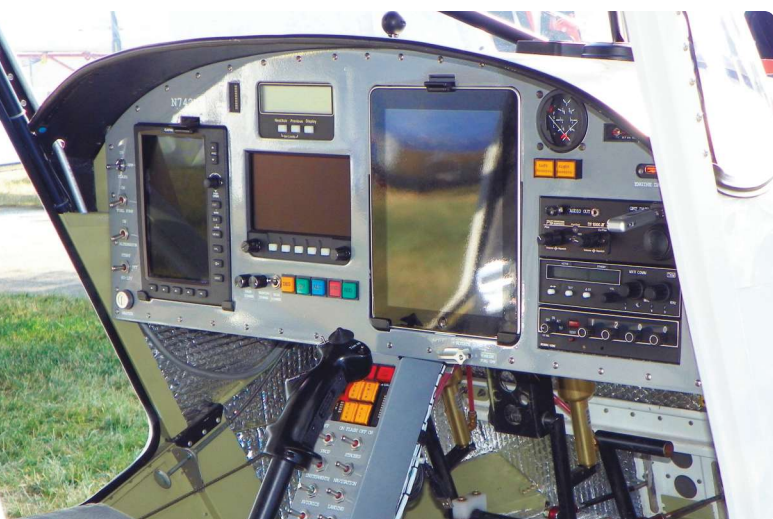
A simple but very useful instrument panel, including an Apple iPad. Sharp eyes might pick up the USB pen drive used for downloading flight data.
