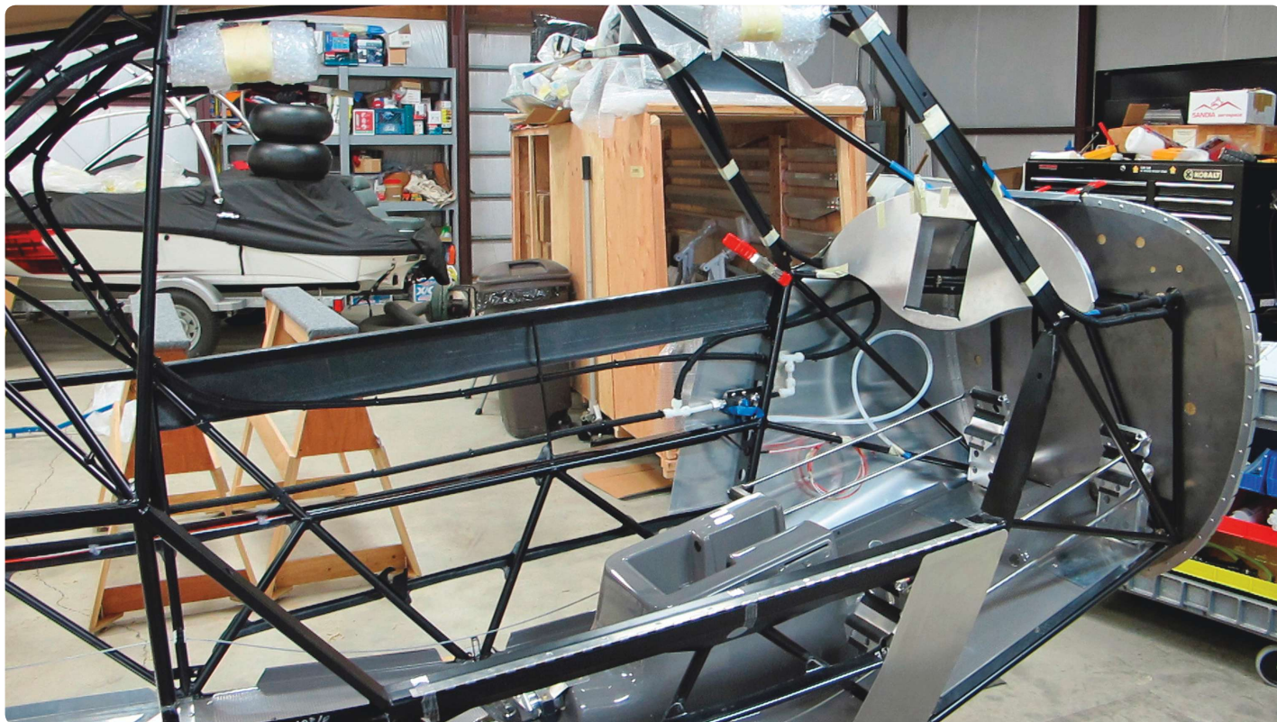
Tony's Cub comes together, showing the structure of the front cockpit.
