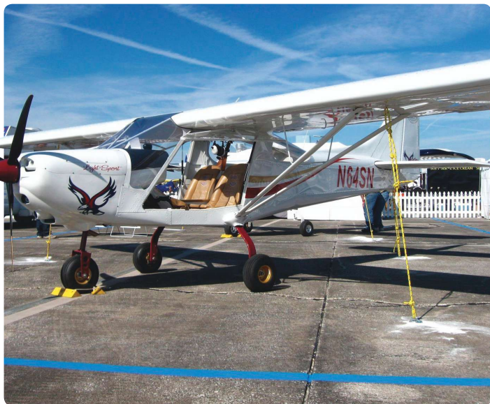
The rugged, all-metal Vision LT features a 48-inch-wide cockpit.
