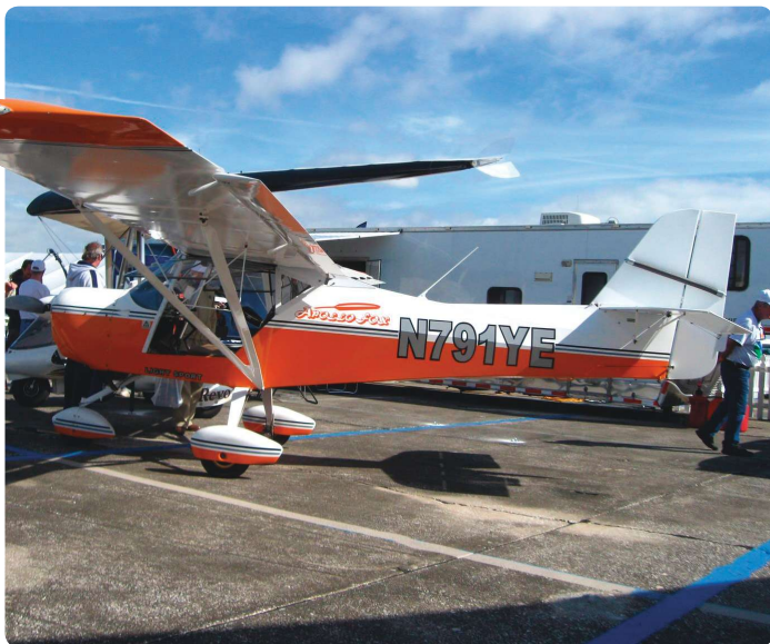
The steel tube and fabric Apollo LSA was inspired by the Avid and Kitfox designs.
