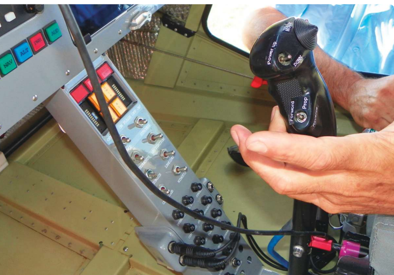
A simple but very useful instrument panel, including an Apple iPad. Sharp eyes might pick up the USB pen drive used for downloading flight data.
