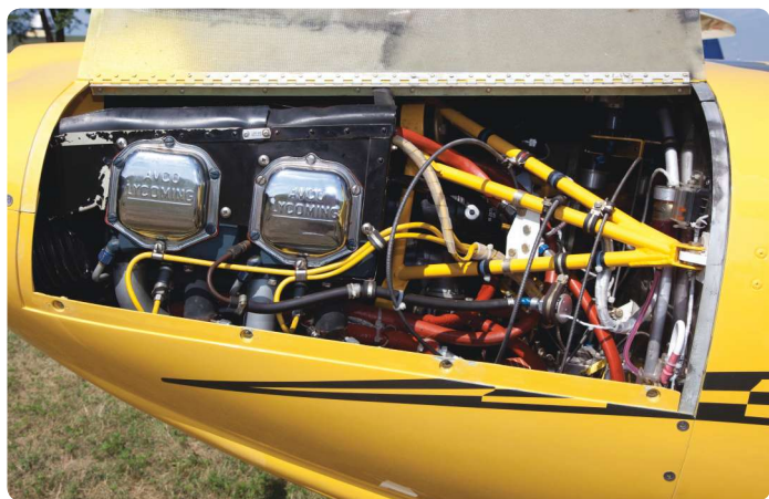
Power for George's Falco is an overhauled 160-hp Lycoming IO-320 paired with a Hartzell prop. Both were "fugitives" from a Twin Comanche.
