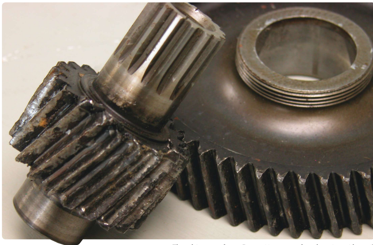
These drive gears, from a Rotax 582, were run for a short time without oil.
