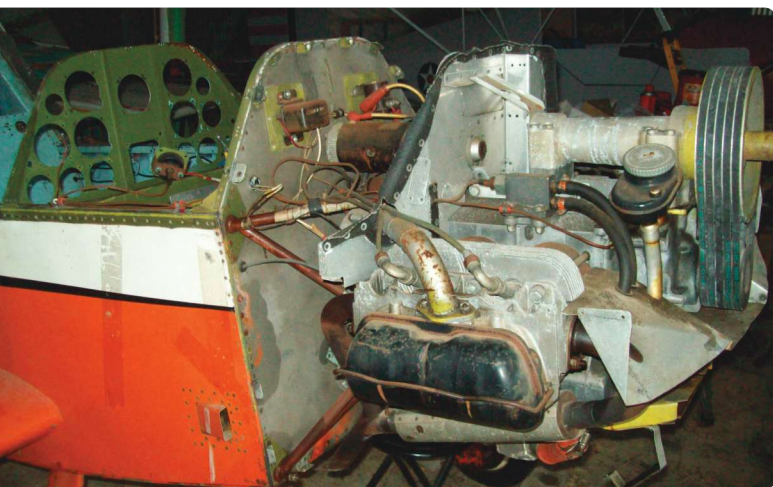
The original 40-hp VW conversion engine with a multi-sheave V-belt redrive wasn't salvageable. Pilots who flew the PL-4A with this engine felt it was underpowered.
