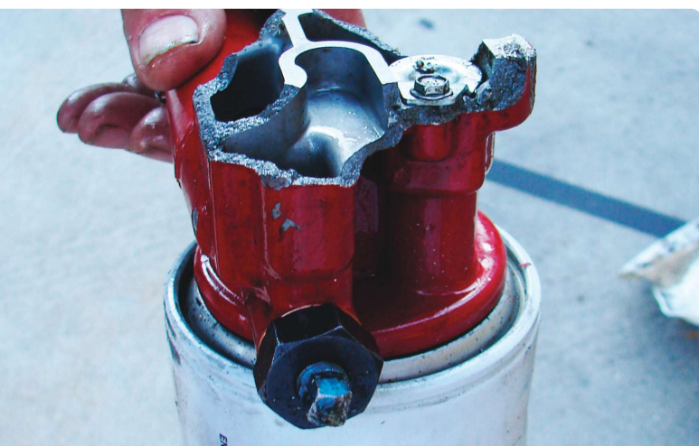
If any component in the oil system fails, you won't get oil. This is a rather catastrophic failure, the kind of thing that happens at Reno. It shouldn't happen on your engine.
