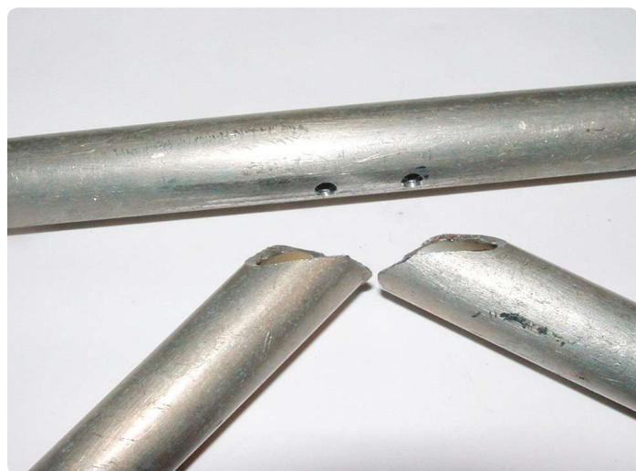
These photos show vent holes drilled in longerons and diagonals as they would form a cluster over the vent holes. Holes allow both venting and oil flow.
