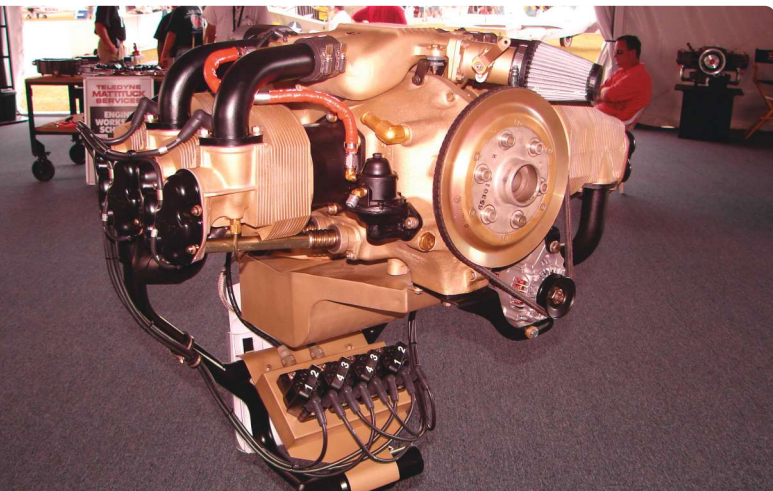
The large sump on this conceptual Continental O-200 collects, de-aerates, and even cools the oil. (Note that there are no cooling fins on the cylinders.)
