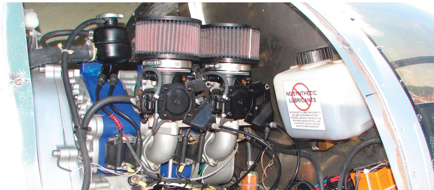
Use the lubricants that are recommended by the manufacturer. This Sadler Vampire's Rotamax is placarded against synthetic lubricants.
