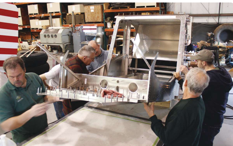
EAA staffers work on setting the center section in place with the help of Zenith expert Tracy Buttles.
