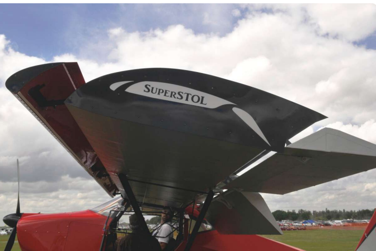
Slotted ailerons and Fowler flaps contribute to slower speeds with full control.
