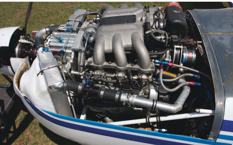
The Subaru 3.3 liter SVX puts out 240 hp at 6000 rpm and is lighter than most V-8s. The induction system, however, forced Holmlund to build a fairing over it.
