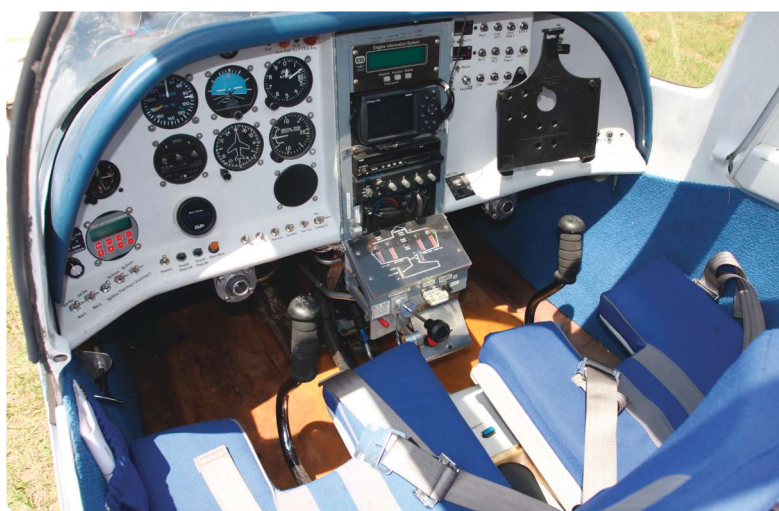
The fuselage is much wider than most aircraft. The builder's group had to build its own top fuselage half, adding right and left doors.
