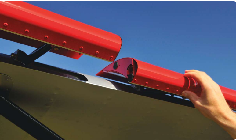
With one fully deployed (on left) and one shown halfway, these automatic slats on each wing help the SuperSTOL fly slowly and land shorter than normally possible.
