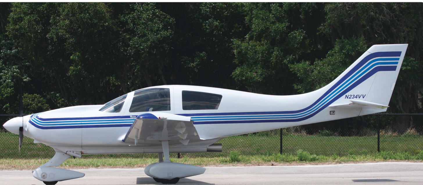
From the fuselage stripe up, everything in and on the fuselage was designed and molded by the builder's group that formed when it was obvious they weren't going to be receiving their kit parts from the former company.
