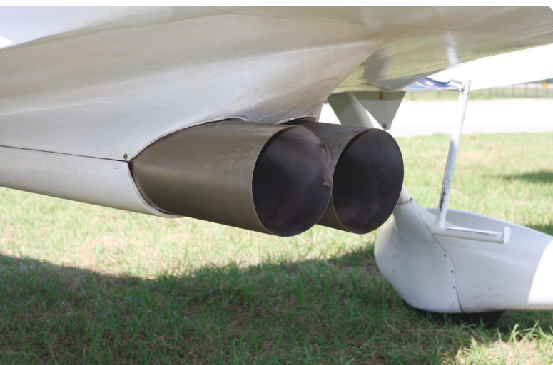
Equal-length headers feed into 6-inch augmenter tubes that help suck air through the radiators and out the cowling and under the fuselage.
