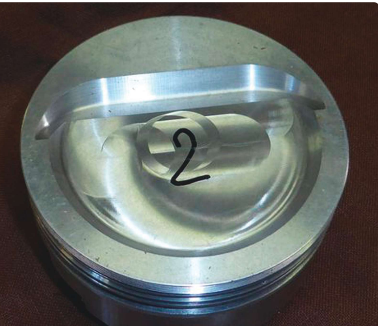
The piston has cutaway for combustion and valve clearance.
