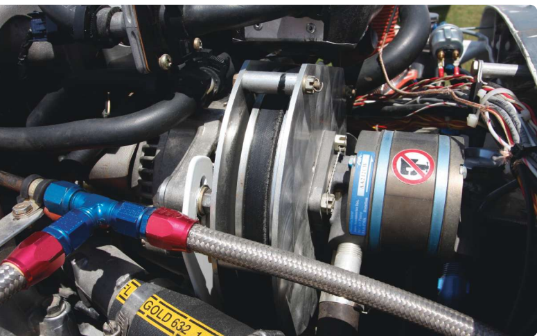
Victor fabricated a pulley and bracket to mount the automotive alternator and vacuum pump while also reducing the rpm of both to proper levels.
