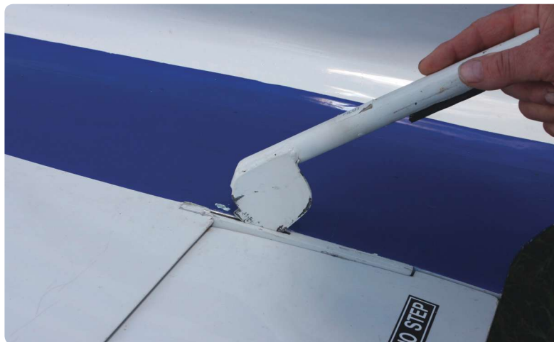
The removable step is another Holmlund innovation. A small, notched blade fits in the top of the wing...
