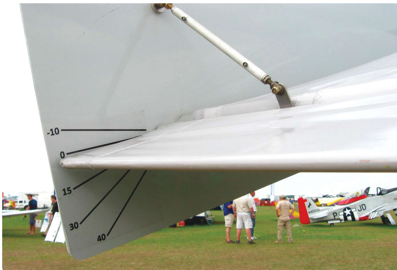
The outboard end of Ray's full-span flap.
