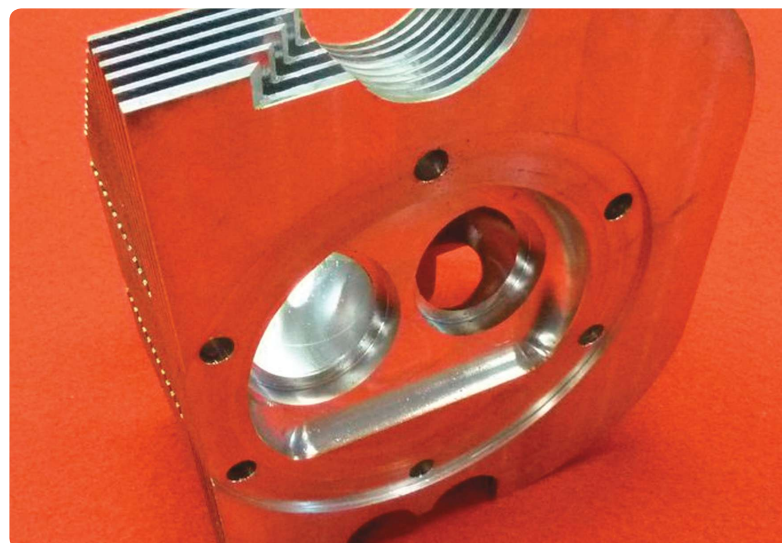
Nearly finished head shows generous finning.
