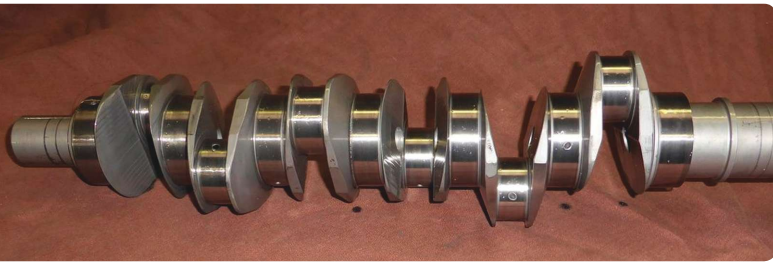
The 7-main crankshaft is well-supported.
