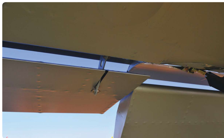
Just Aircraft's SuperSTOL pairs a huge Fowler flap on each wing with an equally large slotted aileron to assure positive control at below-belief angles of attack and below-scale airspeeds.
