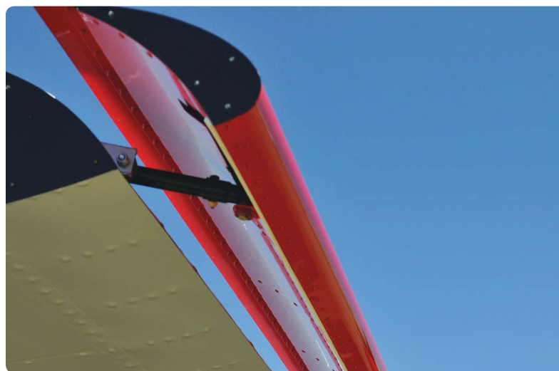
Just Aircraft's SuperSTOL employs a pair of automatic slats on each wing, hinged to retract and extend as airspeed warrants, with slower-than-usual speeds the result.
