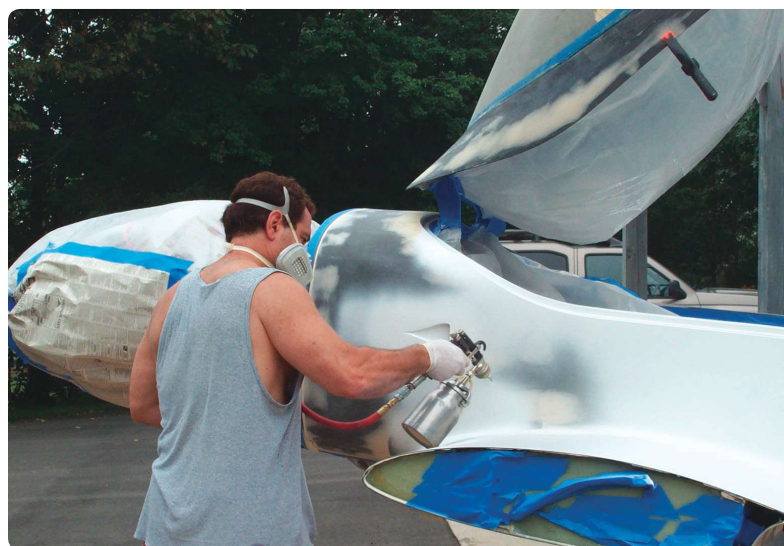
Jay works on the fuselage in the primer stage.
