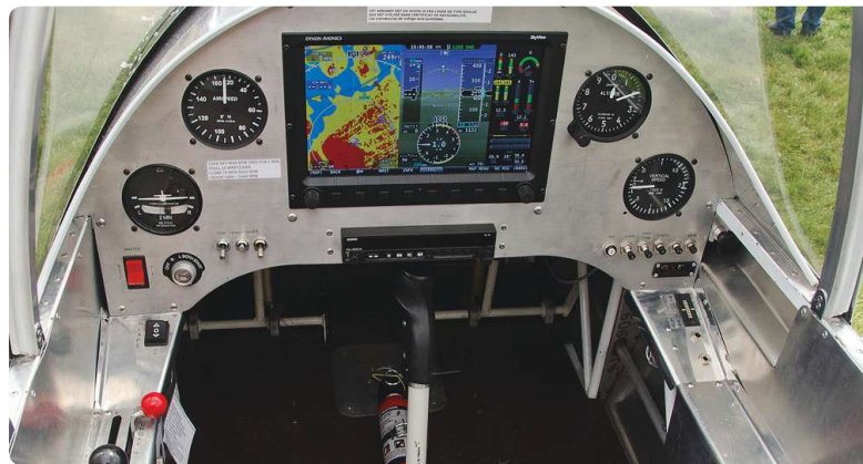
Digital and analog instruments provide primary and backup information in a neat arrangement on the panel.
