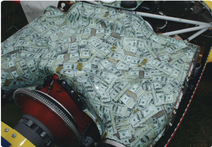
The builder of this RV-7A shared his thoughts about the cost of this 210-hp IO-390 engine by covering his plenum with the image of dollar bills.
