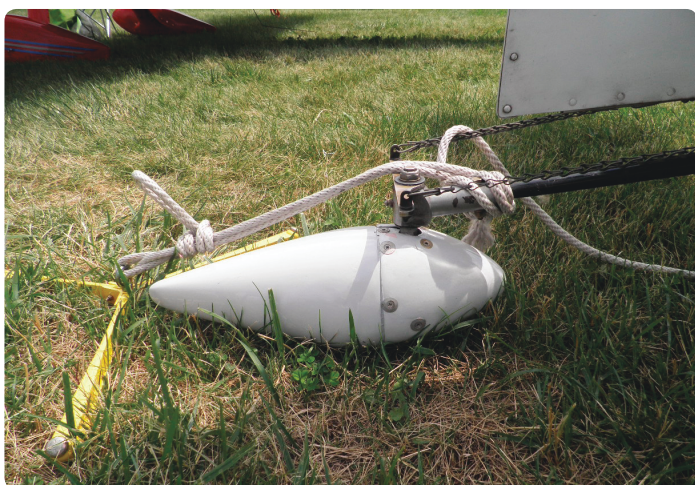
We believe the smallest wheel fairing seen on the AirVenture flightline belongs to an award-winning Thorp T-18 completed by Ronald Hayes in 1992. The tailwheel fairing is only about three inches in diameter.
