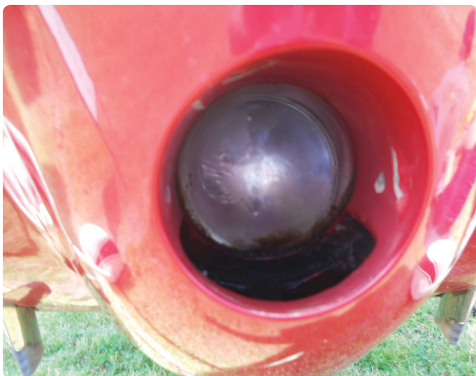
The builder of this Tailwind added a landing light inside the air scoop on this vintage homebuilt.
