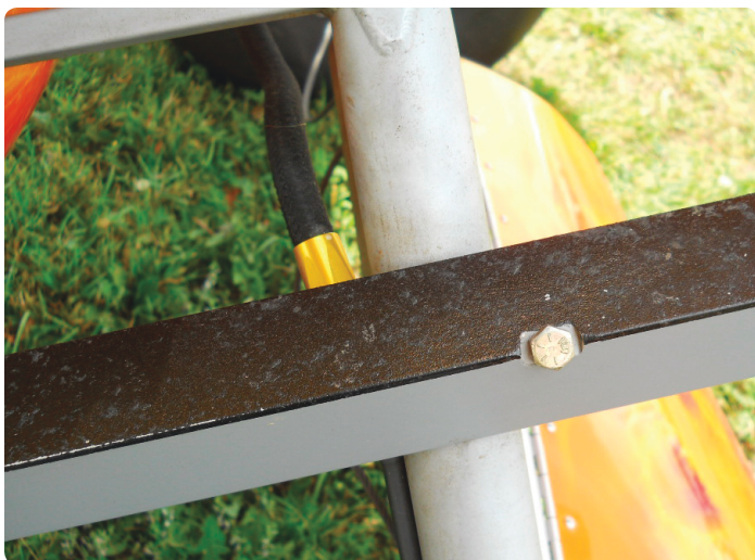
Look at the step on this bushplane. It's a section of angle aluminum with some slip guard added. It is held on with a simple bracket...brilliant!
