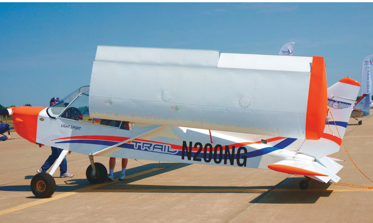
The Trail LSA from Italy folds its wings quickly and easily.
