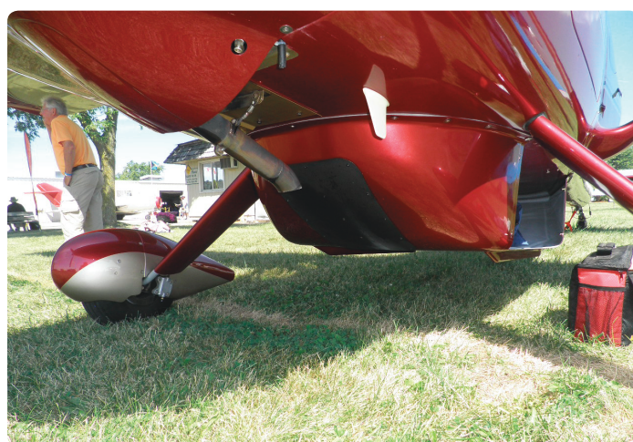
This nicely finished Sportsman GS-2 was completed in 2012 by Gordon P. Anderson. The belly pod appears to be in the exhaust stream, requiring a longer exhaust pipe and a protective pad on the pod.
