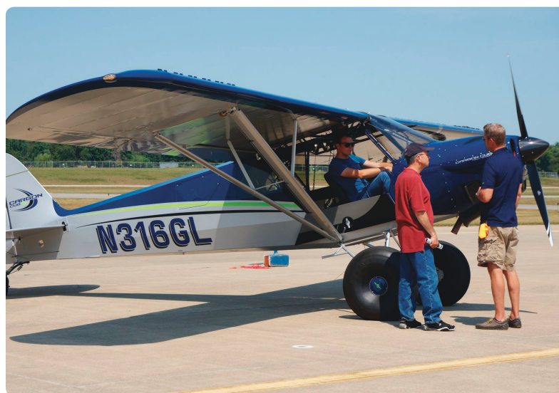
The Carbon Cub LSA fitted with tundra tires.
