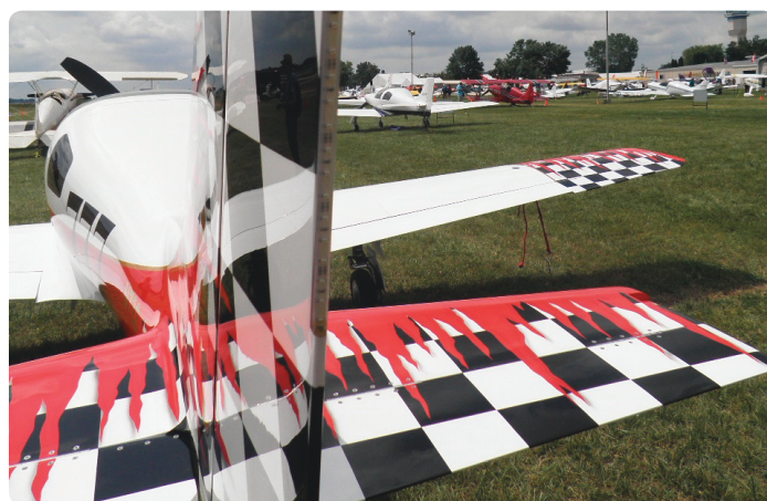
This award-winning Lancair 320 was completed by Craig W. Schulze in 2007. It has a clever aft navigation light built into the trailing edge of the rudder. The LED strip is perfectly faired into the rudder.
