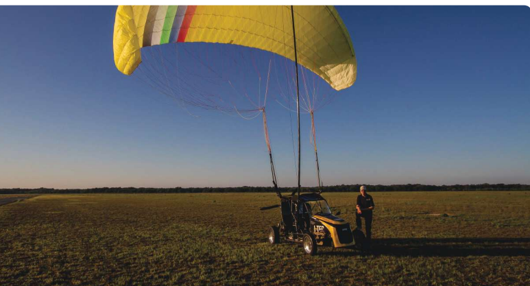
Mast and leading-edge spar system eliminates the need to "kite the wing." The single mast allows the wing to "weather vane" so no load is put on the mast, avoiding tipping forces and allowing crosswind takeoffs by keeping the wing overhead and not allowing it to drift downwind, creating sideways lift.
