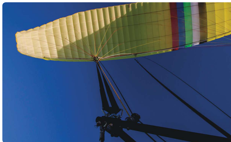
Wing and wing mount arms showing risers, suspension lines, and trim and steering lines.
