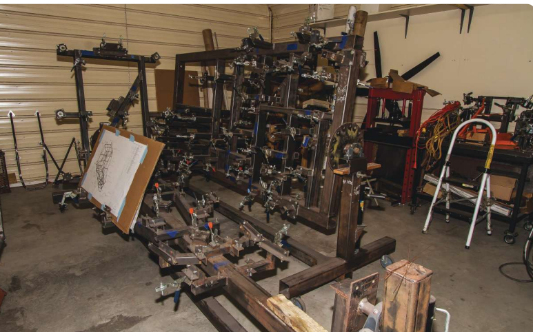
The welding jigs were designed and built as a school project by students at LeTourneau University's mechanical engineering program in Longview, Texas.
