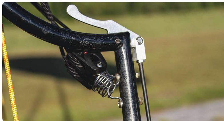
Maverick has a line controller on the right side of the cockpit that gathers the slack out of the parachute wing lines before takeoff to keep them clear of the propeller until the weight of the car straightens the lines.
