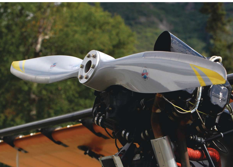
Frank uses an 80-by-30 Catto propeller that really bites into the air.
