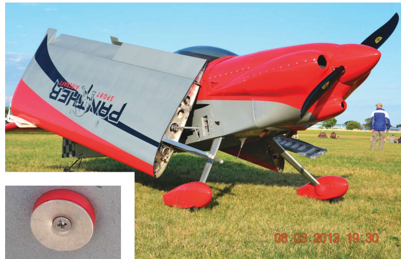
Inset, the isolator used for the automatic connection of the fuel sender unit in the wing. It's created by the 3D "printer."
