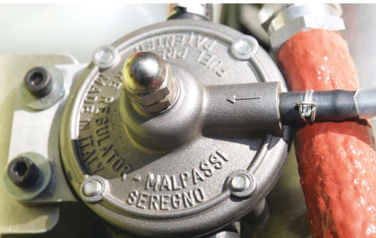
This "altitude corrected" fuel-pressure regulator is very sensible component that a specialised manufacturer developed and calibrated for this turbo-kit.
