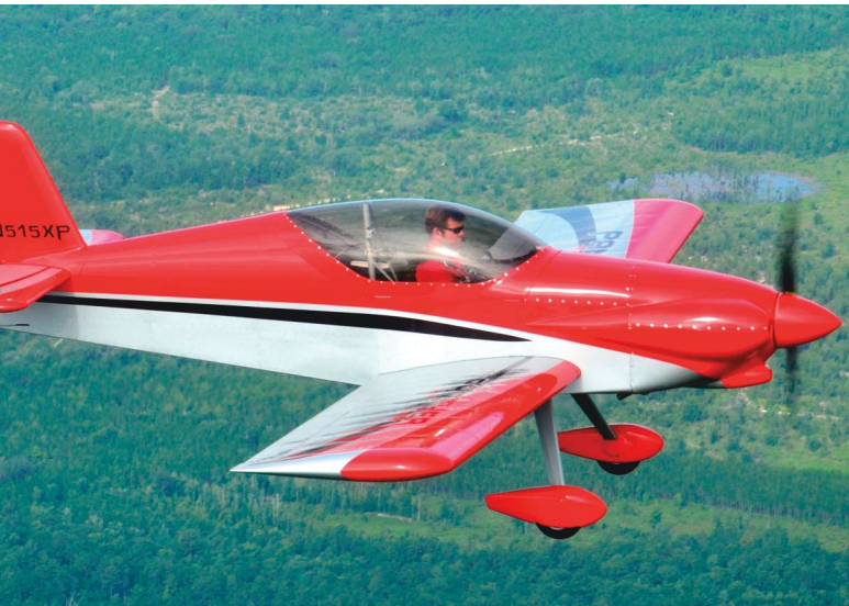
The Panther in flight. It can be built as either a tail dragger or tri-gear.
