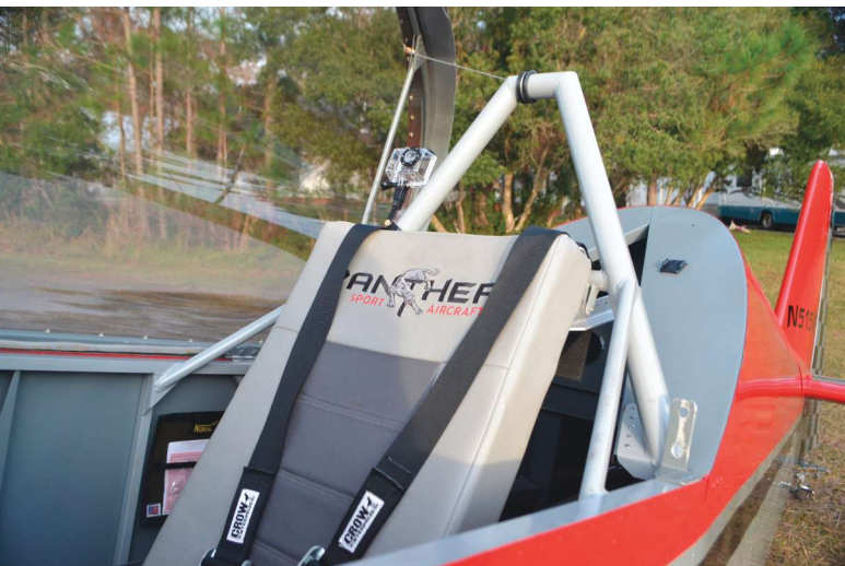
The single-place Panther has a sturdy roll-over structure.
