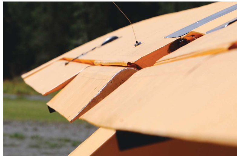
The flaps go all the way down to 70 degrees and the ailerons droop at the same time. At maximum deflection, the ailerons are down 22 degrees.
