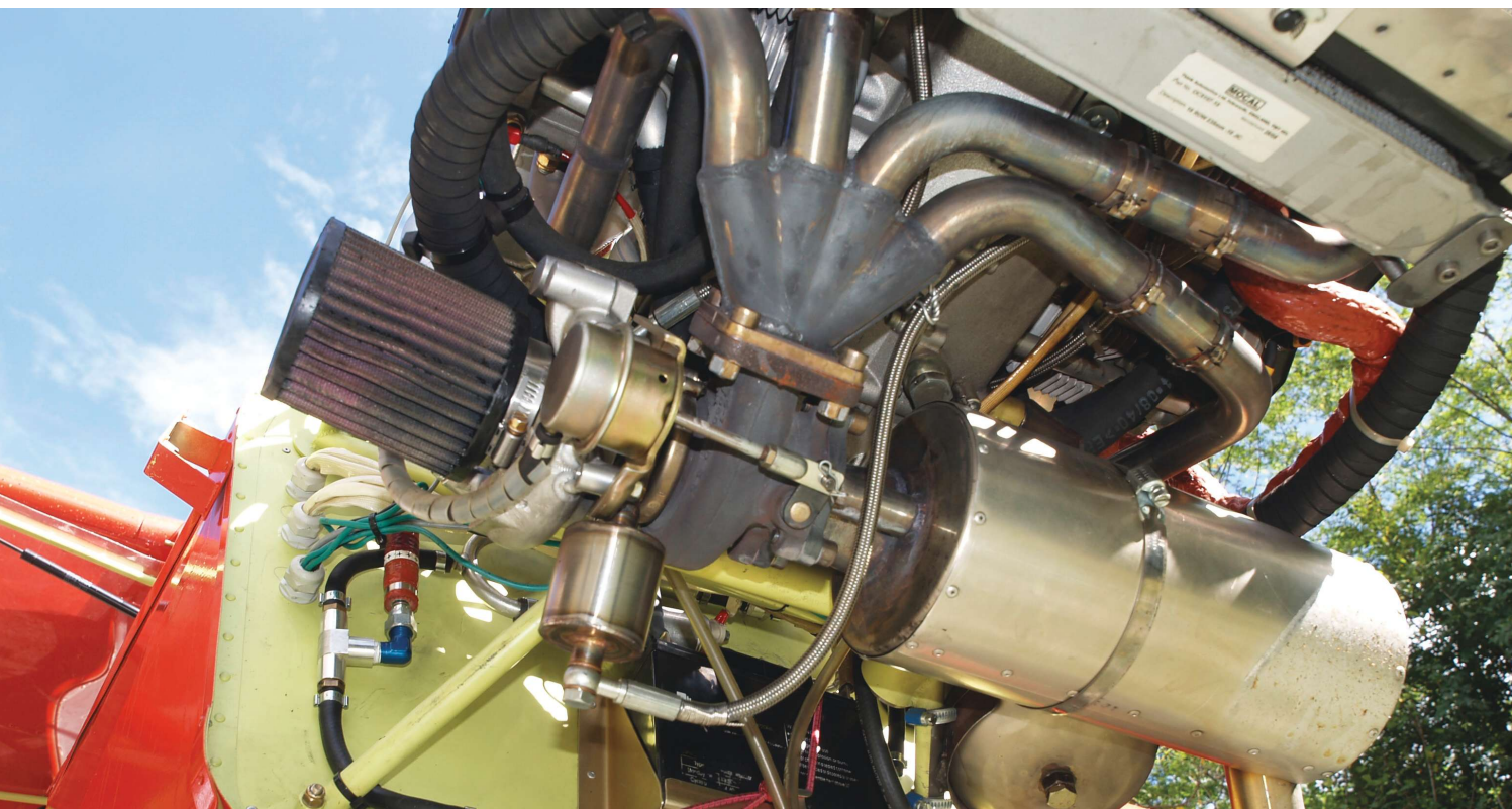
The view from below to the turbo assembly; note the silencer that is directly bolted to the "hot" side of the turbo charger.
