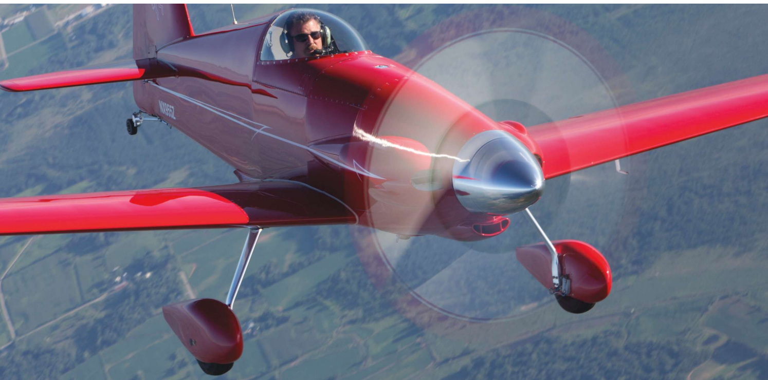
Put on its nose at some point, the Midget Mustang's original landing gear was replaced by Shaw with Grove gear legs, which are gun-drilled and airfoiled.
