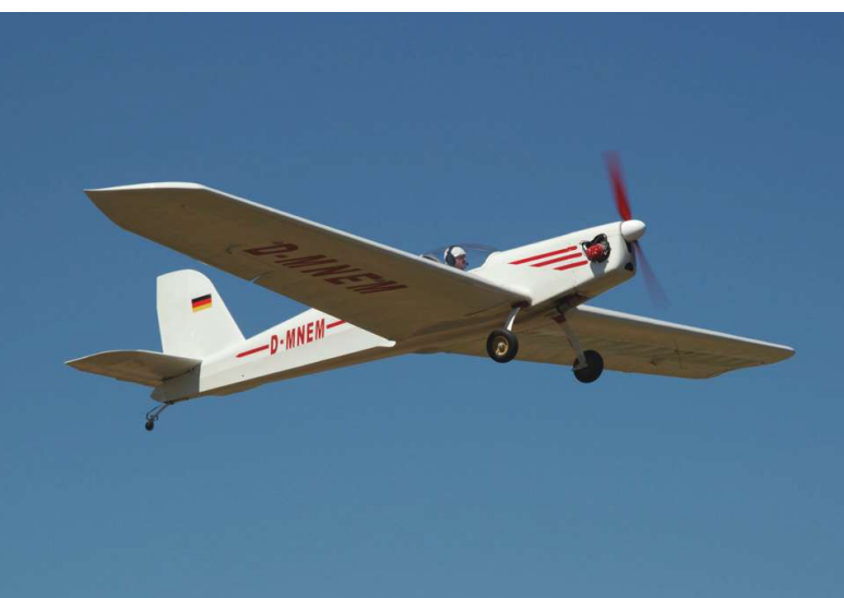
The ULF 2 is a very light, plans-built, wood motorglider from the same designer.
