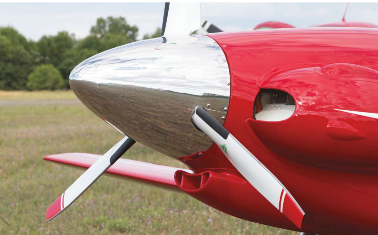
The MT composite, electrically controllable propeller greatly improved the airplane's performance both on takeoff and cruise where it indicates 160 mph at 5.7 gph.
