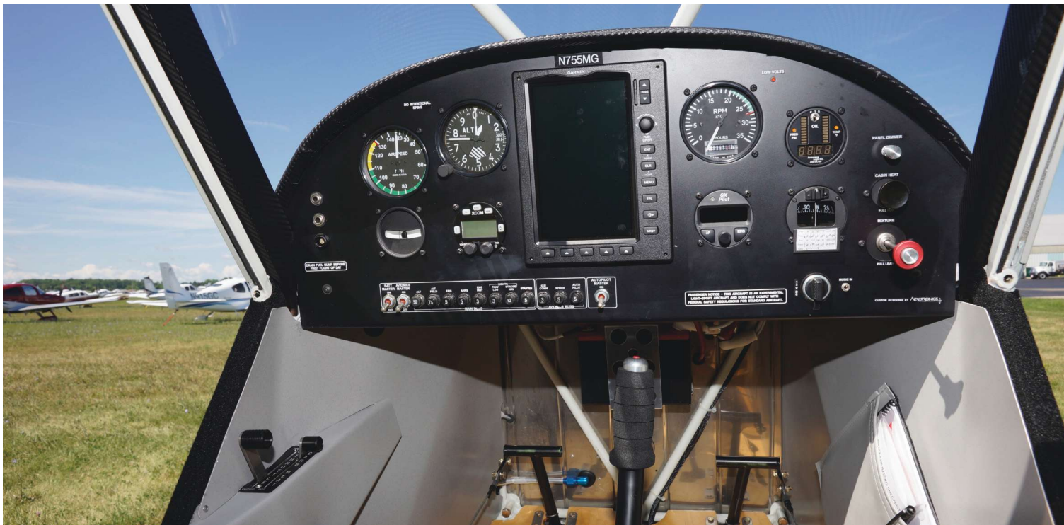
In addition to traditional round instruments, Craig added a Garmin G3x flight display and TruTrak autopilot.
