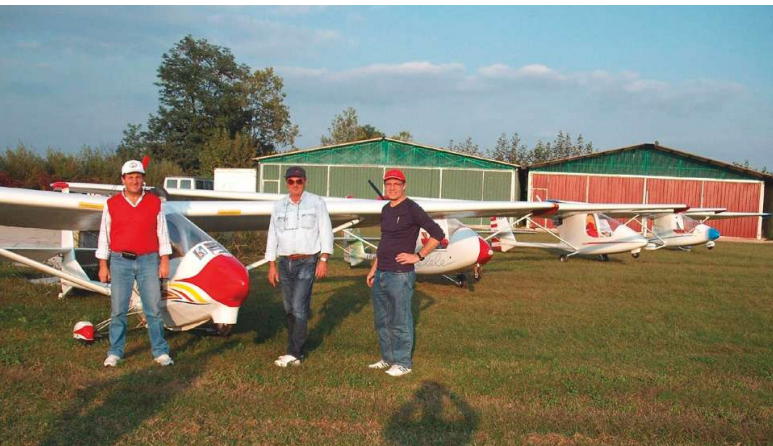
A Piuma Project glider get-together. Piuma's are light, plans-built, mostly wood, one- and two- place motorgliders.
