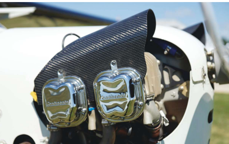
Craig chose the optional Continental O-200D engine because of his good experience with the Continental engine in their Lancair IV-P.
