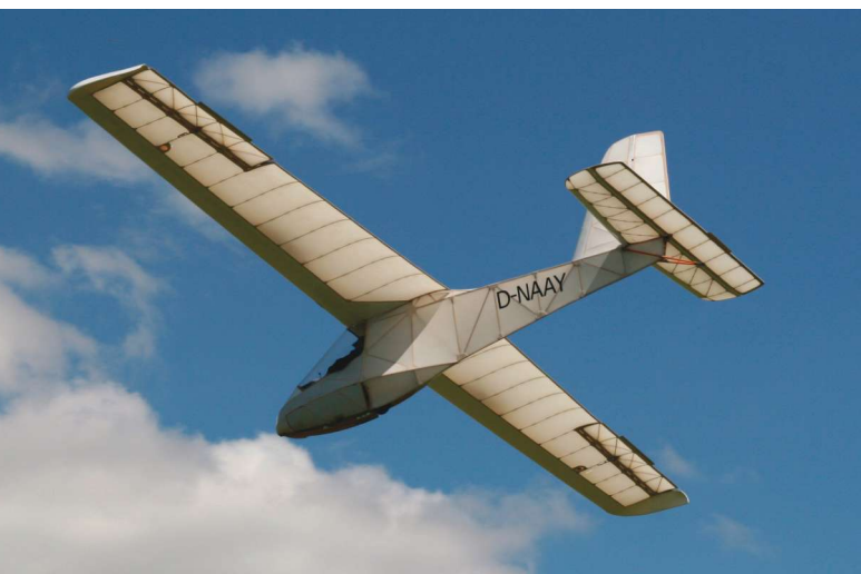
This is a ULF-1 glider; it is a foot-launchable, plans-built, wood ultralight sailplane from Germany.
