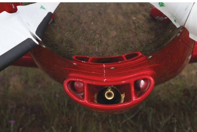
There is no filler or fiberglass in this photo: it is all formed aluminum.
