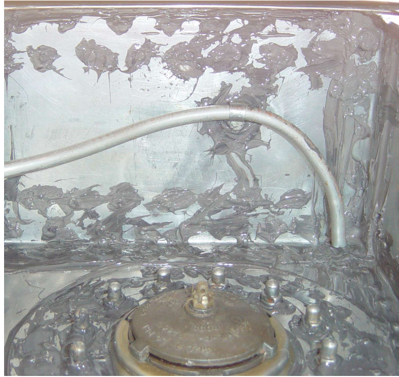
3. After using Pro-Seal on the fuel filler and vent.
