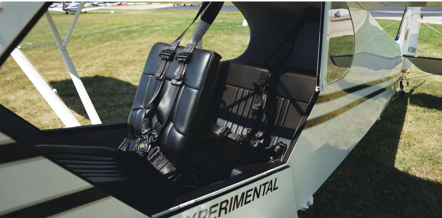
The cabin of the Legend Cub is 28.5 inches wide and 50 inches tall, much roomier than the original Piper Cub.
