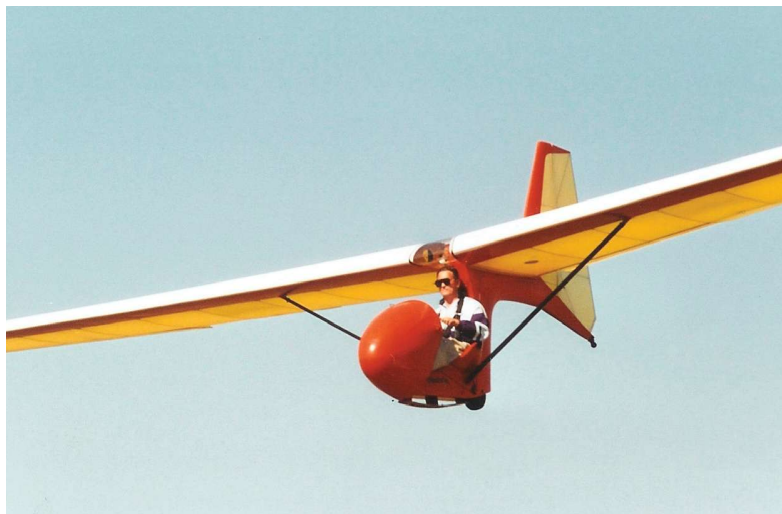
A Marske Monarch on final. The most successful flying wing and tailless aircraft have been sailplanes.
