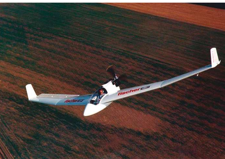
A Mitchell U2, plans-built, mostly wood ultralight flying wing motorglider.
