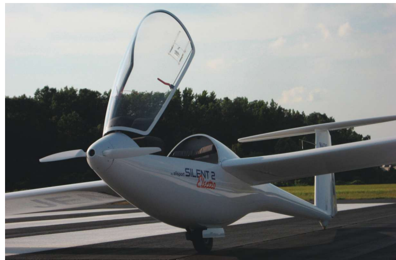
The Silent II Electro has a small electric motor in the nose and has self-launching capabilities. Electric flight is available now!
