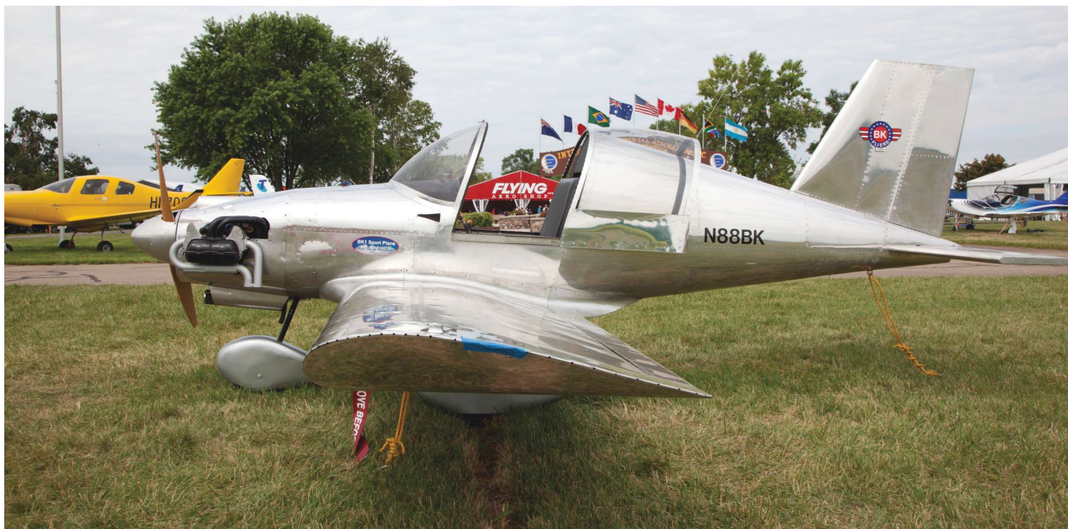
The fuselage and empennage are flush riveted, giving the BK Flier a neat and sleek appearance.
