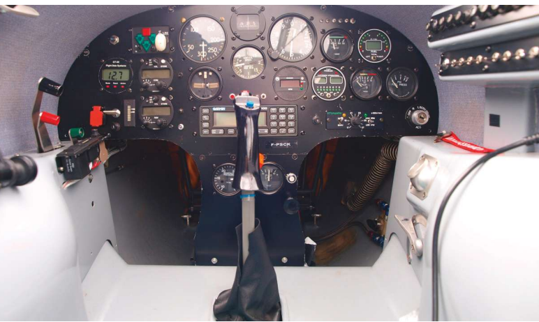
The front cockpit of the CC02. On the left side are the throttle and the prop pitch lever; just to the right of it, the rather complex flap selector lever.
