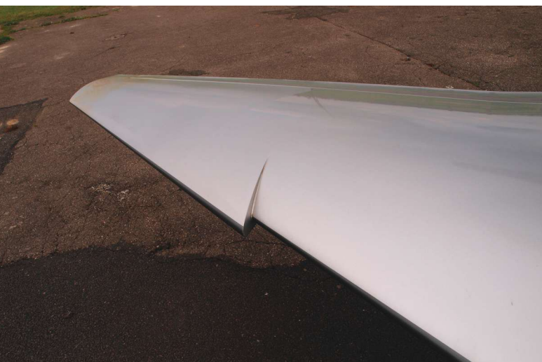
The dropped wing leading edge offers low-speed wing efficiency.
