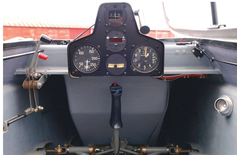
The rear cockpit is pretty spartan as the aircraft is primarily flown from the front seat.
