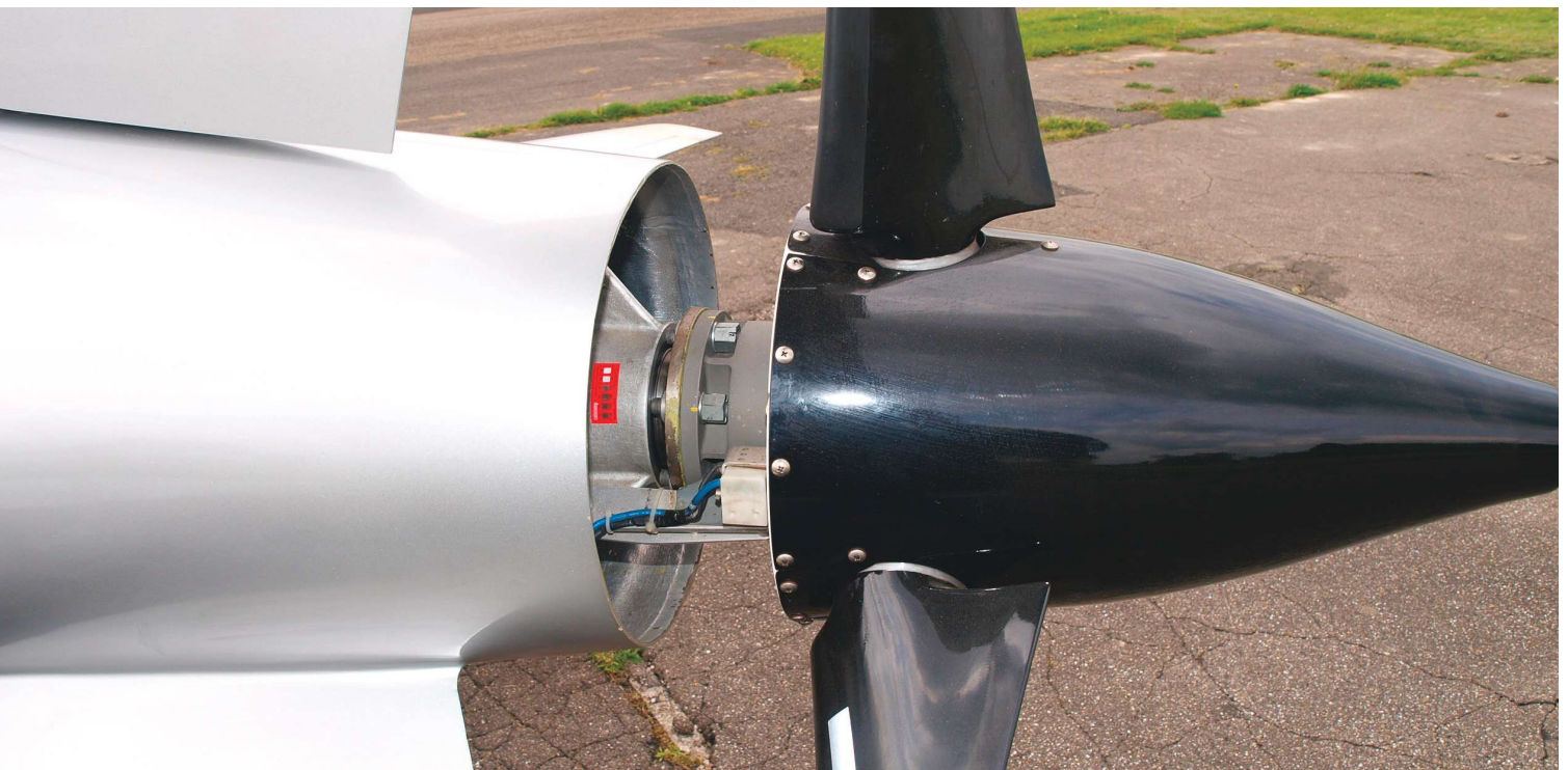
It has an electrically variable pitch prop. The first prop was a fixed-pitch prop.
