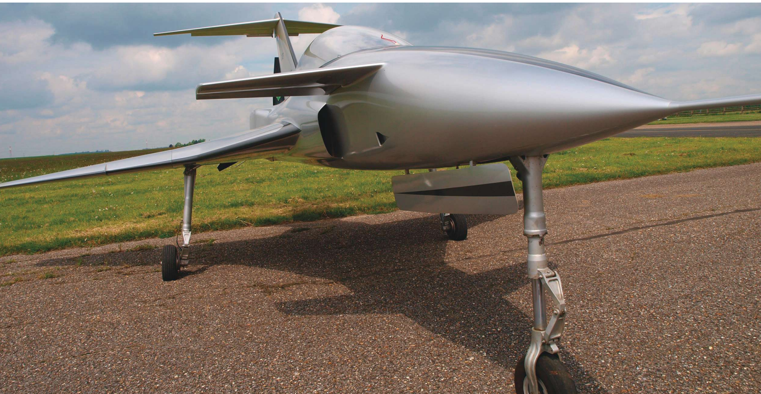
The CC02 has three lifting surfaces—a canard, the main wing, and a flying tail. Claude said this arrangement helped him solve the problem of the wide CG range.
