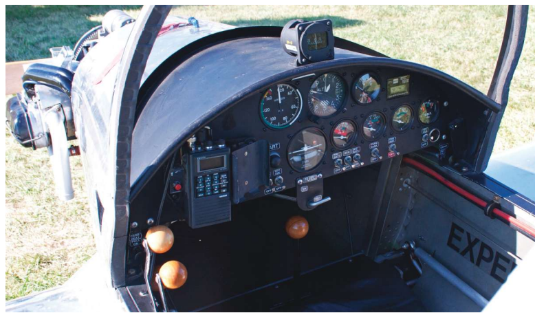
The BK1.3 has electric start and a full complement of instruments for cross-country flying.
