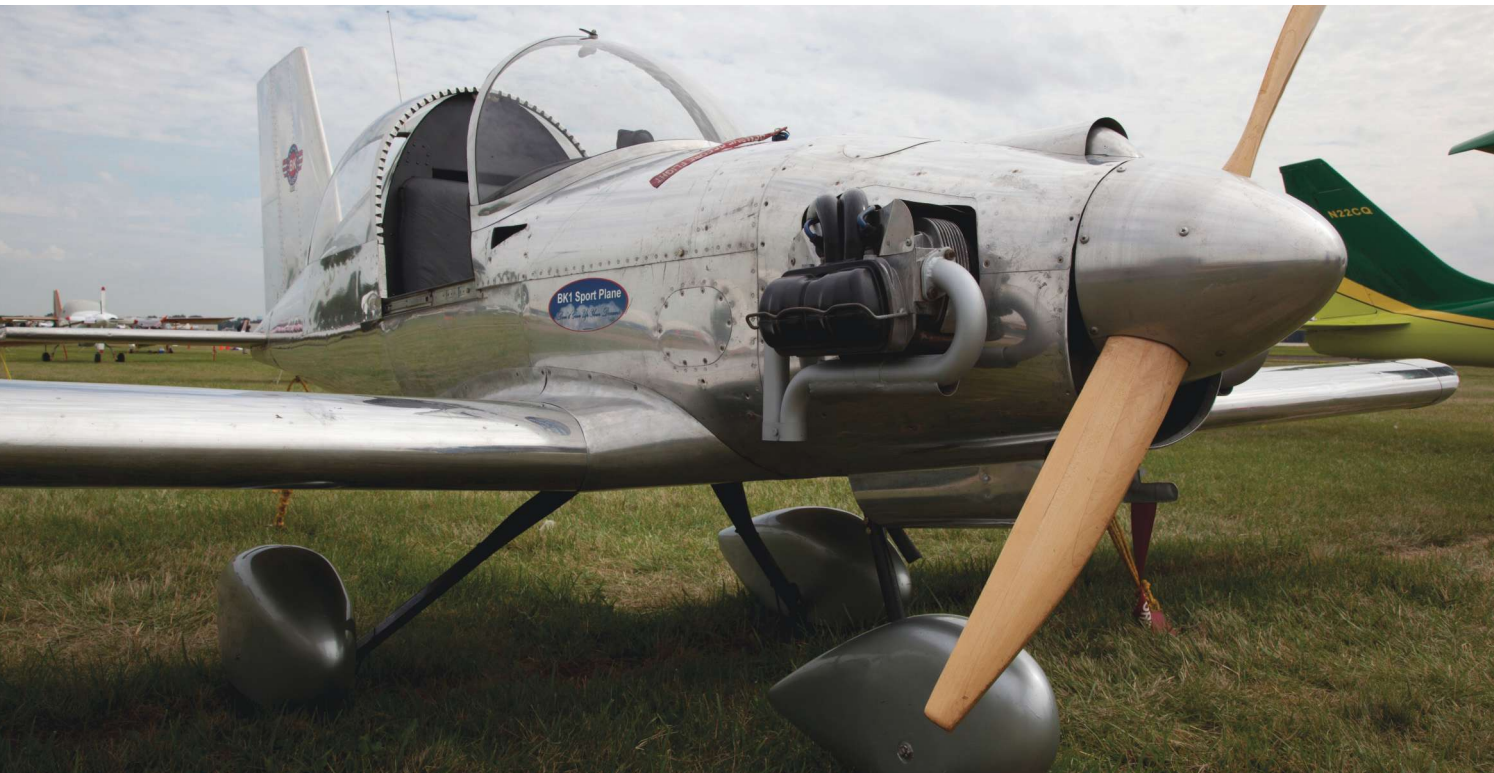
Though small in size, the BK1.3 can carry 30 pounds of baggage aft of the seat. It cruises at 130 mph while burning 3.5 gph, making it a usable cross-country machine.
