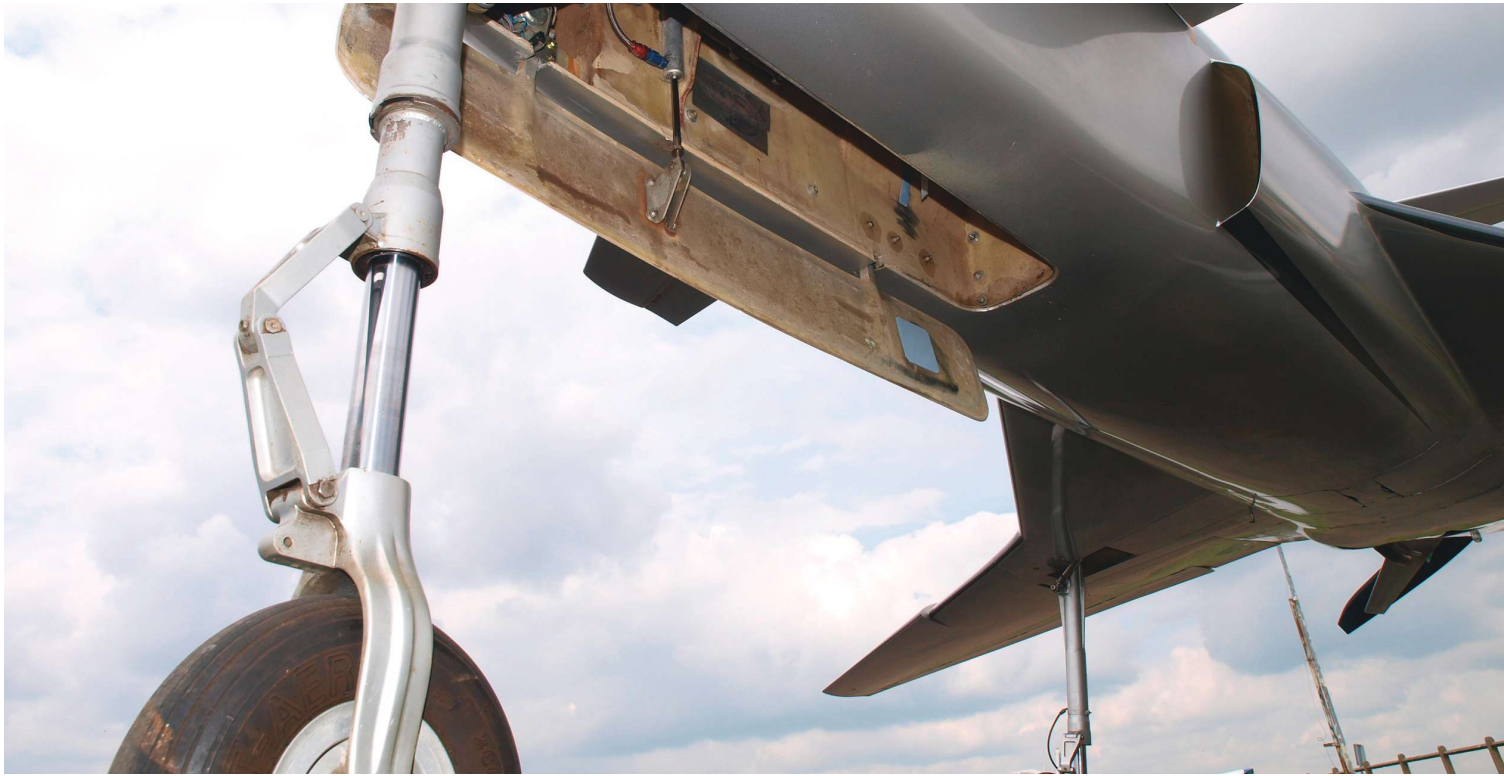
The CC02's fuselage features a clean belly and smooth lines. Note the closed main gear doors even while the gear is extended.
