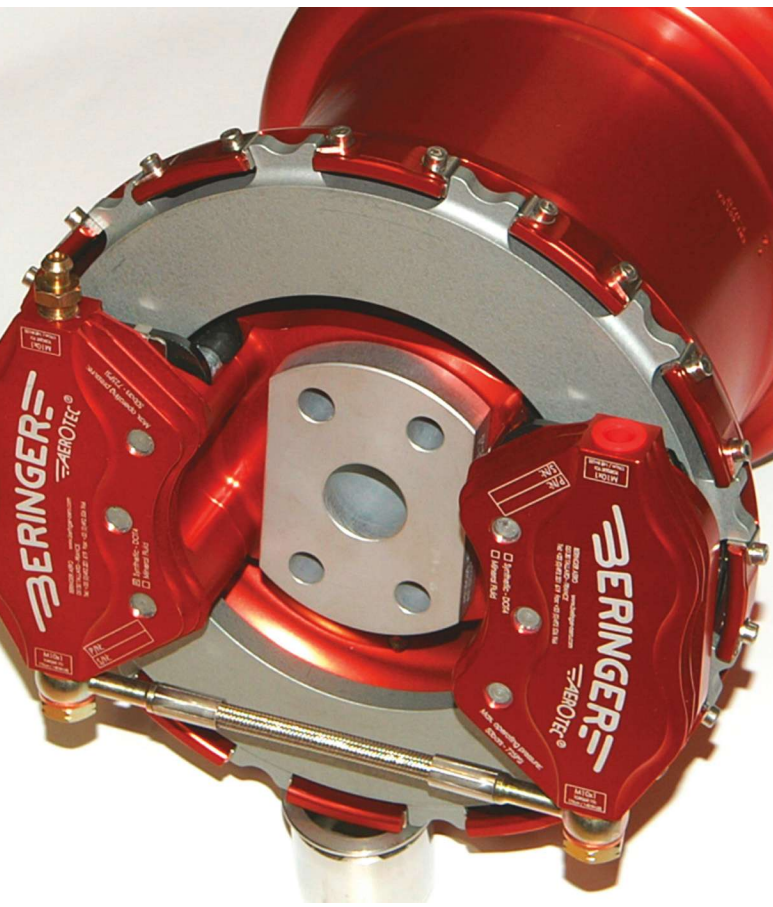
For fast-landing or heavy airplanes, or an aircraft with tundra tires, one caliper may not be enough.
