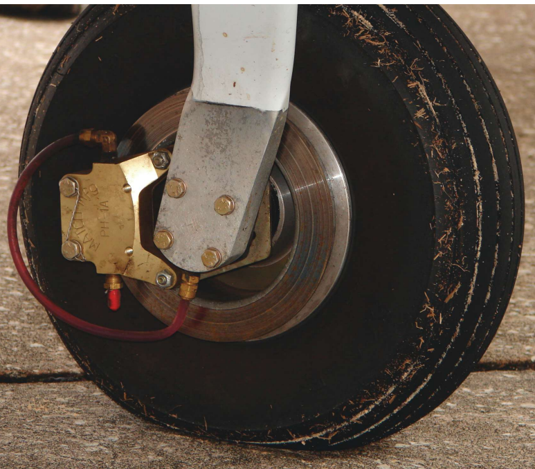
When well-protected and where flexibility is not critical, clear brake lines can save ounces.
