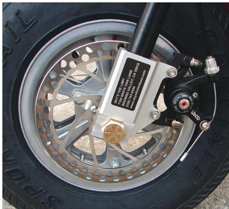
Very light, very small aircraft don't need a lot of braking power. This Infinity powered parachute carries only one tiny, cable-operated brake on the front wheel.
