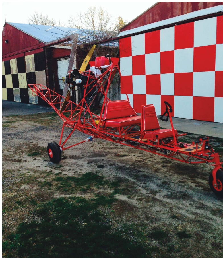
The O-200 engine mounted on the steel-tube fuselage, as the project sees daylight for the first time.
