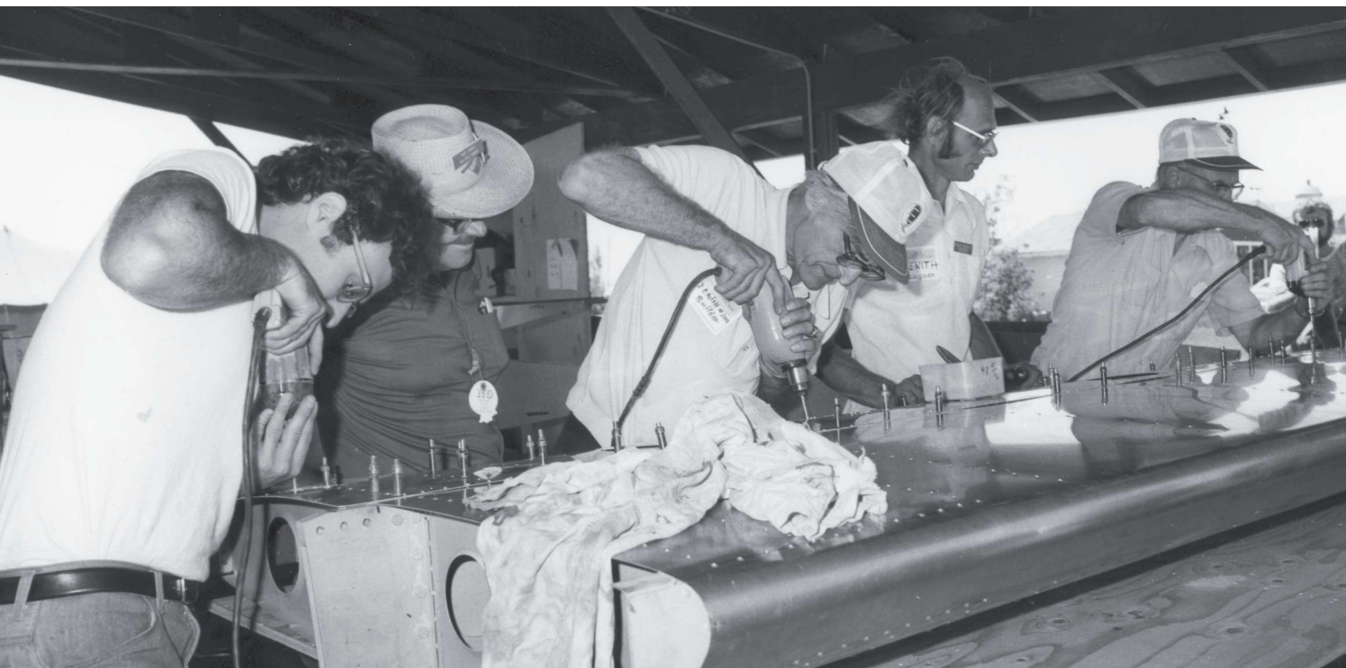
Zenair founder and designer Chris Heintz (second from right) watches as Zenith staffers riveted the wing skin on a Zenair CH 200 at Oshkosh in 1976, completing the aircraft in eight days. Here's a video from that event.
