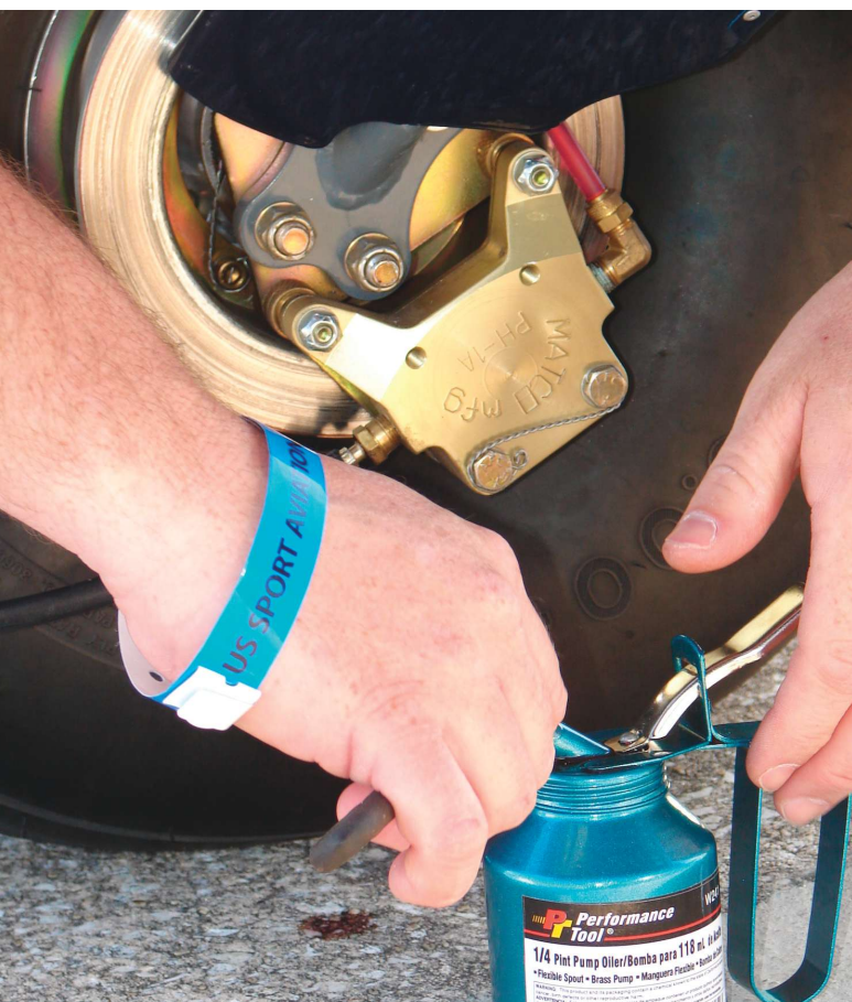
No matter what brakes you have, bleed them frequently and properly, as this RANS employee demonstrated at Sebring.
