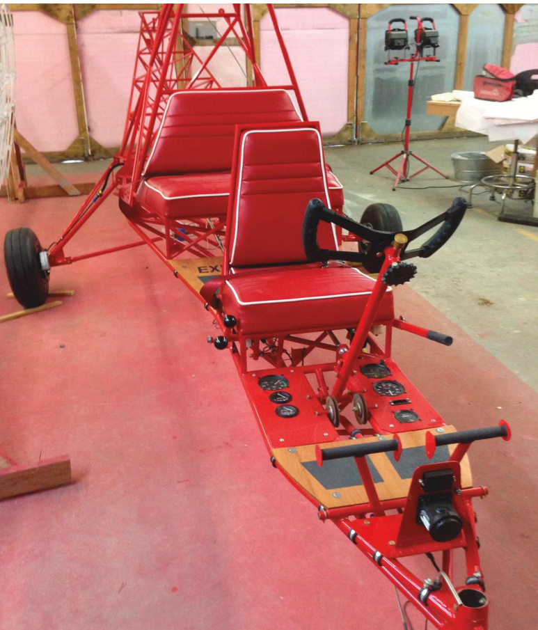
Jon and Mike's Breezy fuselage comes together as they fit the seats and install instruments.
