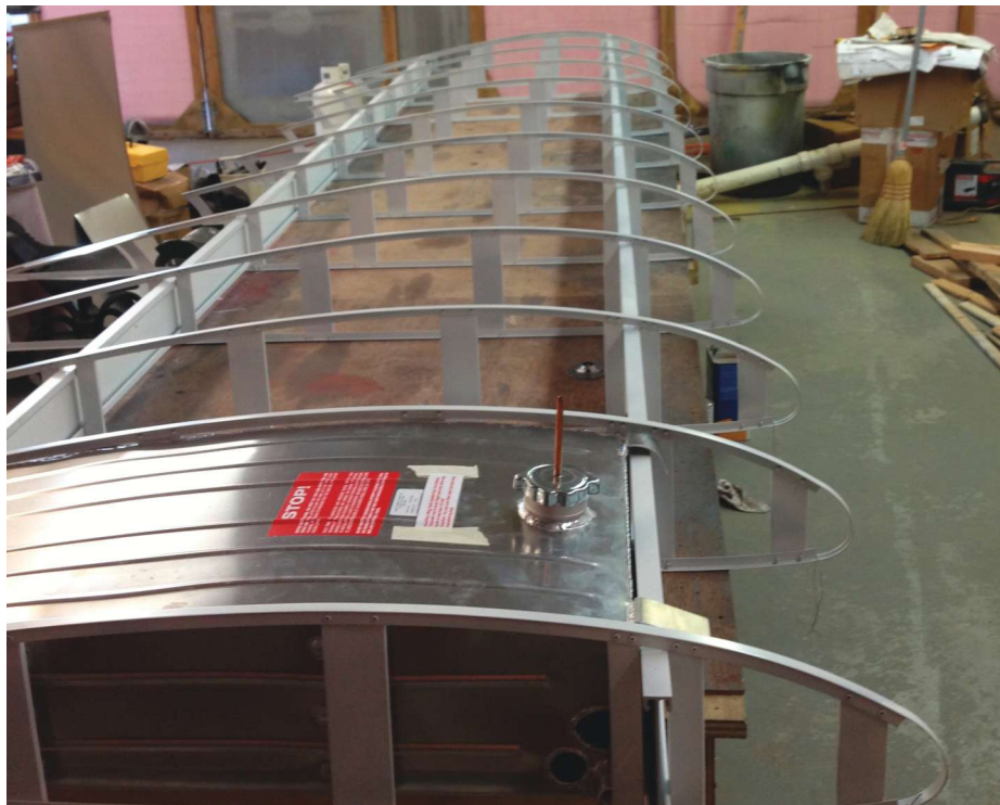
Jon and Mike purchased a wing kit for the Wag Aero J-3 Sport Trainer to build their all-metal wing.
