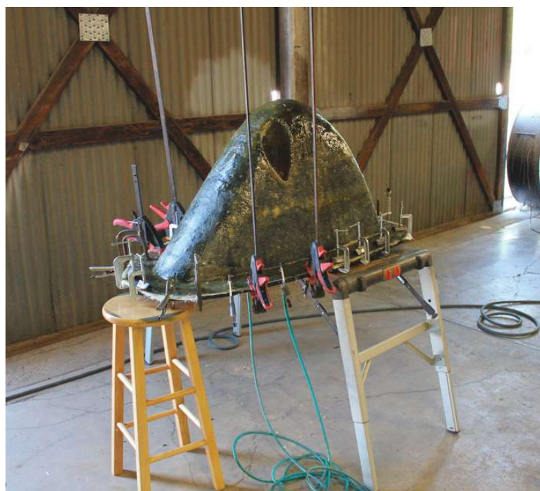
It took a considerable amount of preplanning to figure out how to extract the nose cone's female mold from the male plug. What we ended up doing is pre-drilling holes down through the inlet ducts and inserting air fittings on the bottom of the male mold, which allowed us to pump air pressure in between the female fiberglass mold and the male plug. In this picture, the air hoses are hooked up to the bottom of the plug forcing air in between the two components. We were able to exert force throughout the entire component and separate the two pieces.
