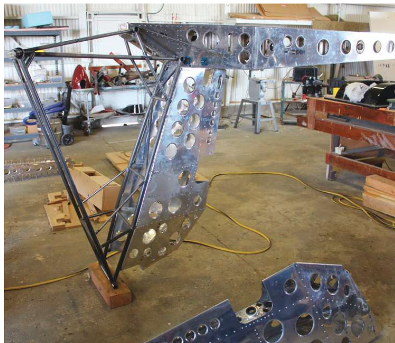
The aft fuselage fairing assembly installed, which incorporates the aft motor mount. The fairing attaches with one bolt and 5 screws on each side of the fairing, making it relatively simple to remove for maintenance and or inspection.
