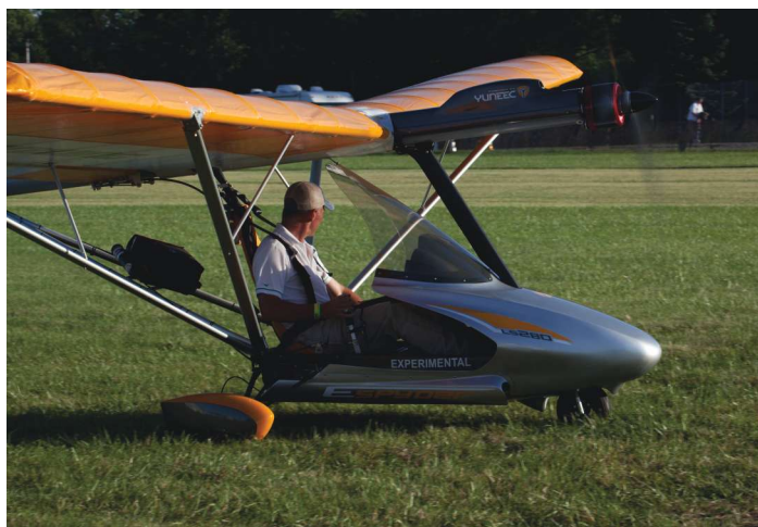
The e-Spyder is one of several electric-powered ultralights in development at this time. The e-Spyder is based on the original Flightstar ultralight design. www.greenwing.aero
