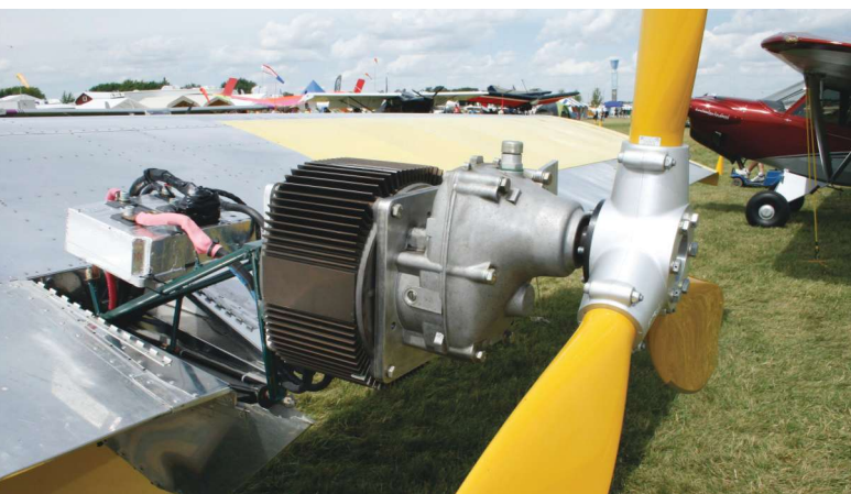
This is the electric motor on Mark's 2013 machine; while it flew acceptably well, Mark wanted more performance for the aircraft so began designing a second motor...and that's when serendipity entered the process.
