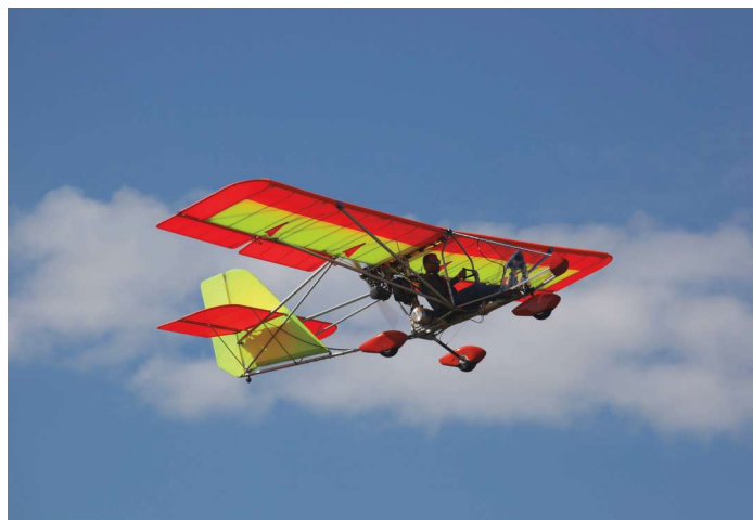
The Aerolite 103 is an example of a tube-and-fabric ultralight that's offered as a ready-to-fly machine. A variety of engine options are available. www.uflyit.com/aerolite103main.htm
