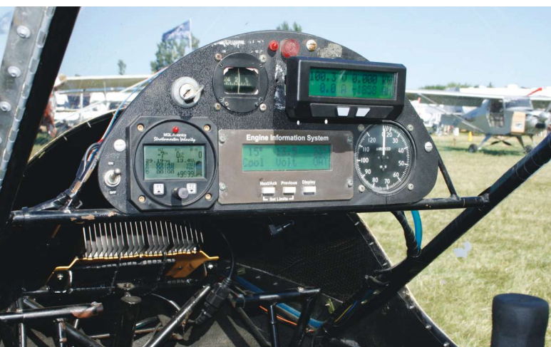
While not a thing of beauty, the instrument panel for Mark's e-Gull provides all the information he needs...including information in the upper right gauge on the electric motor's performance and the state of its batteries.
