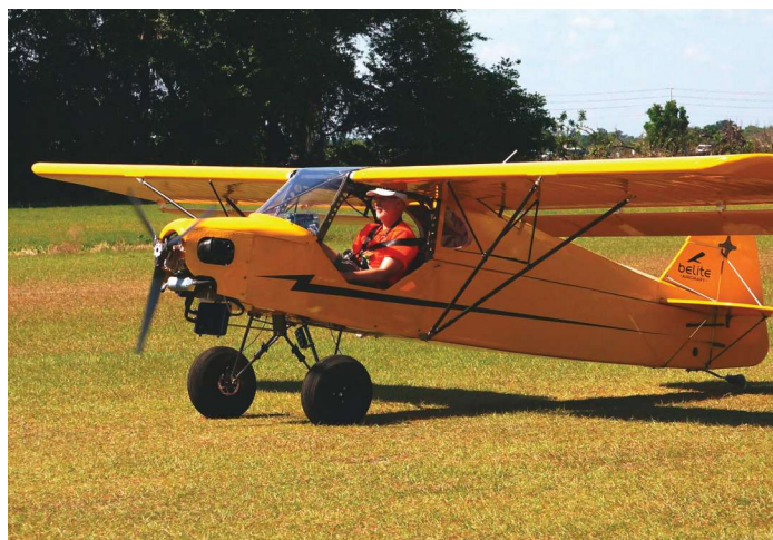
The new Belite ProCub, flown by designer James Wiebe, features extensive use of carbon fiber and foam construction to stay under the ultralight weight limit of 254 pounds. www.beliteaircraft.com
