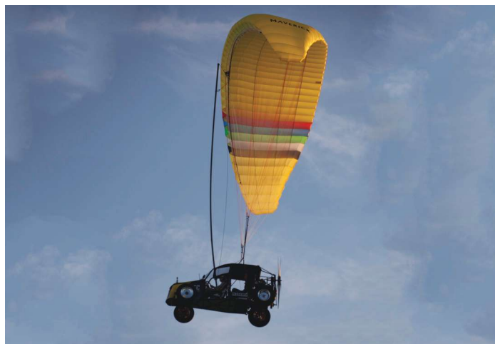
This Maverick powered parachute sports a "My car is an airplane" slogan exemplifying the design concept behind the Maverick light-sport aircraft, which is a very capable and sporty ground vehicle that also functions as a powered parachute. www.mavericklsa.com
