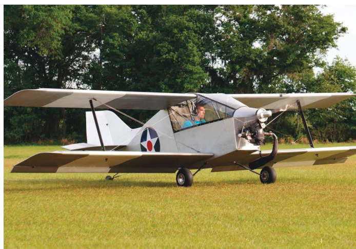
Jonathan Amundsen of Winter Haven, Florida, is flying this SNS-8 Hiperlight, a negative-stagger biplane ultralight design introduced by the Sorrell brothers of Washington state. EAA Founder Paul Poberezny also built and flew a Hiperlight. www.hiperlightaircraft.com
