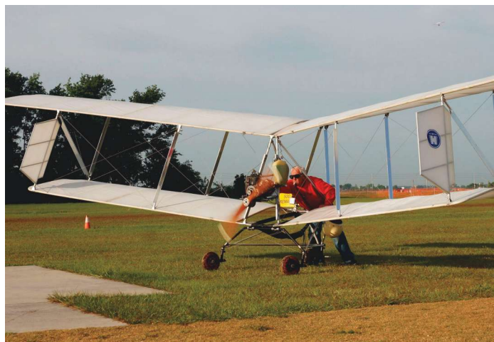
John Moody, first to fly an Easy Riser ultralight in 1975, is seen here in 2014 doing a pre-takeoff static engine check with a mouth-controlled kill switch, a carryover from the early days of foot-launched ultralights.
