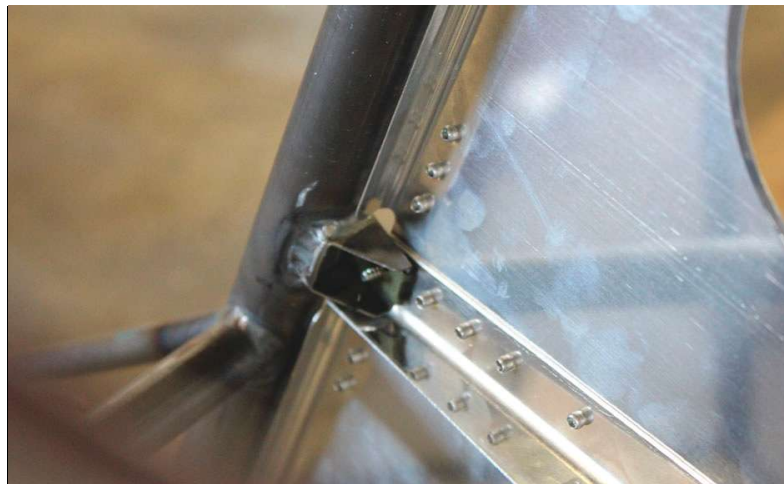
An example of how the fairing is attached to the 4130-steel fuselage frame; \frac{3}{4} -inch square tubing is cut and profiled to make clips to which the Tinnerman nuts attach. These attachment clips were made large enough to be able to incorporate machine screw nut plates or Rivnuts.
