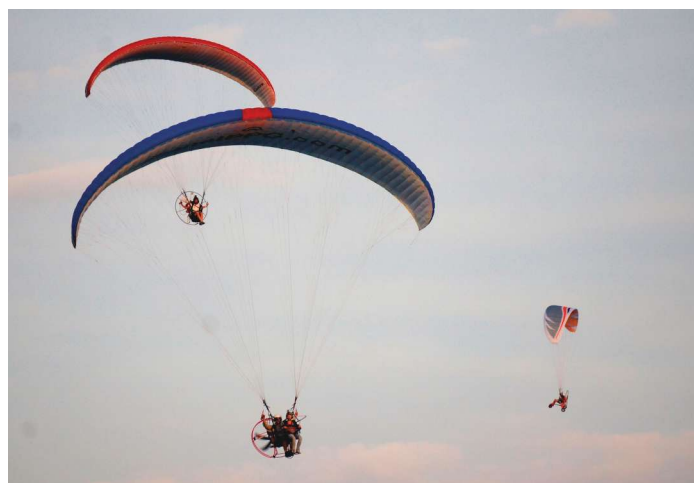
A tandem, foot-launched powered paraglider; a single-place, foot-launched powered paraglider; and a single-place powered paraglider on a tricycle cart represent the three forms available for this type of flying while sharing some premium air time.
