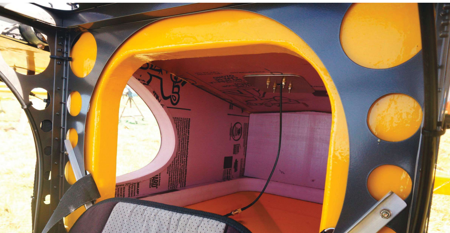
This cabin photo shows the CNC-manufactured aluminum components of the cabin structure and the inside of the turtle deck.
