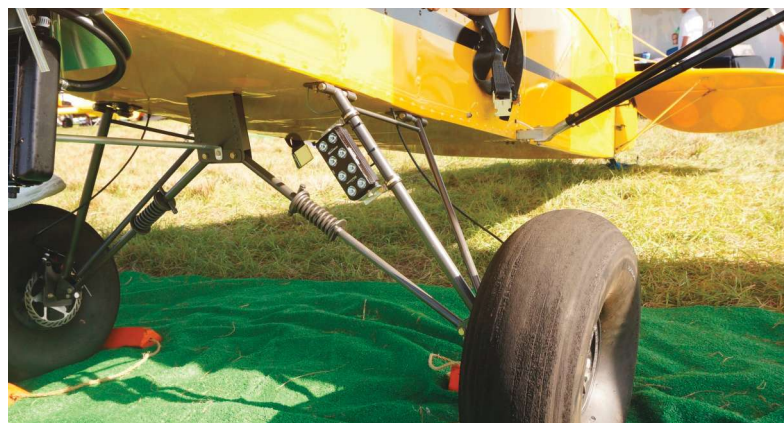
Tundra tires are shaved at considerable expense to save weight, hence their worn appearance...and an LED landing light for obvious reasons.
