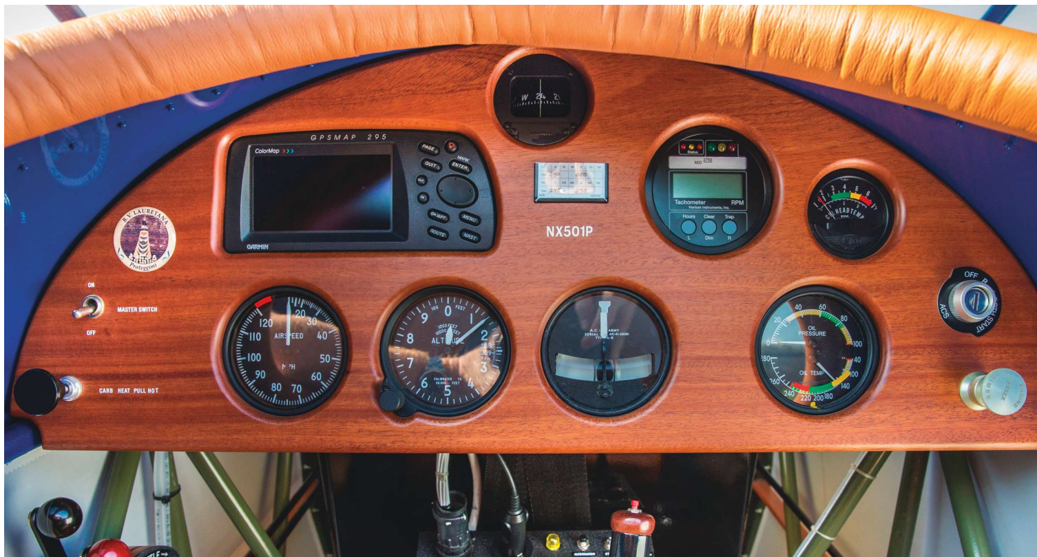
Traditional round instruments maintain the “feel” of the Hatz as an antique homebuilt, with the GPS for modern-day peace of mind.
