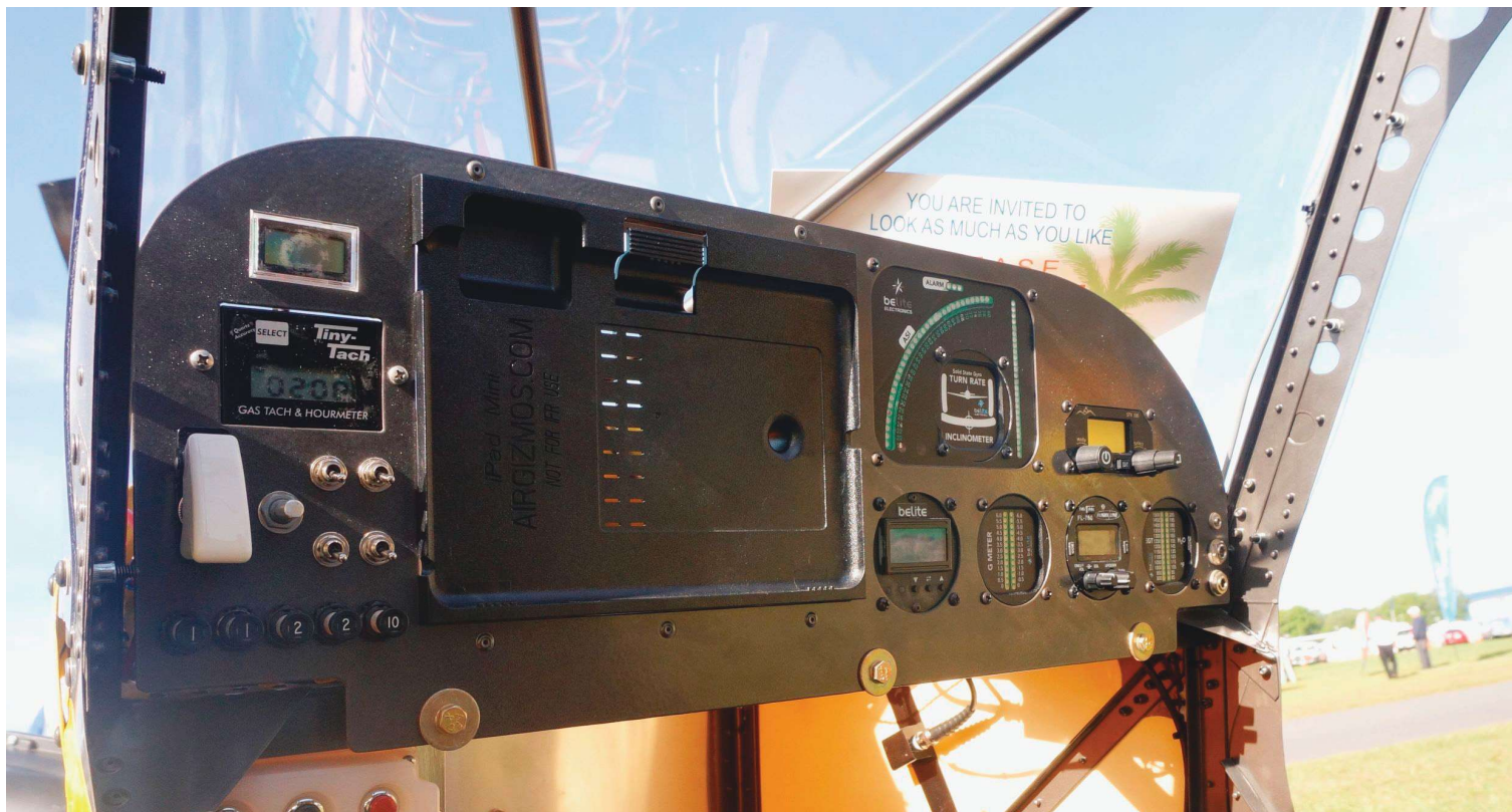
This is Belite's lightweight, simple panel dominated by an iPod dock that could make it very advanced and still ultralight-weight legal.
