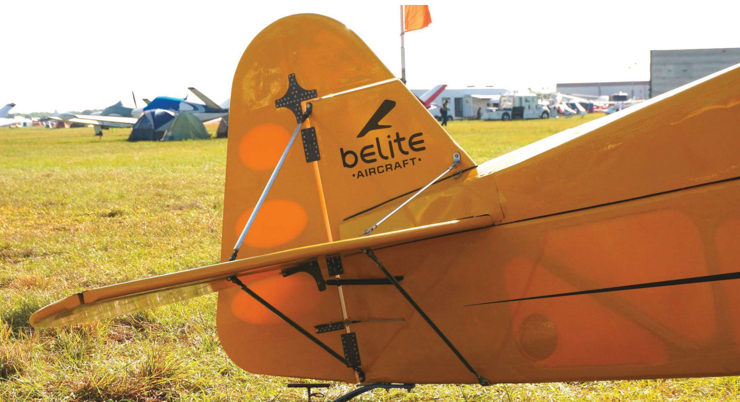
Hinges and gussets can be hidden under the fabric on the ProCub tail built with foam sheets and visible lightening holes.
