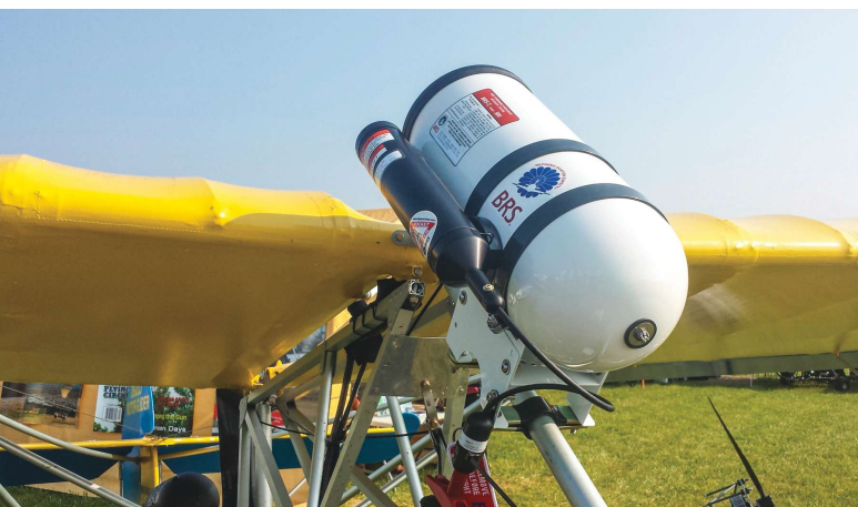
The BRS ballistic chute mounted on the Zigolo ... one of two chute options; the other being the Comelli pneumatic chute.
