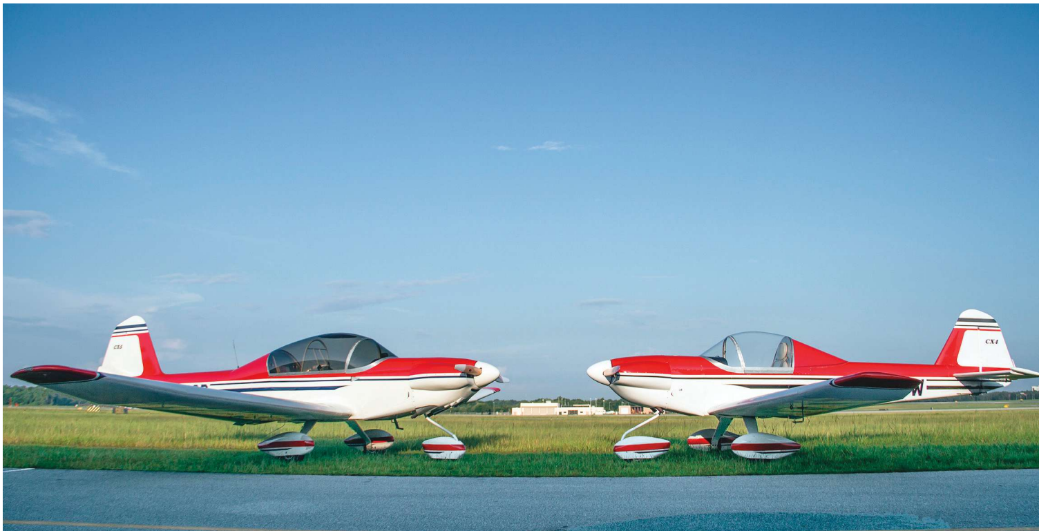
Nose to nose; compare the profiles; two-place at left. The CX5 cockpit is barely distinguishable from the CX4's, but it is several inches wider and taller, measuring a full 28 inches in width (25 inches between the seatback longerons) and nearly 36 inches from the seat bottom to the top of the roll bar.
