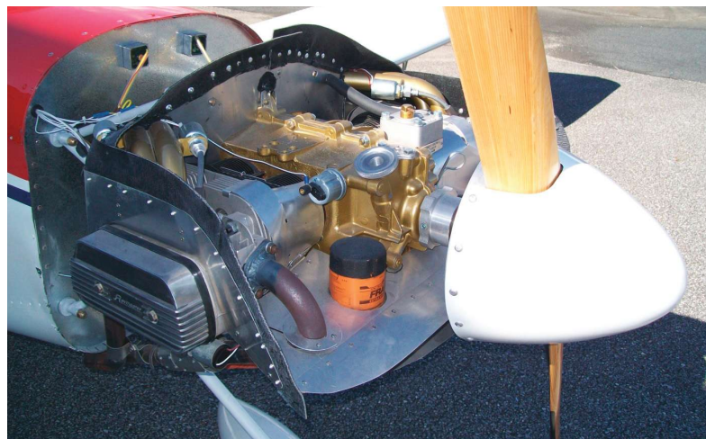
It's no coincidence that the Revmaster R2300 looks at home on the nose of the CX5. It was selected as the engine of choice from the beginning.
