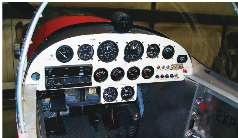
The instrument panel is designed for traditional round instruments, but ingenious builders will no doubt find room for some "glass," too.
