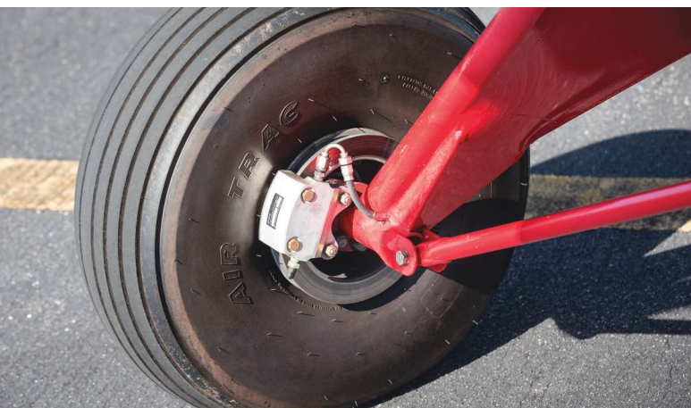
Mark chose to go with small tires because the airplane was slated to go on floats from the beginning.
