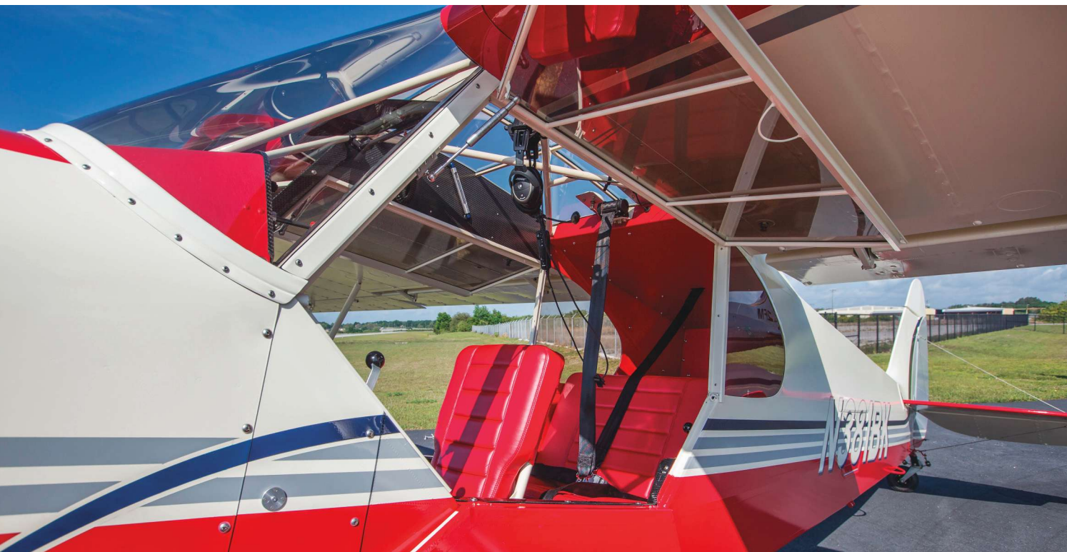
The pre-welded kit fuselage, although wildly out of line when Mark received it, is wider than a PA-18 and the left door is standard.
