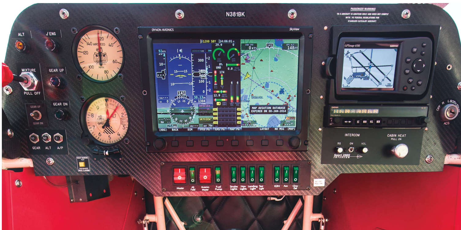
A “new age” Cub with carbon fiber panel and “glass” instruments. This is the second panel, the first was all steam gauges, but buying and flying a Cirrus convinced Mark that glass was good.
