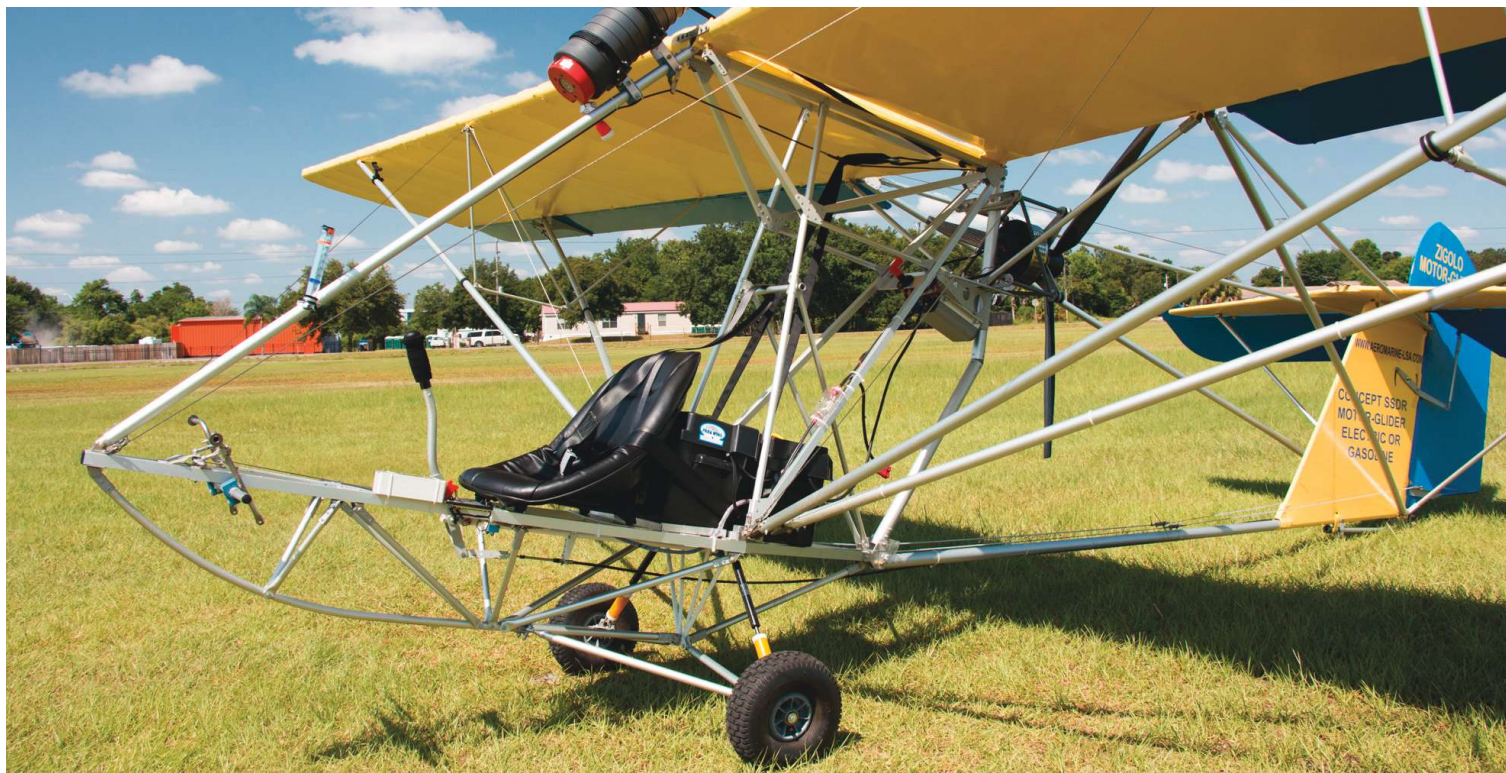
The very ultralight-looking Zigolo with its pneumatic chute.
