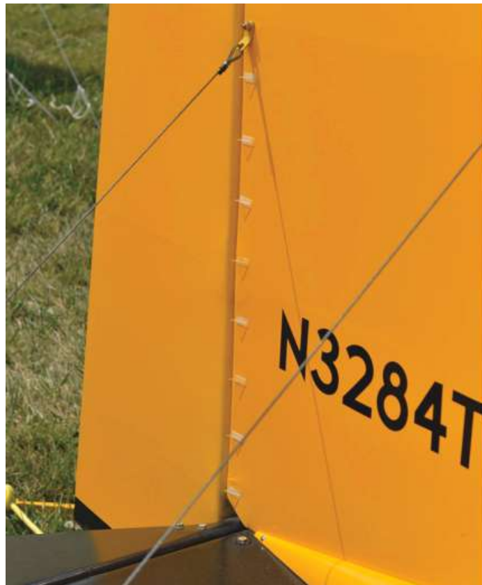
Figure 8 – Vortex generators are also used on other surfaces, such as the elevator.
