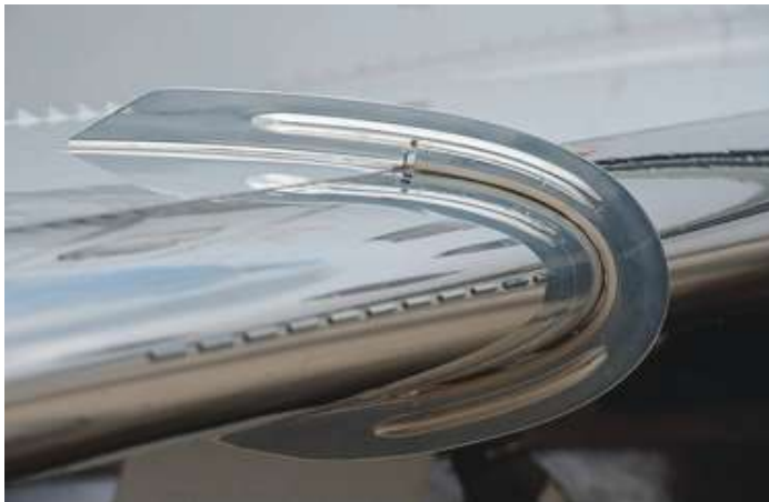
Figure 14 – A wing fence.
