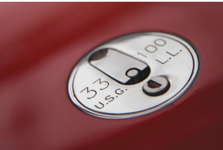
Attention to detail is evident throughout William's Legacy. To attain more speed, every effort was made to make sure everything fits flush.
