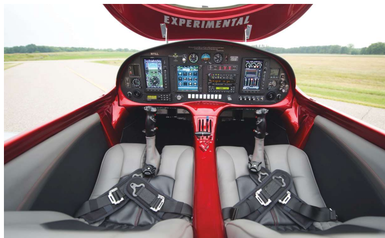
A Starflight panel surround, console, throttle quadrant, and rudder pedals are used. William is proud of the panel's symmetry and clean look.
