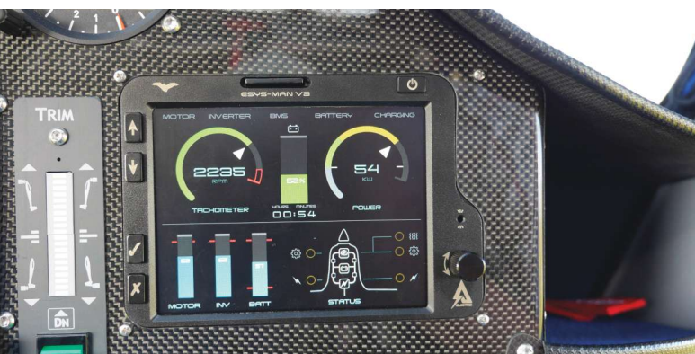
This is the power train/battery annunciator panel, running in a flight simulation mode indicating 2235 rpm and 54 percent battery capacity .
