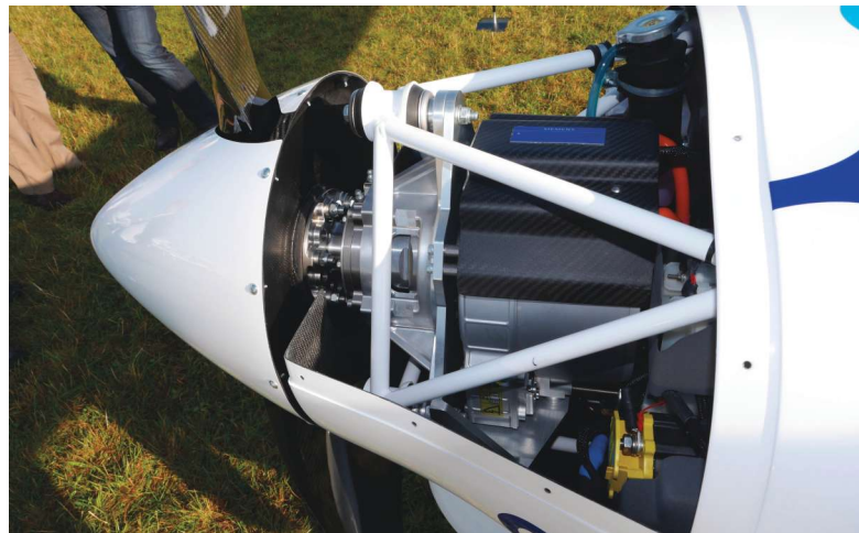
The Siemens propulsion package weighs only 31 pounds; it's all you need under the cowling.
