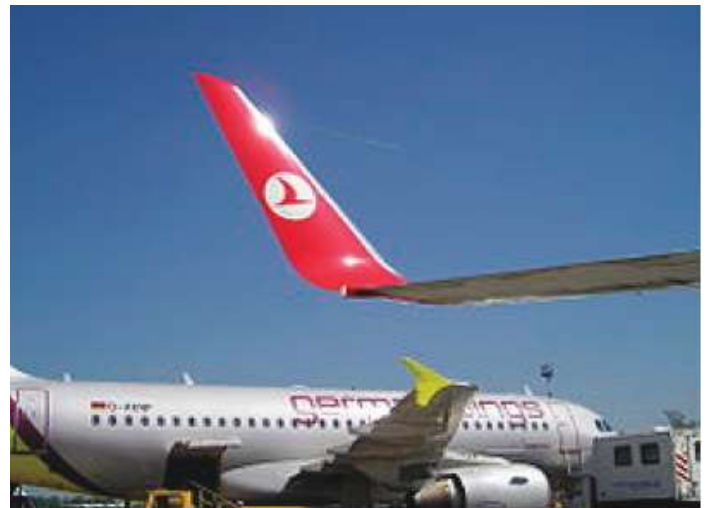
Figure 16 – A wingtip winglet.
