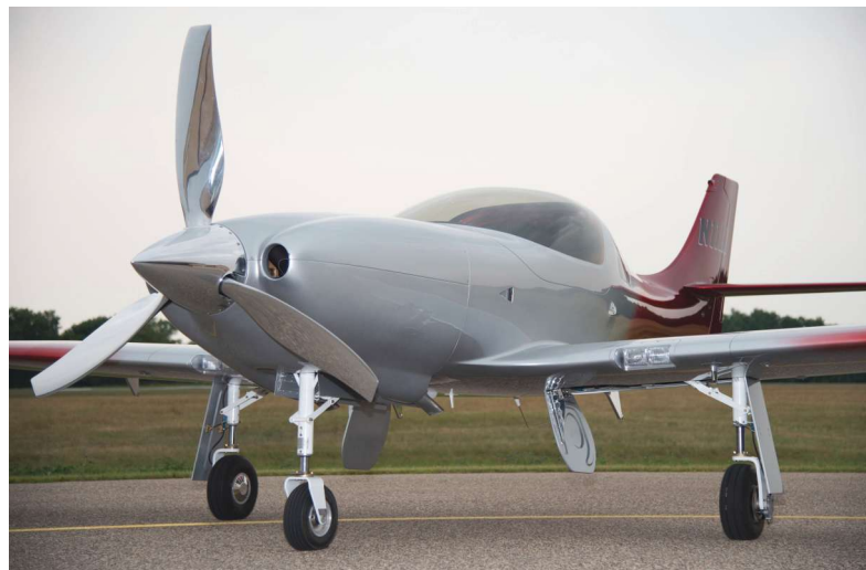
Lancair and Hartzell Propellers cooperated on development of the scimitar-style propeller.
