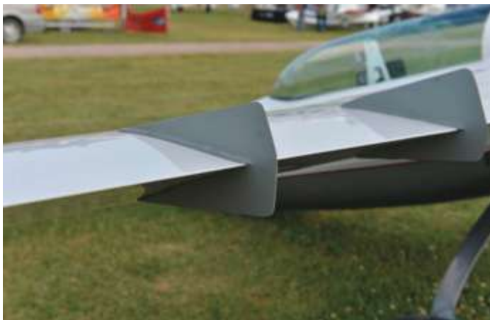
Figure 15 – A fence attached to the trailing edge of a wing.
