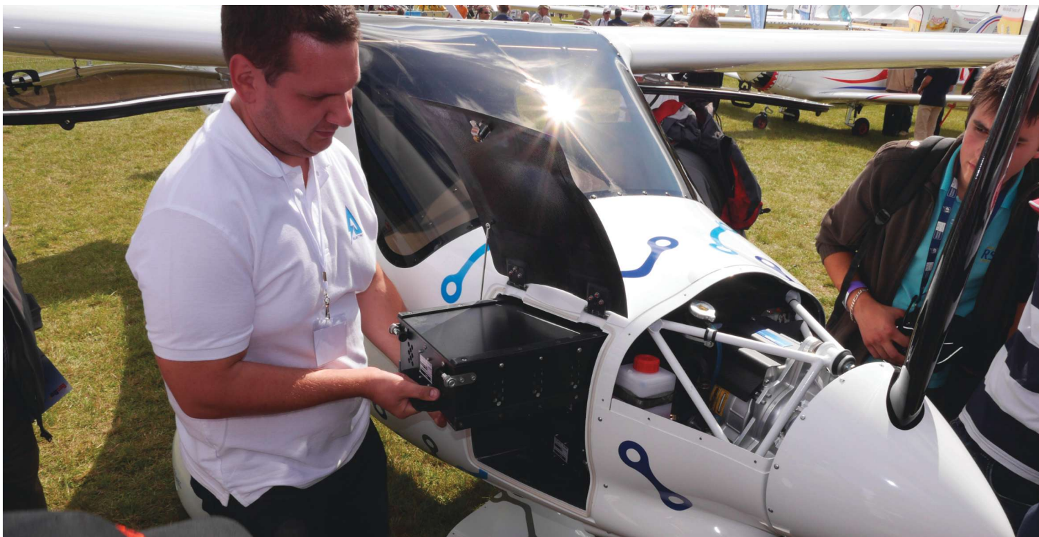
Tine Tomazic demonstrates how easy it is to remove the single battery block. He said, "If you can't do this, don't fly."
