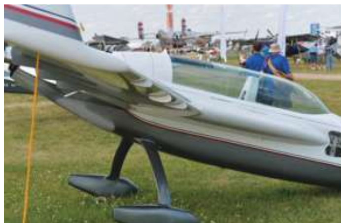
Figure 18 – Two types of vortilons.
