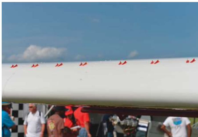
Figure 7 – Vortex generators are often placed right in front of the transition zone where the air goes from laminar to turbulent.
