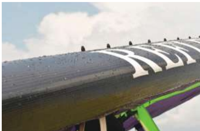
Figure 9 – Vortex generators on this trike wing have a conical top.
