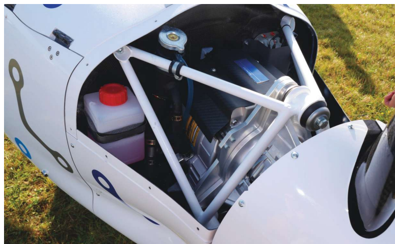
The electric motor is liquid cooled. The bottle with the red cap/liquid is the overflow bottle.
