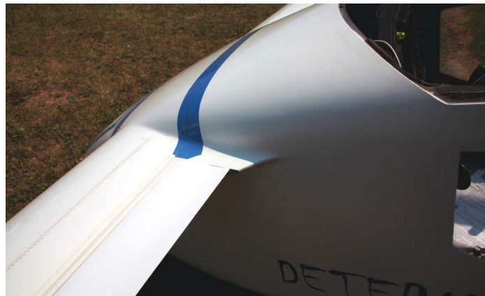
Figure 10: Klaus occasionally uses this zig-zag tape to trip the boundary layer on his wing.
