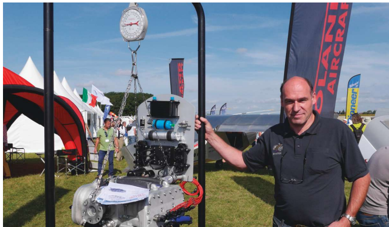
Alain Dejager showcased the six-cylinder engine, the LF39, at the French Blois Fly-In this fall. The scale was indicating 175 pounds.
