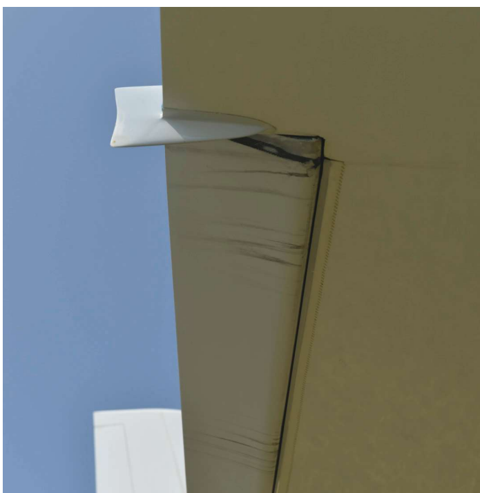
Figure 9: A trailing edge fence.
