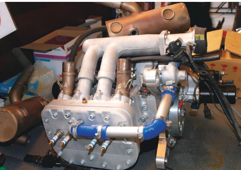
This image of the upside-down engine shows the flat cylinder head cover...
