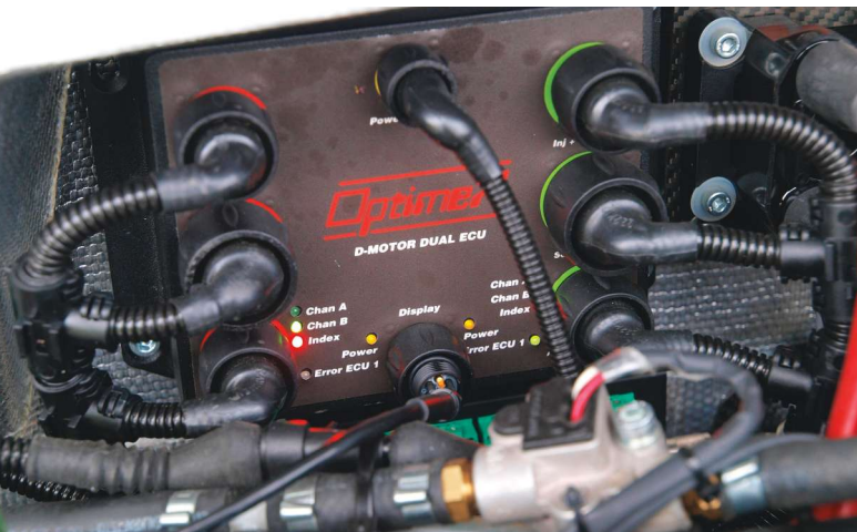
This is the all new double ECU used on the LF39 engine (standard on LF39, optional on LF26); the “B” channel is in use.
