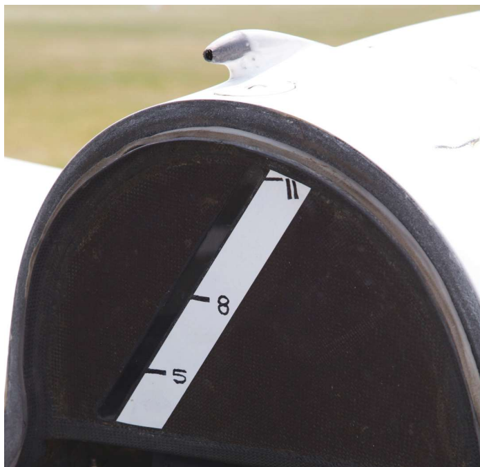
Figure 3: The header tank with a visual gauge.
