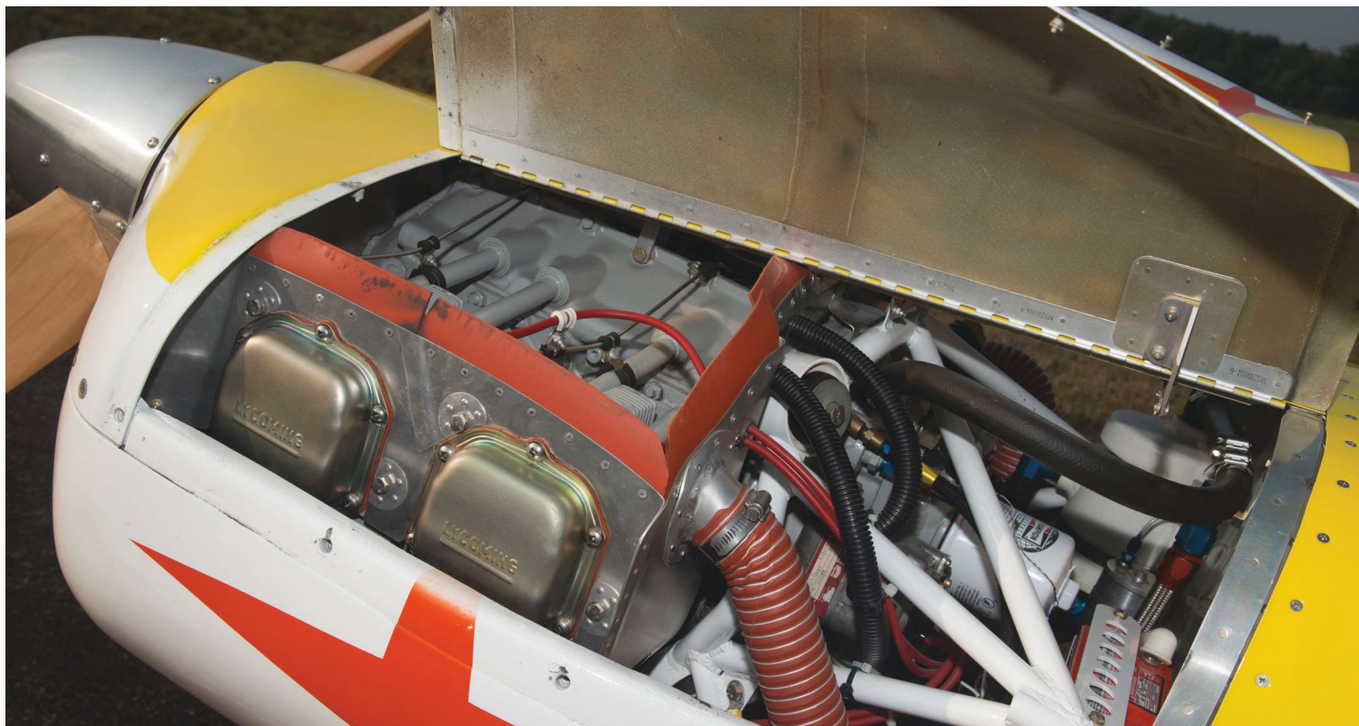
The Lycoming O-320E2D was a totally disassembled basket case that Randy found on Barnstormers.com. In the course of rebuilding the engine, Randy added a Silver Hawk fuel-injection unit and a Christen inverted oil system.
