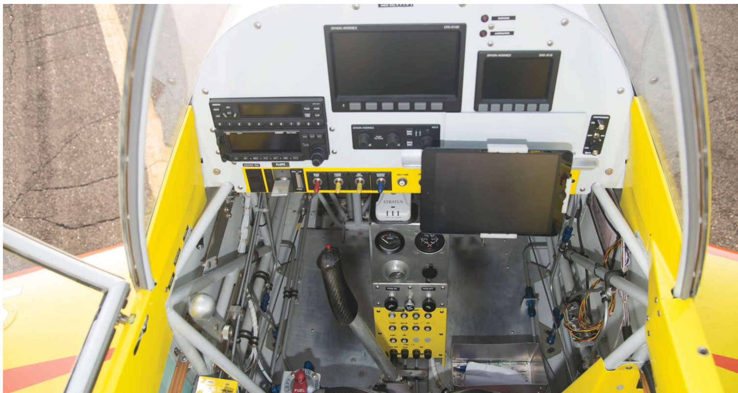
Randy's panel reflects the trend toward glass cockpits in almost any kind of airplane. And the iPad is becoming the most popular navigation add-on.
