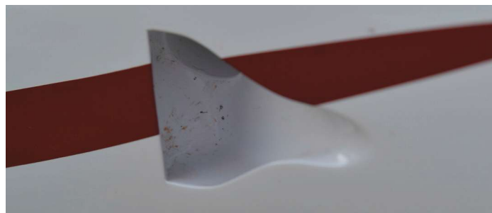
Figure 6: The bugs inside the cooling duct show that the airflow into the duct isn't smooth.
