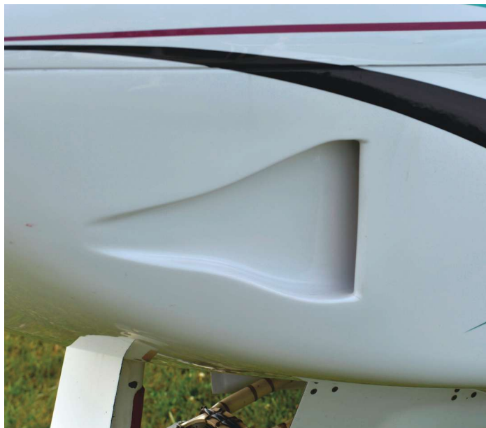
Figure 12: A standard NACA cooling air duct.
