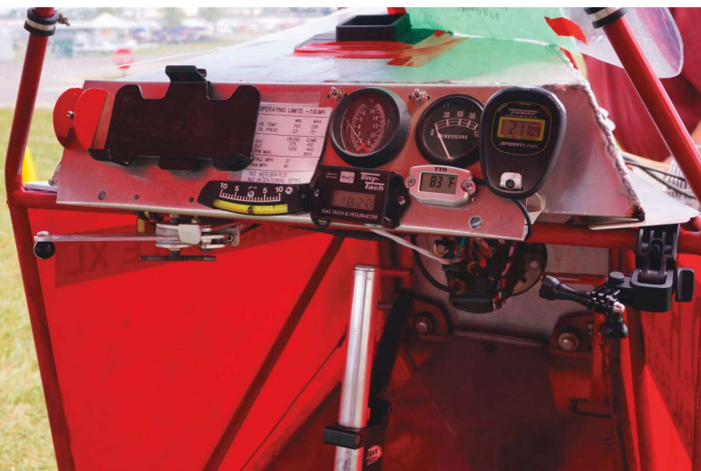
The cockpit of Les Homan's Legal Eagle XL reveals minimal instrumentation.
