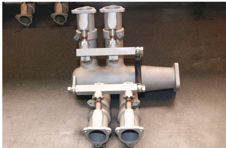
The intake manifold is located below the engine; note the two short high-pressure fuel rails and four injectors.
