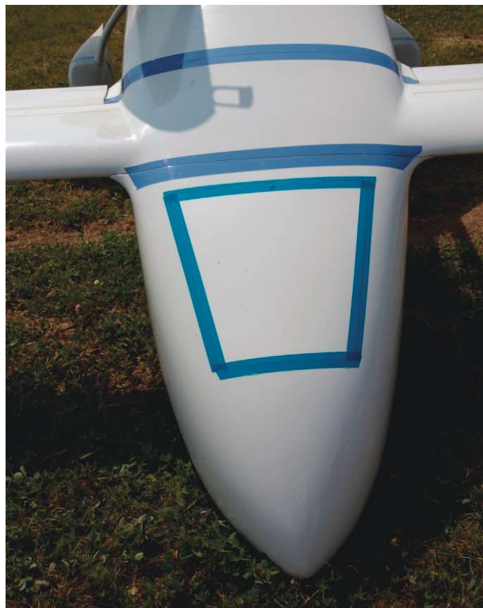
Figure 8: Klaus uses this special blue "flash breaker" tape because it doesn't leave a residue and doesn't come off in flight.
