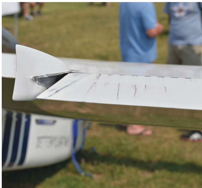
Figure 7: Aerodynamic improvements to the ailerons.
