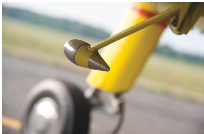
The aileron balance weights hang out into the wind.
