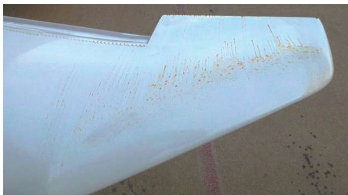
Figure 5: Using oil visualization to determine airflow.
