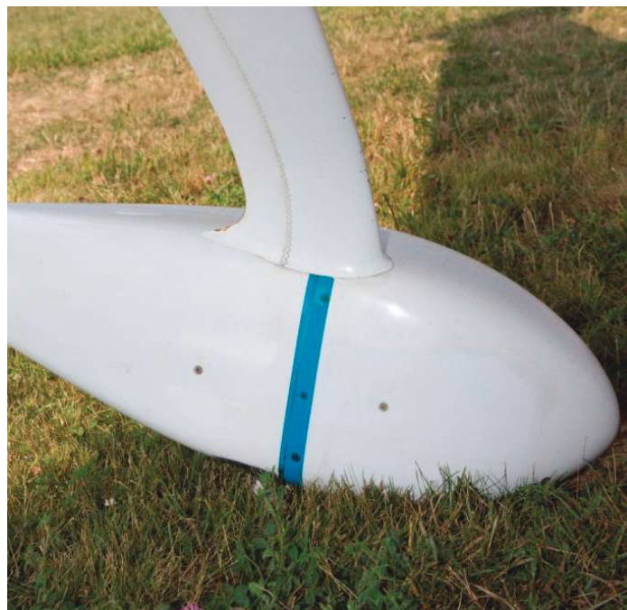
Figure 11: More zig-zag tape on the wheelpant trips the boundary layer there as well.
