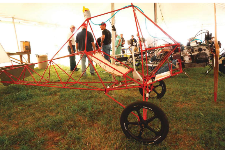
A Legal Eagle welded tube fuselage in the Ultralight Workshop tent at AirVenture.
