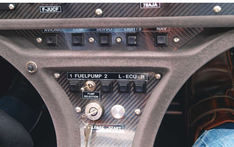
When the two-channel ECU is installed, the engine panel will look like this; note the two (left and right) ECU channel selector buttons.
