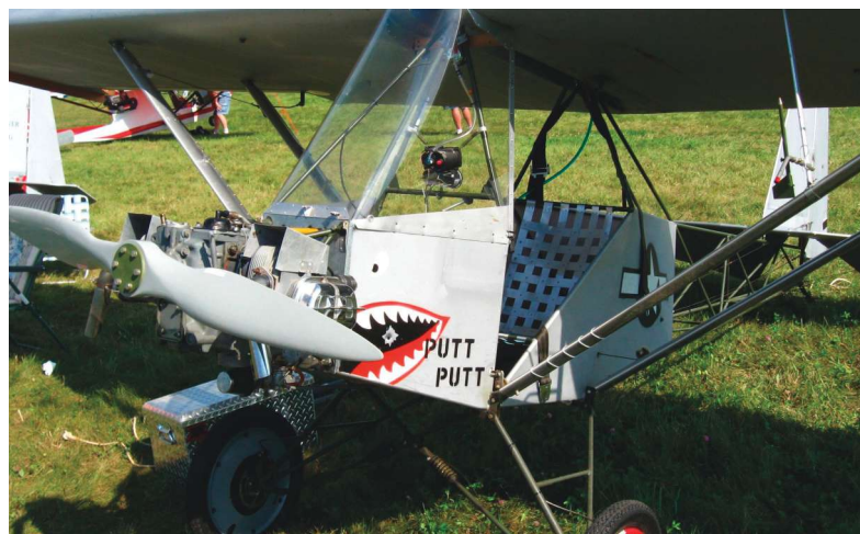
Joe Spencer's PuttPutt showing the unique, one-pound seat made of woven metal strips.
