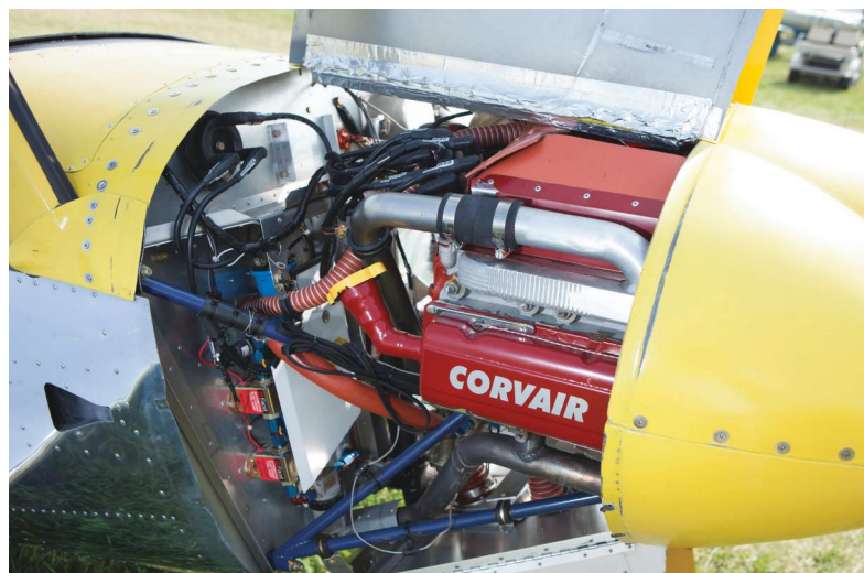
Pat also built the Corvair engine that powers his Zenith. He used William Wynne's conversion plans. He's building another Corvair engine for the Tailwind he is building now.
