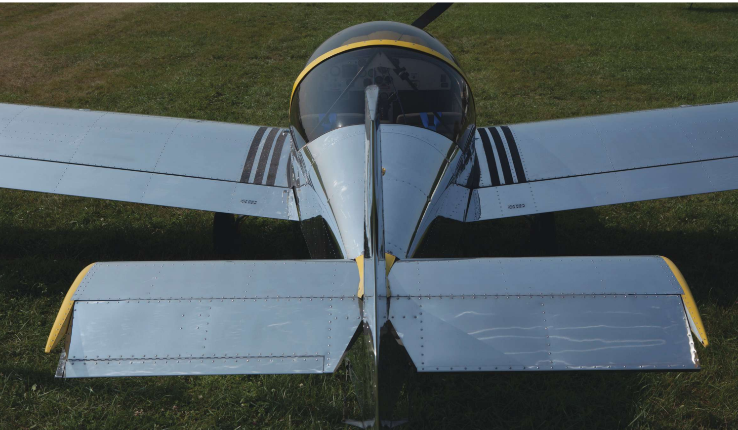
Pat's 601 weighs in at 840 pounds, 40 pounds more than factory's Lycoming O-235-powered model. Pat's custom BRS parachute system and custom canopy account for the majority of those pounds.
