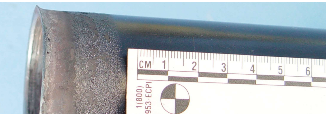
Figure 2—The aft fracture surface of the failed forward weld on the left side propeller shaft tube, as received.
