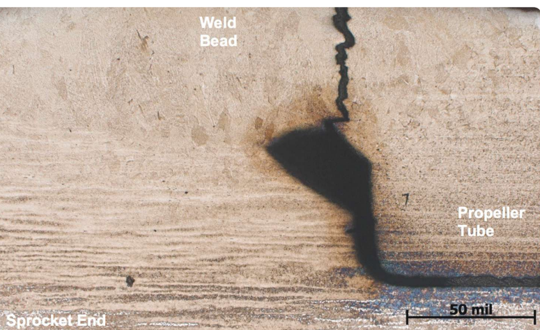
Figure 14—Cross-section of a cracked section the right side propeller shaft aft weld, showing a crack emanating from a gap that had not been welded (~25X, etched with 4% Nital).
