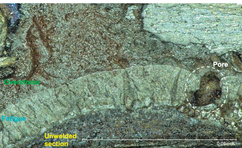
Figure 8—Closer view of a typical area of the right side propeller shaft forward weld fracture surface, after cleaning. An area of fatigue could be observed between the unwelded inner area and the rest of the fracture surface.
