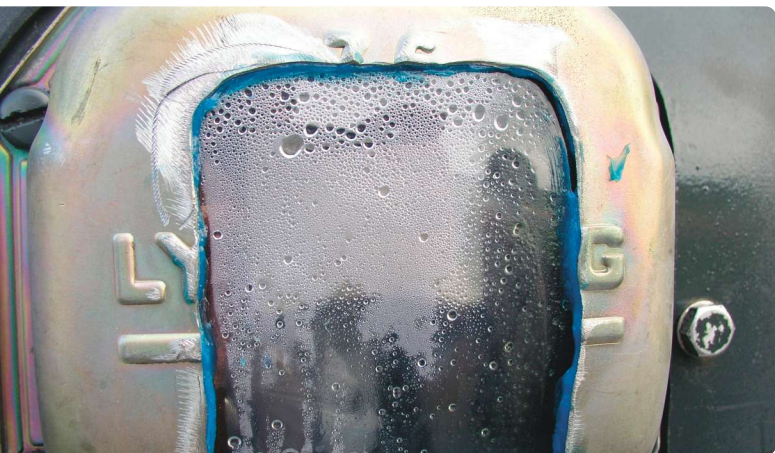
Penn Yan put a window in a valve cover, to show how much moisture can accumulate, just from condensation. Frequent use (flying) is the only remedy, though frequent oil changes definitely helps!
