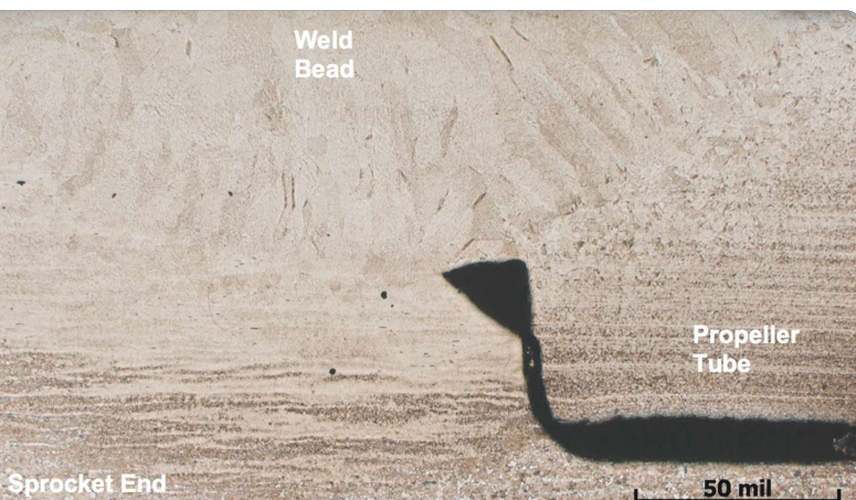
Figure 13—Cross-section of an intact section the right side propeller shaft aft weld, showing the depth of the weld penetration relative to the joint (~25X, etched with 4% Nital).
