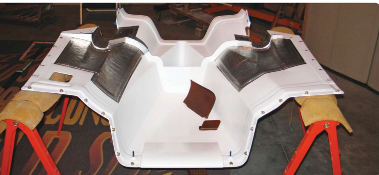
The inside view of lower cowl showing thin forward and aft stiffeners, a one-inch thick airfoil on the lower inlet lip, heat shields, and cooling air deflectors to promote even cylinder cooling. The heat shields consist of one layer of fiberfrax insulation bonded to the cowl with high temperature RTV, covered by a layer of heat reflective material that is used in firefighter's suits. The combination works very well.
