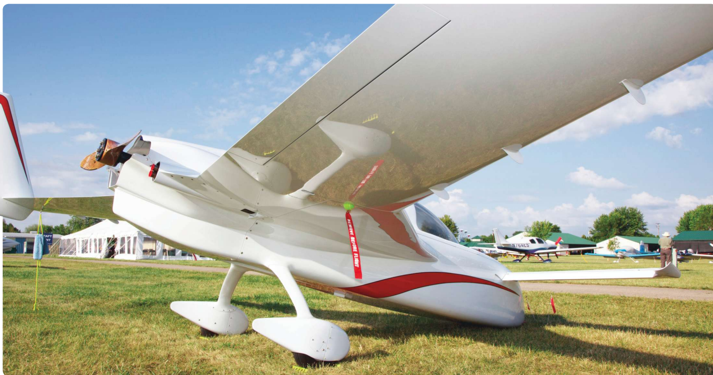
The highly reflective finish of Dennis' Cozy IIIP resulted from two coats of clear top-coat, with half of the final coat sanded away with 1500, then 2000 grit wet sandpaper. This was followed by buffing with two successively finer grades of buffing compound.
