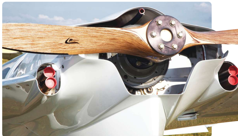
The aft end of lower boat-tail cowl was extended as far back as possible to minimize curvature and reduce airflow separation. Aft end of upper cowl was cut as far forward as possible to allow relatively unimpeded engine cooling air to exit.
