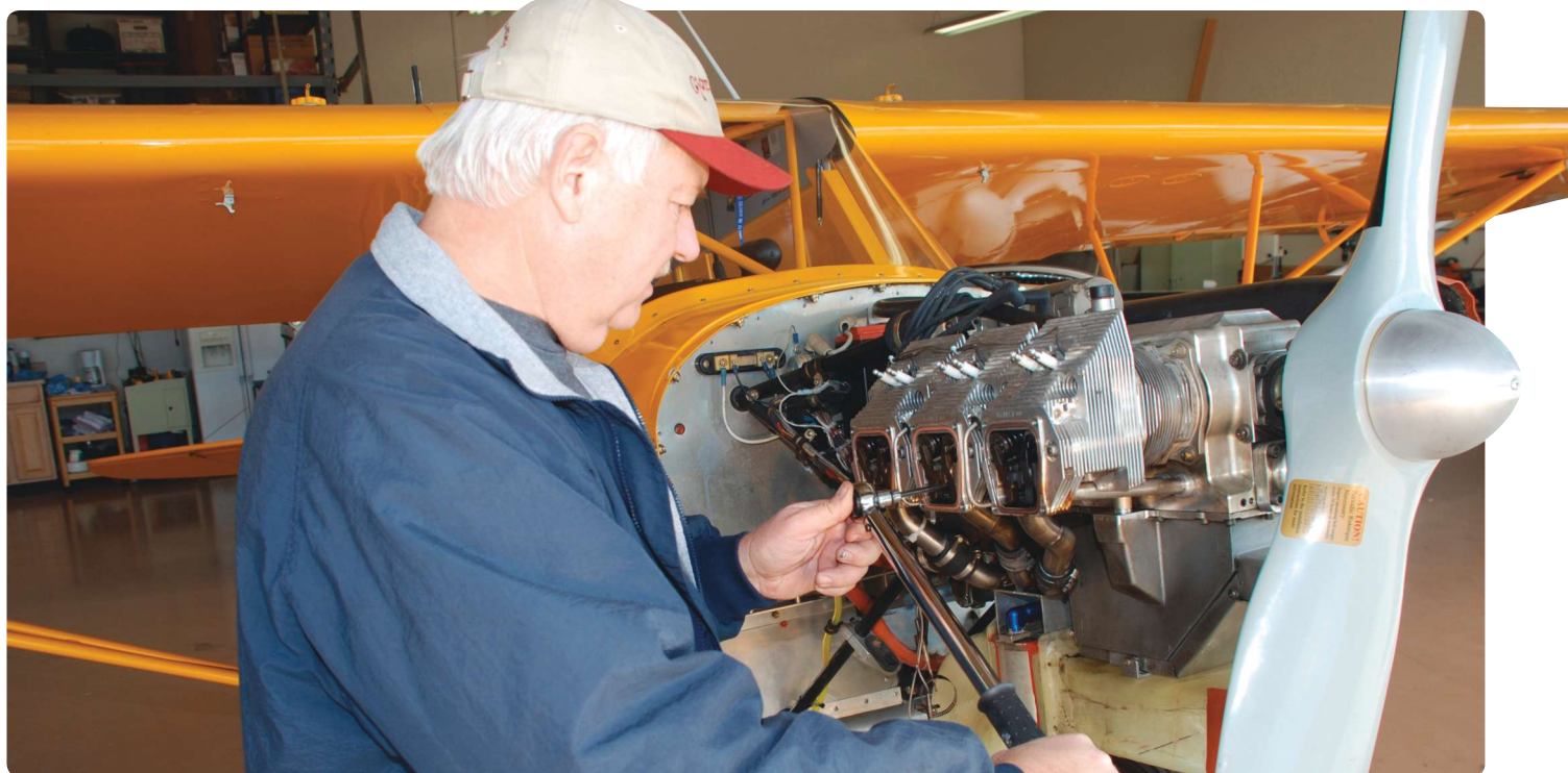
Your author torques the head bolts on his Jabiru 3300A engine during an annual inspection. This engine saves about 30 pounds compared to a Continental O-200, but it was more difficult to get running well and requires more maintenance.
