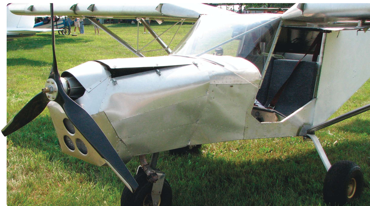
Although not the final version, one would hope that your cowl would be a better match for the airframe and powerplant than this one is.
