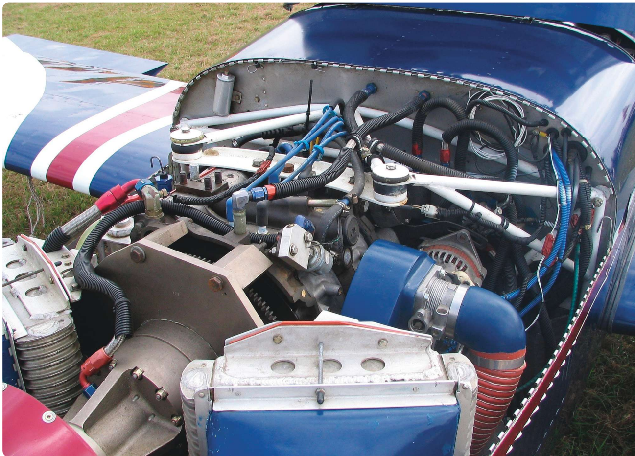
Ed Anderson went against the status quo when installing his 13B Mazda Wankel rotary engine in an RV-6A with the “spark plugs up.” PSRU is by Real World Solutions.
