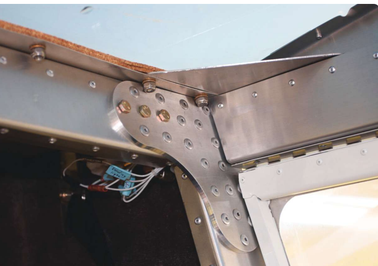
The CruZer uses aircraft-grade pulled rivets throughout.
