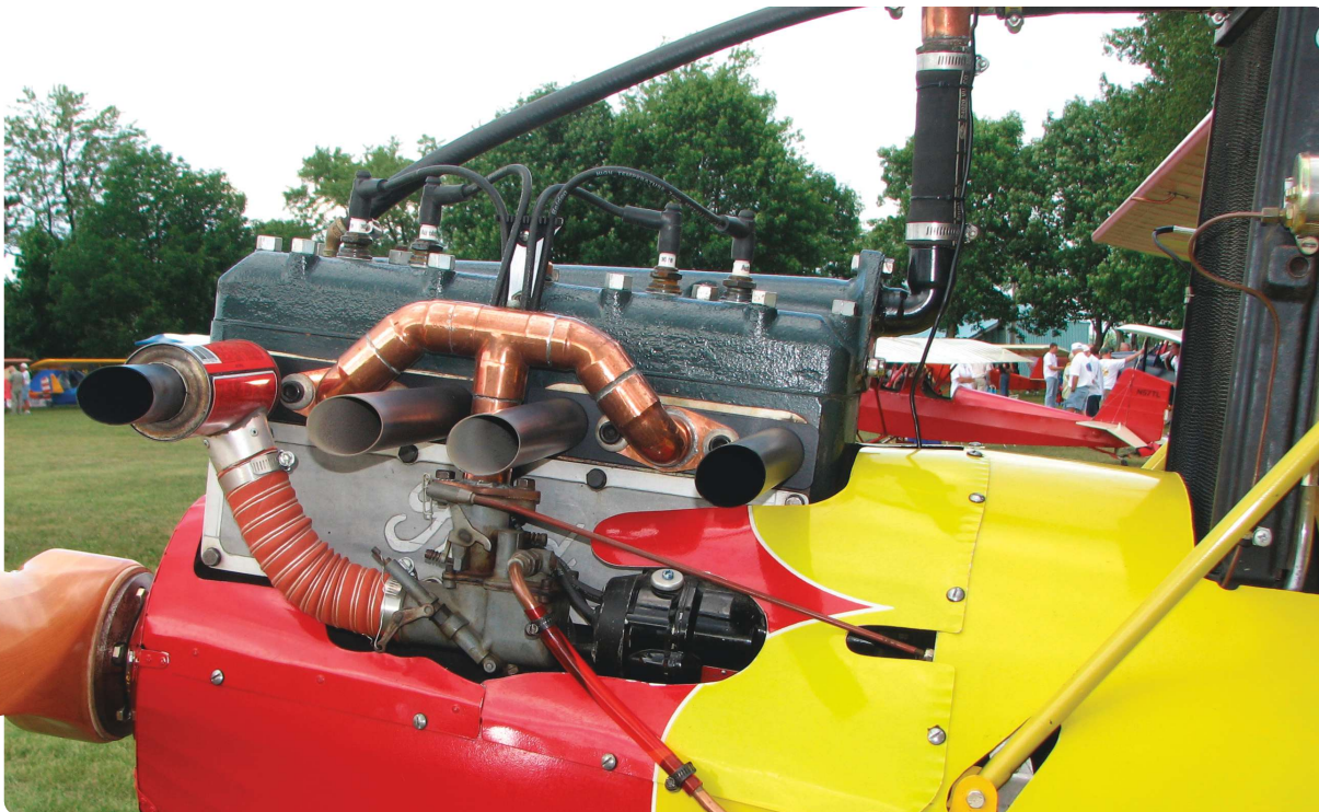
Many auto conversions, like this antique Ford engine, are not supported by a manufacturer and are, for the most part, one-off creations by the builder.
