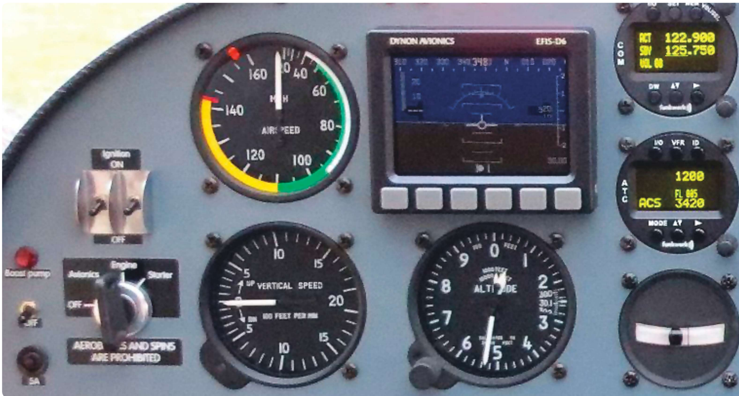
Aerotrek instrument panel with Funkwerk radio and transponder in upper right corner of photo.
