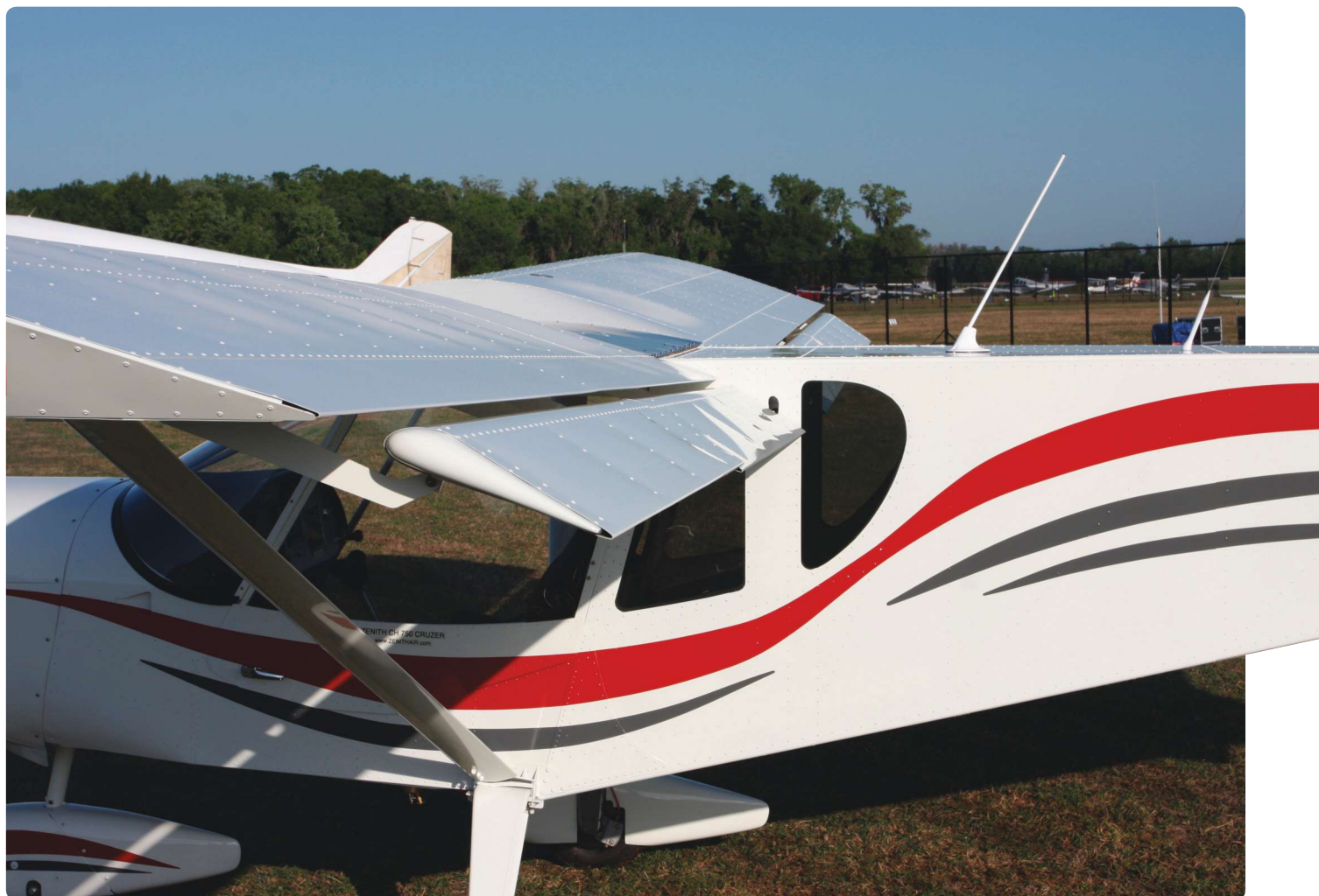
The ailerons droop with the flaps for more lift with less drag.
