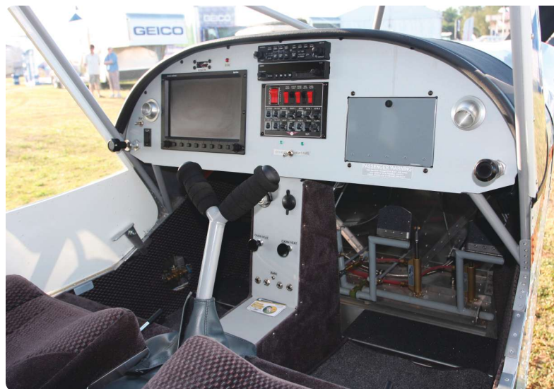
The much wider-than-normal cockpit has a “Y” control stick so both seats have control with minimal obstruction.
