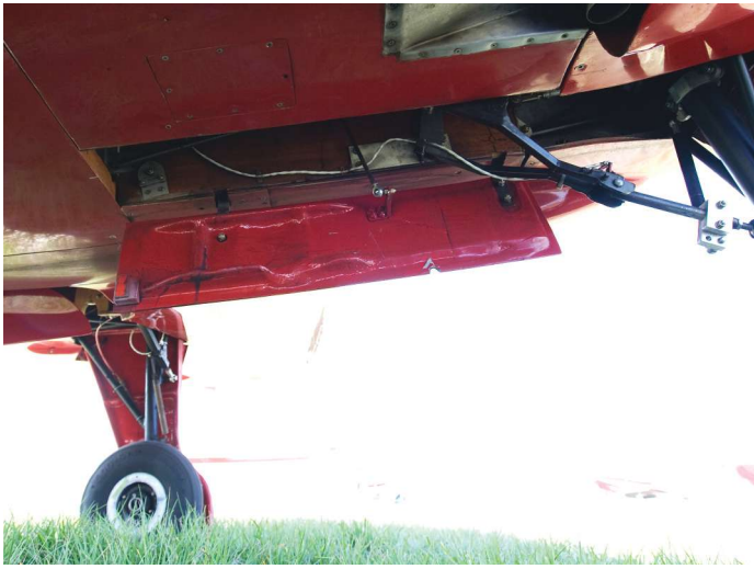
Wanting to get all three gear doors closed as tightly as possible, Mike designed a separate system that uses a small hydraulic cylinder that is sequenced to close the doors after the gear is up.
