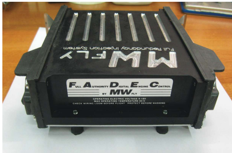
The new single-engine controller casing hosts two separate engine controller units.
