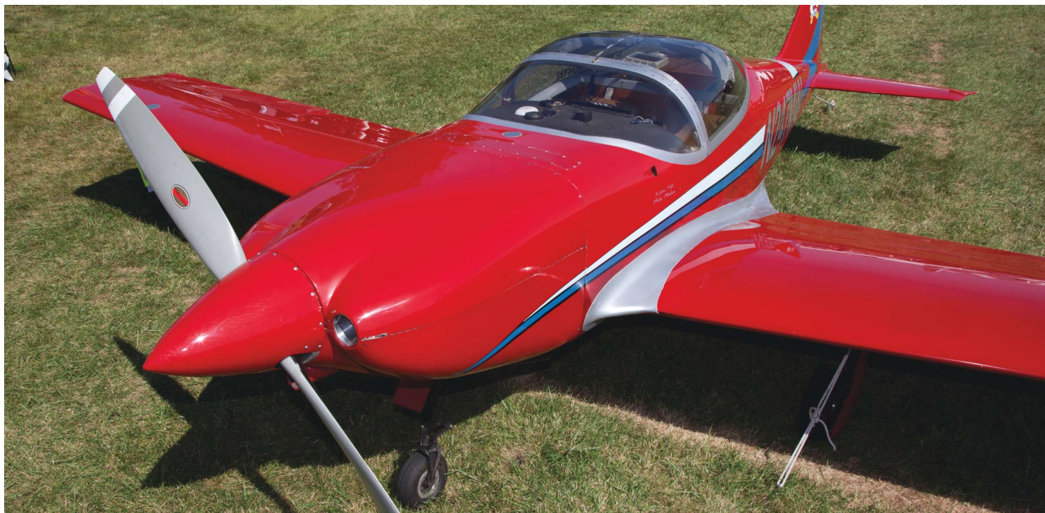
Mike modified the fuselage sides subtly using thin layers of foam to give the airplane's sides a more rounded appearance.
