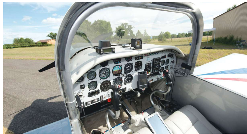
Instrumentation in Bob’s Mustang II includes a three-axis electric trim, a Navaid AP-1 wing leveler/tracker autopilot, a Garmin SL 40 Comm, a TerraTXT 760D Comm, a TN 200D Nav, and a TRT 250 D transponder.
