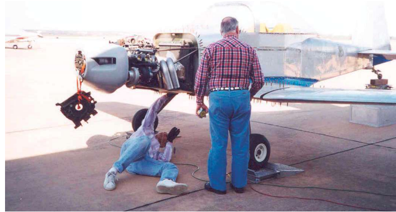
Bob measures to determine the engine mount spacing needed to keep the aircraft within the Mustang's weight-and-balance envelope.
