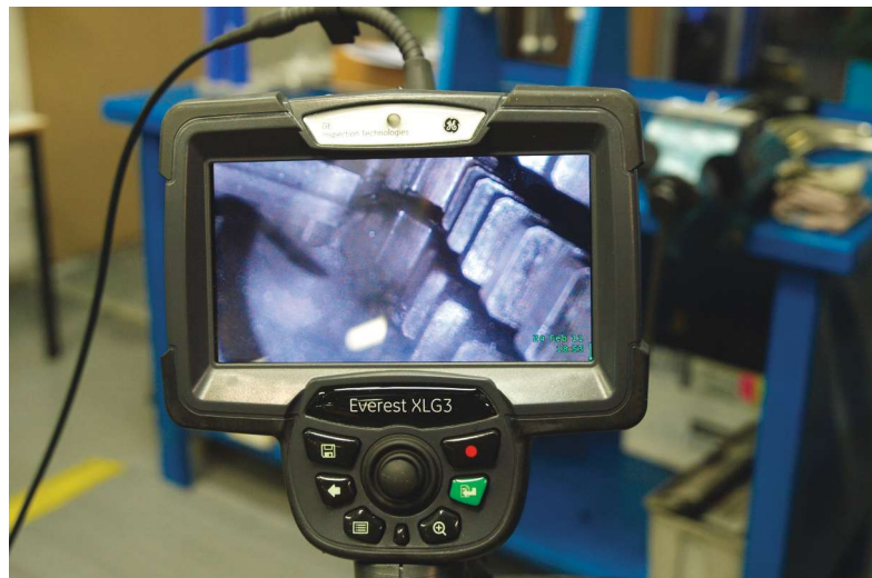
Probably the most unique feature of MW Fly engines is the numerous openings on the engine casing allowing the entire engine to be inspected with a borescope.
