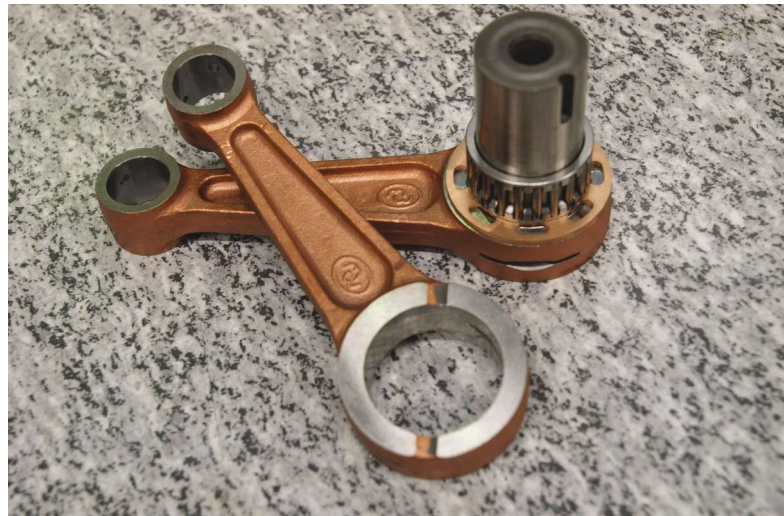
Two of the four monolithic (one-piece) connecting rods on the MW Fly engines.
