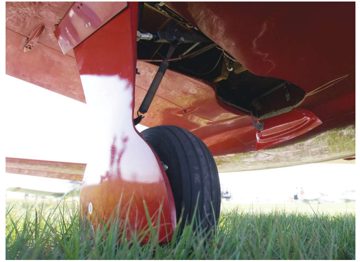
Wanting to get all three gear doors closed as tightly as possible, Mike designed a separate system that uses a small hydraulic cylinder that is sequenced to close the doors after the gear is up.
