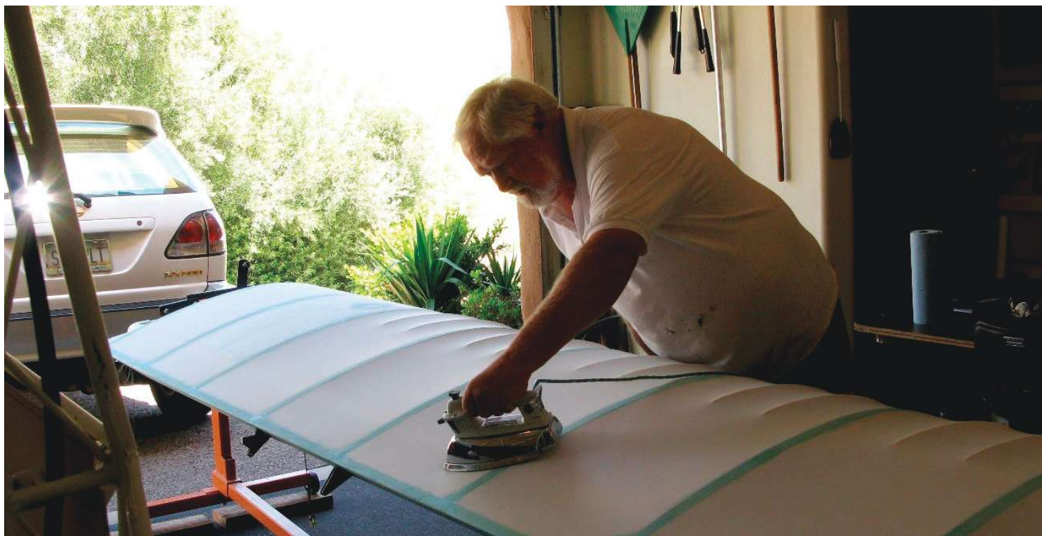
Dennis shrinking the fabric tight on the right wing.
